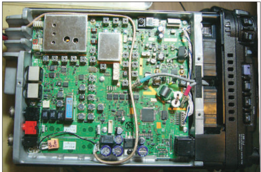
Figure 5 — This prototype was installed by VA7MP into a diecast aluminum enclosure for use in a Yaesu FT-857/897 series transceiver.
