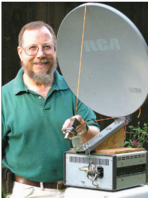
Figure 3 — A piece of string is all that is needed to position a feedhorn at the focal point of an offset-fed dish.
