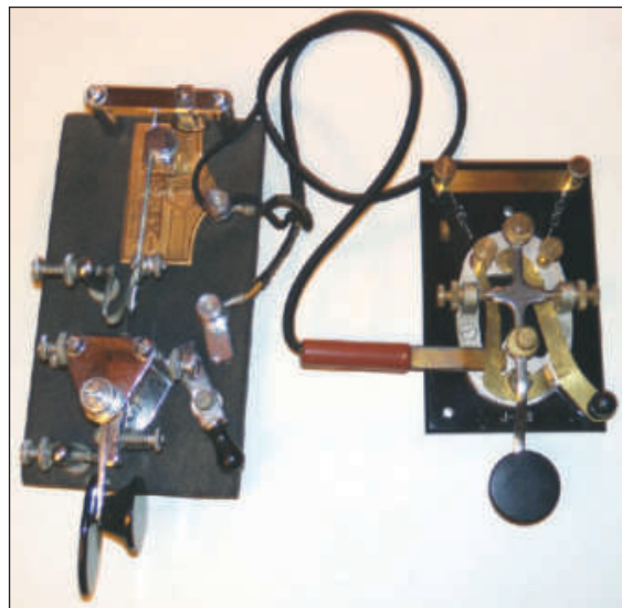
Figure 2 — A circa 1956 Vibroplex Lightning Bug attached to a WWII vintage J-38 straight key using the cord and wedge. Note that the rope made from the cotton covering is used to provide strain relief under the bug terminal.
