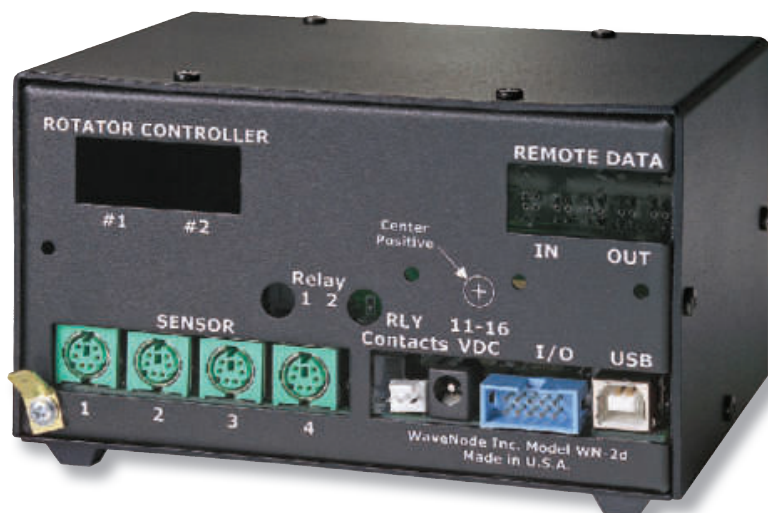
Figure 2 — Rear panel of the WaveNode WN-2d stand-alone unit. Up to four power sensors can be plugged in at once, along with auxiliary inputs and logic outputs.
