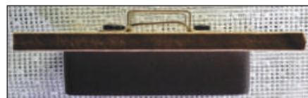
Figure 5 — This is a side view of the microphone holder showing the microphone clip on top, next the particleboard and finally the pine brace shaped to fit the cup holder. [Tom Hart, AD1B, photo]
