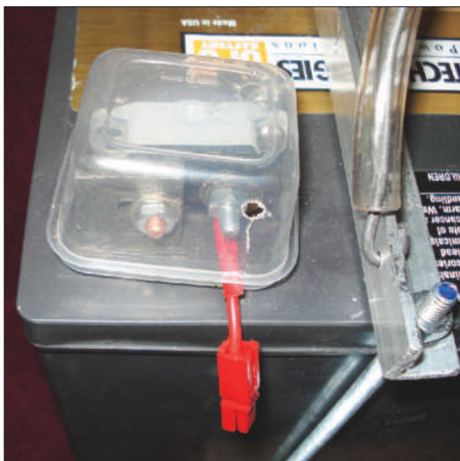
Figure 3 — Here you can see the plastic container rotated into position to cover the battery terminal, protecting it from an accidental short circuit.
