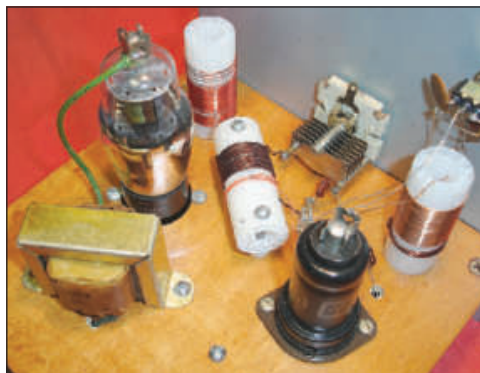
Figure 3 — The author's two-tube regenerative receiver using three paper roll coil forms. [Bill Higgs, NT4C, photo]
