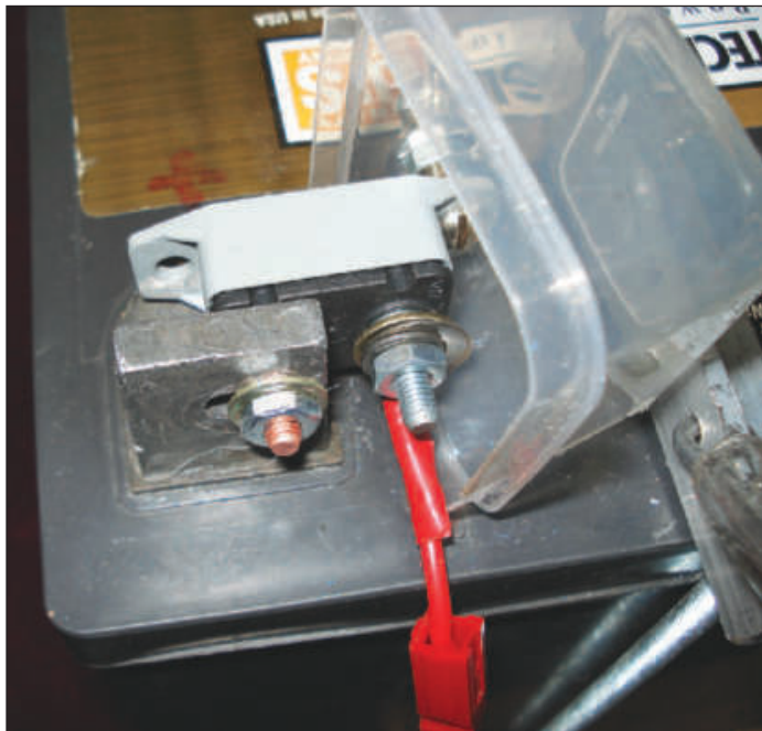
Figure 2 — An automotive-style circuit breaker can be mounted directly to the positive battery terminal, eliminating the need for a fuse at the connection point. A plastic container bolted to the breaker provides a convenient way to protect the terminal, breaker and wiring from a tool or metal object falling against the terminal and causing a short circuit.
