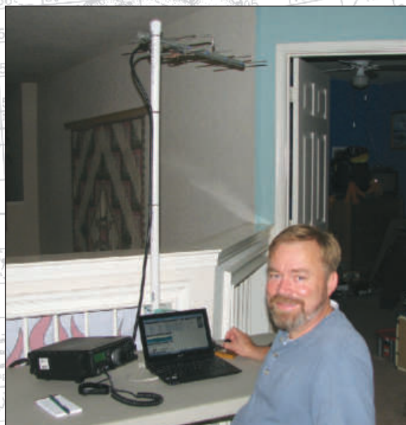
Steve Yates, AA5TB, set up a station in his Fort Worth, Texas game room for the 2011 August UHF Contest, and was able to work stations 230 miles away with a tiny 6 el Yagi. Where there's a will (and a touch of RF), there's a way! [photo courtesy Steve Yates, AA5TB]
