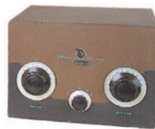
Figure 4 — A 1950s vintage E. F. Johnson "Matchbox" antenna tuner designed to work with vacuum tube transmitters of its day. This capable tuner could match balanced or unbalanced loads on the ham bands of its day.
