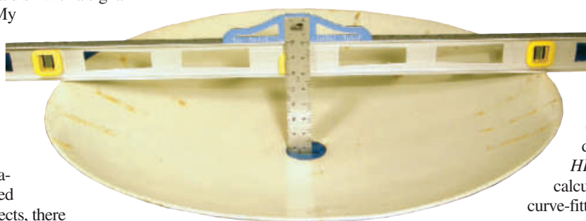
Figure 2 — The depth of a parabolic dish is easily measured using a straightedge and a T-square.
