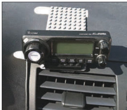
Figure 2 — Here the completed mounting holds the control head where it doesn't interfere with driving but is accessible for easy operating. [Mike Fesko, KB1LKH, photo]
