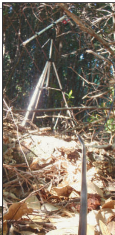
The Elk log periodic antenna in the heavily wooded "clearing." This was the best place available to reach the easterly satellites.
