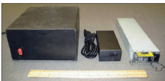
Figure 1 — Modern switching power supplies are smaller, lighter and more efficient. The linear 9 A supply on left weighs 10 times more and takes 16 times more volume per ampere than the 8 A laptop and 18 A switching supplies shown.
