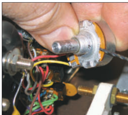
Figure 5 — To cure a stuck potentiometer drill a small hole at the base of its mounting threads and apply a small amount of light oil or WD-40. [Charlie Liberto, W4MEC, photo]
