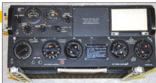
A pristine AN/ART-13 (actually the Navy version called an ATC).
