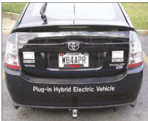
Figure 3 — The outlet on the rear of my Prius (on right) provides about 1 kW at 115 V ac from a 12 V inverter.
