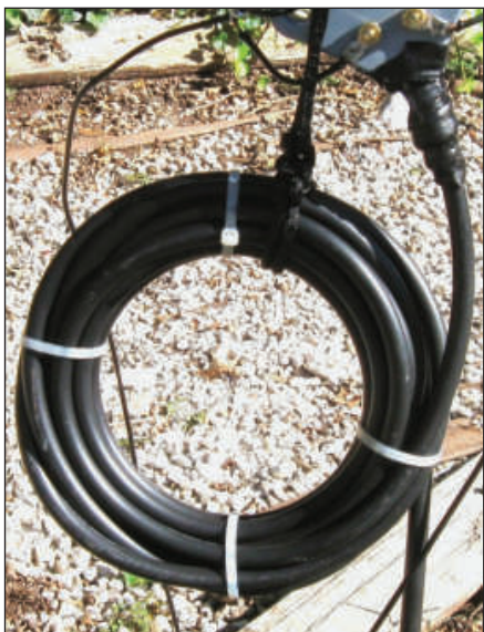
Figure 5 — The coil choke balun keeps common mode currents off the outside of the coax.
