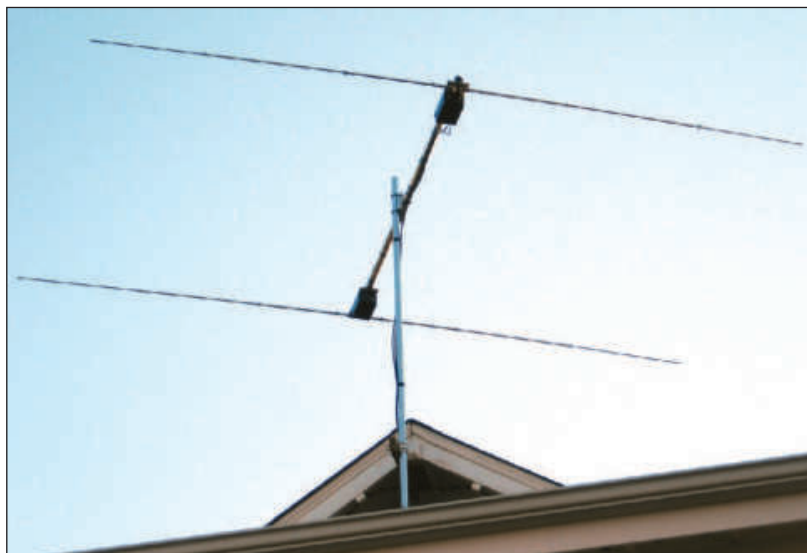
Figure 6 — The completed Q-52 installed on a rooftop mast about 30 feet above the ground. The antenna mounts easily on a 1\frac{1}{2} inch mast and can be turned with a light duty rotator such as an AR-40.
