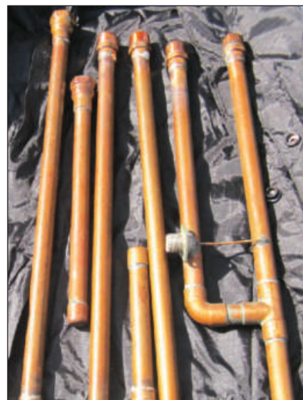
Figure 1 — The 1/2 inch copper dual band J-pole antenna cut into 15 inch segments with 1/2 inch copper threaded fittings to screw together for reassembly. Notice that the antenna parts are wrapped in a ripstop nylon rain poncho.
