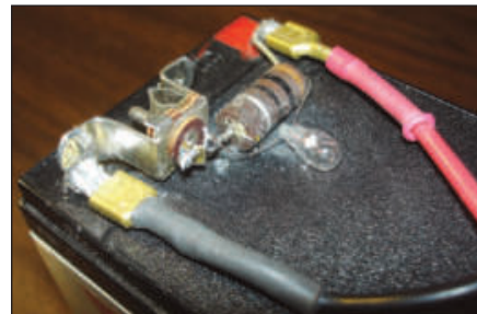
Figure 5 — This simple arrangement combined with an unfiltered wall wart works well as a trickle charger for SLA batteries. [David Gauger, W9CJS, photo]
