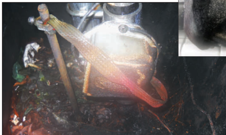
Here are the remains of the planter. You can see the charred ground braid, unun and antenna base surrounded by the remains of the plastic flowers. Note how close the braid was to the hot side of the unun. [Tom Schaefer, NY4I, photo]
