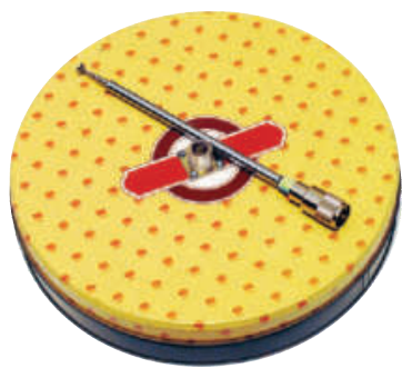
Figure 4 — Mount an SO-239 connector to the top of a cookie tin, add the quickie antenna and you're on the air. [John Portune, W6NBC, photo]
