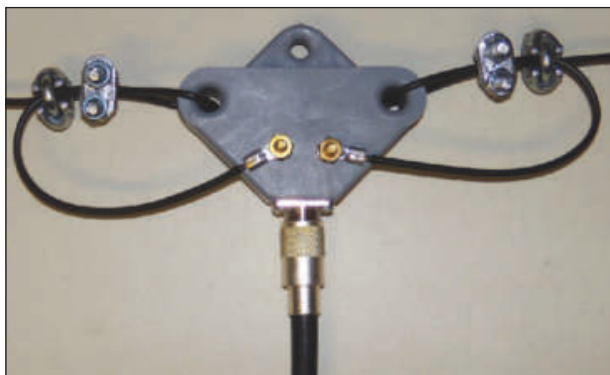
Figure 4 — Center insulator connection and mechanical detail. The wire is secured using wire rope clamps — tightened just to be solid — not so tight that the insulation or wire is deformed. Terminals are crimped and soldered and secured with stainless lock washers to ensure contact. After it's all finalized the coax connector is socked down and taped and all connections and the clamps are sprayed with clear lacquer.
