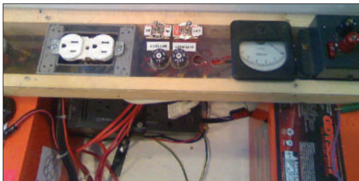
Figure 9 — Panel with fusing, meter, Powerpole strip and switches. See text regarding circuit breakers.
