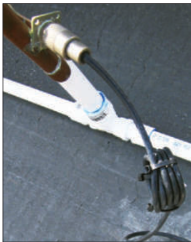
Figure 2 — The feed point choke prevents current from coming back to the radio via the outside of the coax. It is five turns of the RG-58 transmission line held together with zip ties.
