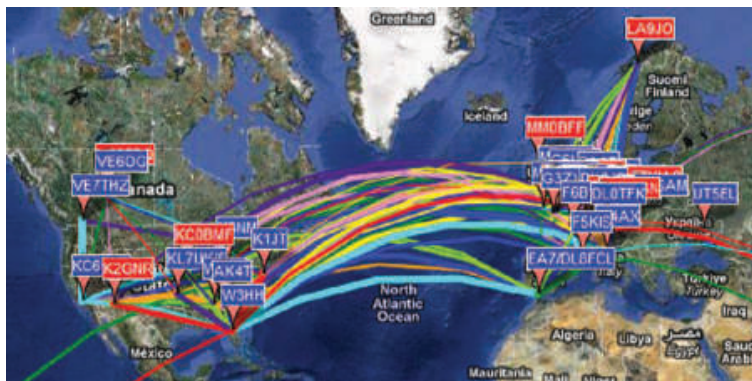
A WSPRnet map of 1 hour's activity. By focusing in on the US a sudden burst of activity can alert you to a dead band springing to life. [courtesy Joe Taylor, K1JT, and Bruce Walker, W1BW]
