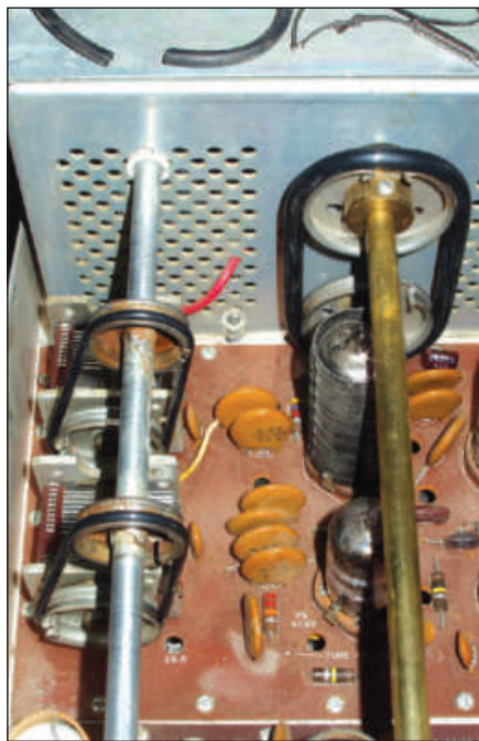
Figure 3 — The photo shows how inexpensive O-rings can be used as an alternative to the more expensive drive belts when restoring Heathkit transceivers.
