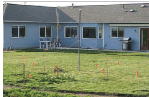
Figure 16 — Completed four element shared apex loop array utilizing two orthogonally positioned arrays identical to those described in this article.
