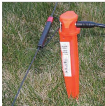
Figure 10 — Coupler stake and coupling link with phasing dot toward anchor.
