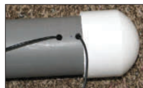
Figure 7 — Top mast section showing guide holes and loop wire routing.
