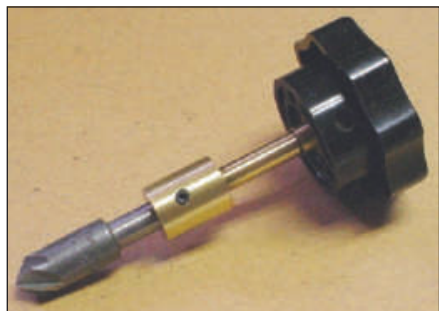
Figure 5 — A countersink, shaft extension and handle make deburring jobs easier and more professional. [John Franke, WA4WDL, photo]
