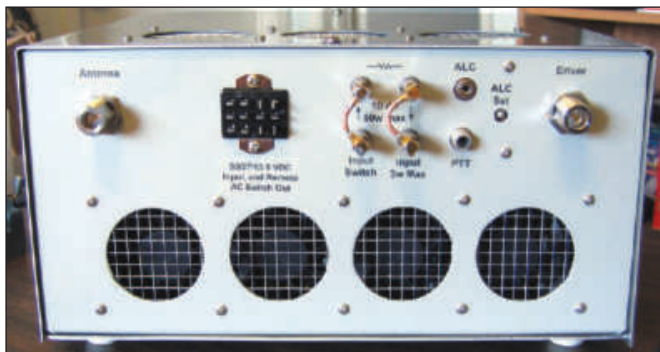
Figure 6 — View of the rear panel showing the connectors provided for moving the 10 dB attenuator in or out of the input path. There is also a screwdriver adjustment for setting the ALC level.
