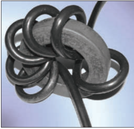
Figure 2 — Common mode choke made by winding the antenna feed coax through a ferrite toroid. The coax can be neatly secured with nylon tie wraps. The choking inductance is proportional to the square of the number of turns.
