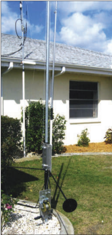
Figure 6 — The fully nested antenna is approximately 13 feet in height.
