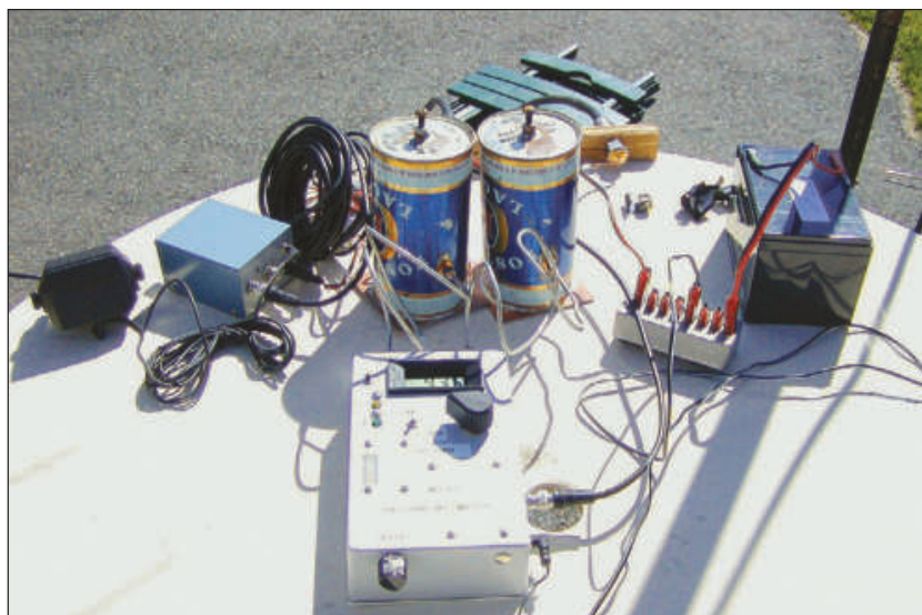
Figure 4 — Here is an actual antenna ratiometry test setup using homebrew ratiometer, filters and tonemeter.
