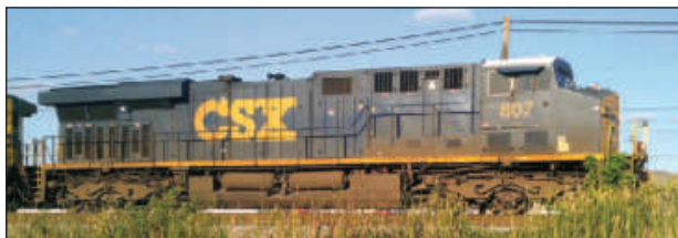
This 807 is a GE model ES44AH ready to pull a train south out of Osborn Yard (CSX Transportation) on the south side of Louisville, Kentucky. [John Morton, WA4UMR, photo]
