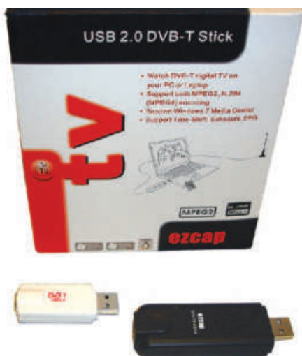
Figure 1 — DVB-T dongles are all you need for a V/UHF SDR. They come in various shapes and sizes.
