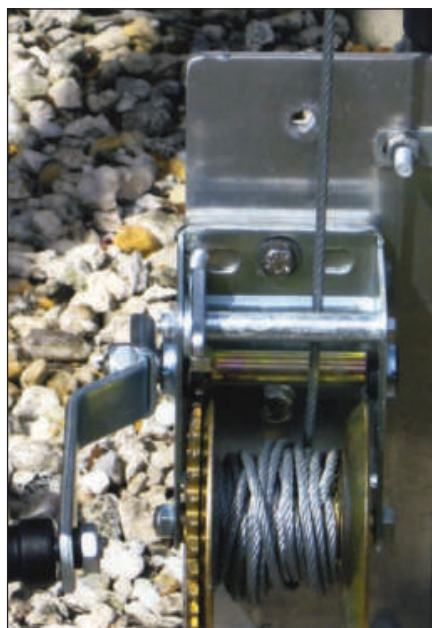
Figure 4 — The winch used to raise and lower the antenna. It can work in either position, but performs better if raised.
