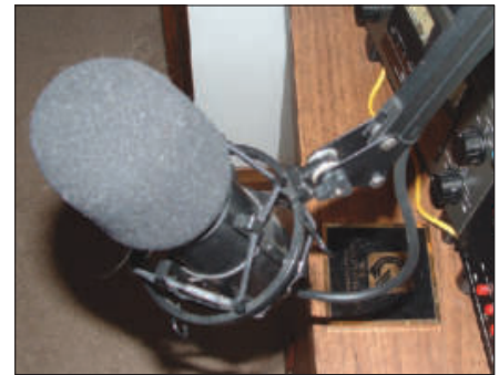
Figure 5 — A couple of washers will compensate for the difference in size between the lamp assembly and the microphone holder. [Joe Vlk, W8DCQ, photo]
