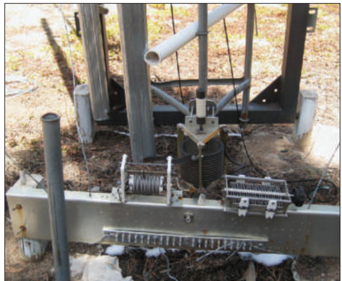
Figure 2 — The base of the 90 foot, tilt-over, linear loaded vertical with matching L/C tuner. This antenna has a ground screen made of 500 feet of barbed wire buried six inches below the ground for lightning protection, plus quarter-wave radials four inches above ground.
