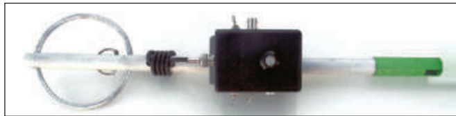
Figure 1 — Left to right, loop, coupling loop, balun, attenuator and handheld transceiver mount (behind attenuator).
