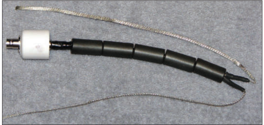
Figure 3 — A common mode choke can be made from multiple ferrite beads. This is a better solution for foam dielectric coax, such as RG-8X. The choking inductance is proportional to the number of beads. [Photo courtesy Lou Burke, W7JL]
