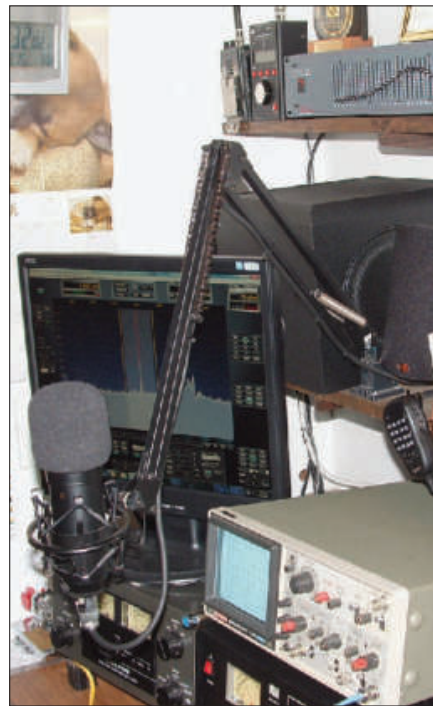
Figure 4 — For a few bucks and a little time an inexpensive flexible-arm desk lamp can become a boom for your microphone. [Joe Vlk, W8DCQ, photo]
