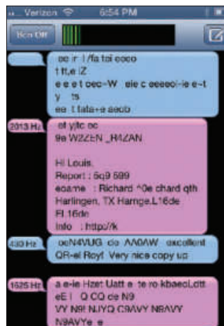
Figure 1 — PSK31PAN decoding multiple signals simultaneously.
