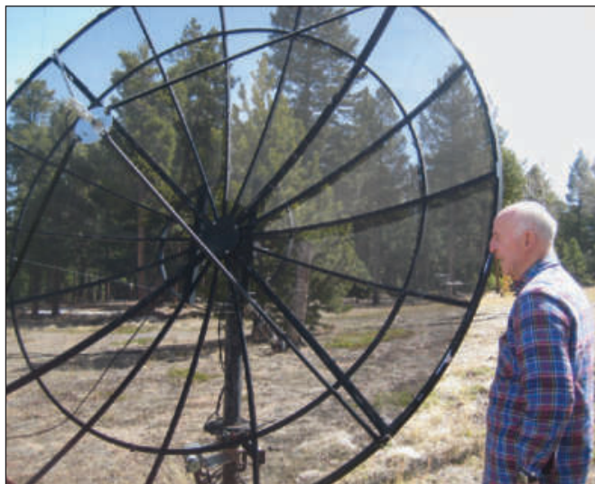
Figure 1 — The 14 foot dish on a 10 foot Rohn 45 tower with a triband patch feed for 435, 1269 and 2401 MHz.
