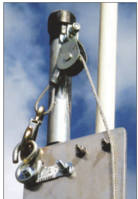
Figure 5 — The end of the winch cable is attached to the trolley as shown.
