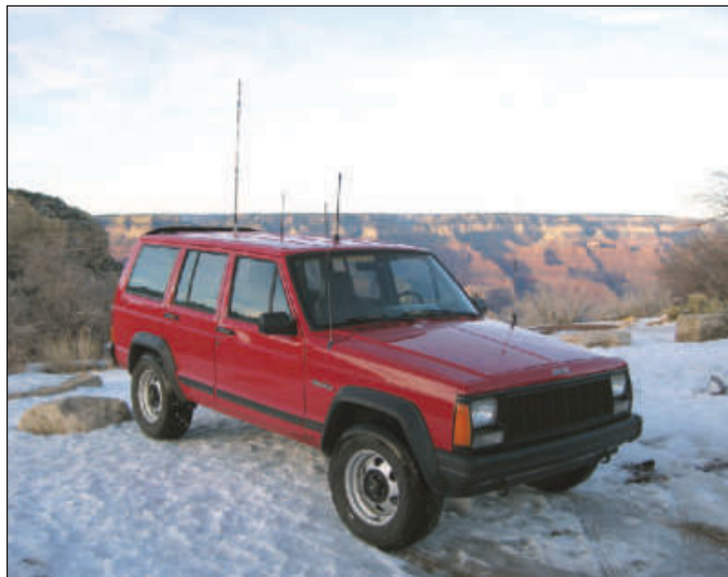
When parked close to the South Rim W7SAZ's Kenwood D700-equipped Jeep can crossband signals from down in the Canyon to a repeater and IRLP node up on top. [George Helser, W7SAZ, photo]
