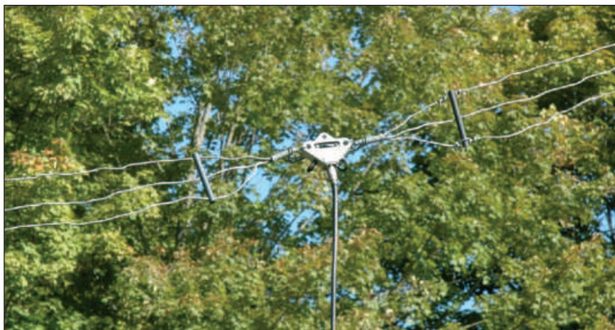
The center section of the DX-EE at a height of 25 feet.
