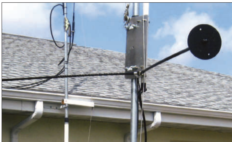
Figure 1 — The capacitance hat end loading arrangement on the repurposed CB whips used as radials.
