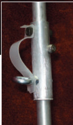
Figure 2 — A close-up of the removable antenna element splice showing the eyebolt that serves as a thumb screw for easy removal of the upper element. Also shown are the bolts that permanently attach the upper element to the tube and the flexible plastic that keeps the eyebolt from getting lost. [Doug Hart, AA3S, photo]
