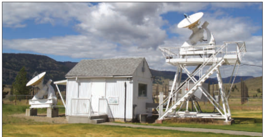
Figure 2 — The solar radio flux monitors at Dominion Radio Astrophysical Observatory near Penticton. Flux monitor 1 is on the left; flux monitor 2 is on the right.
