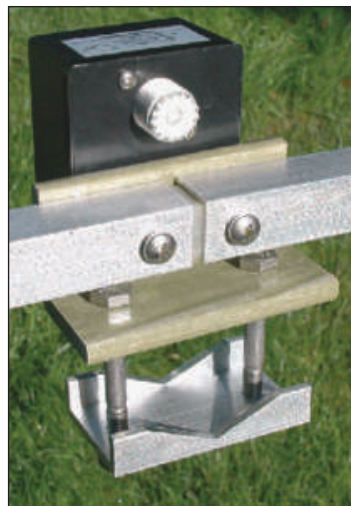
The transformer at the Omniangle feed point.
