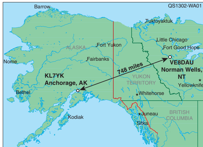
Figure 1 —This 6 meter contact between BP51 and CP65 spanned 748 miles using only 80 W and an attic loop.
