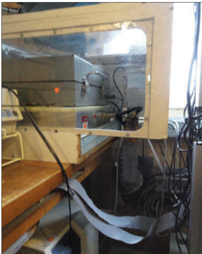
Figure 5 — The aluminum boxes contain the RF components for the A and B receivers.
