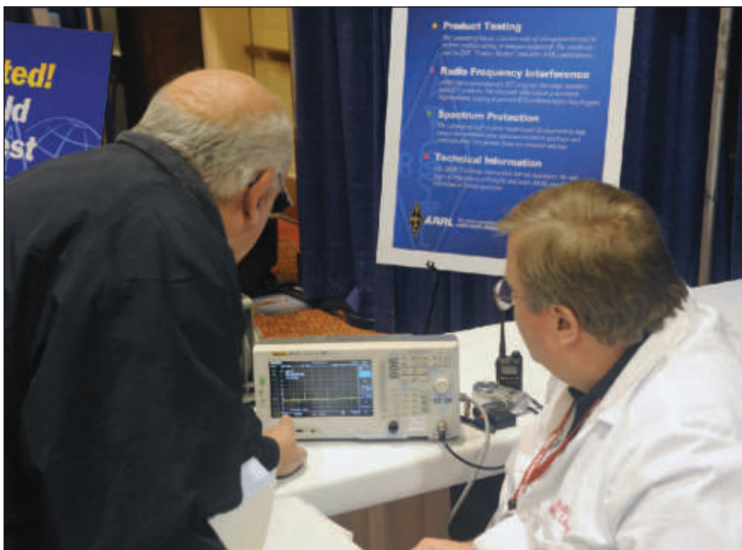
Figure 3 — Bob Allison, WB1GCM (in the white coat), checked the spectral purity of handheld radios for visitors at the ARRL National Convention at Pacificon last November. Most radios met FCC requirements, but there were a few surprises.
