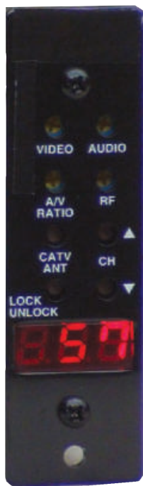
Figure 3 — Examples of an analog CATV modulator (left) and a high definition digital CATV modulator (right).
