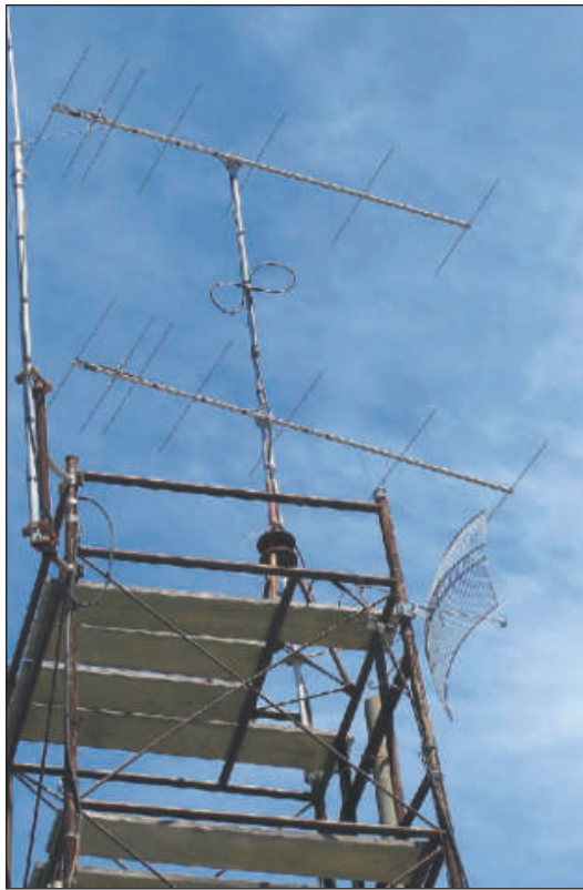
Figure 5 — This is the KH6HME beacon's 2 meter 7 element stack pointed at the USA mainland. [Fred Honnold, KH7Y,photo]
