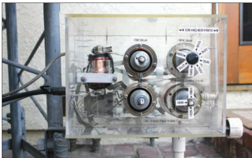
Figure 6 — 80 and 160 meter shunt capacitor adjustment calibration scales. C1, a 75 pF vacuum capacitor, is mounted vertically on the left.
