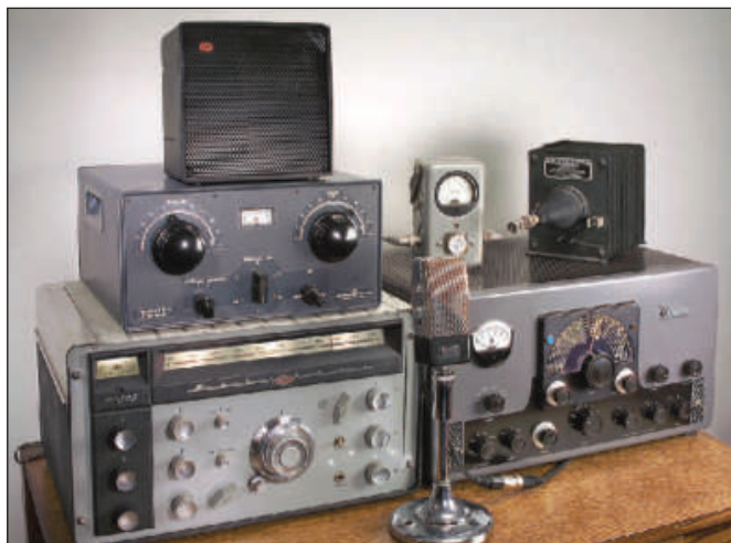
Figure 4 — The fully operational AM station the ARRL Lab crew has set up in HQ's new museum area. The station uses a Johnson Viking Valiant transmitter, National NC-303 receiver and a Millen 92200 transmatch.
