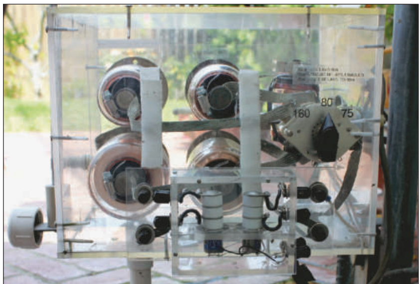
Figure 5 — Latching relays and band switch.
