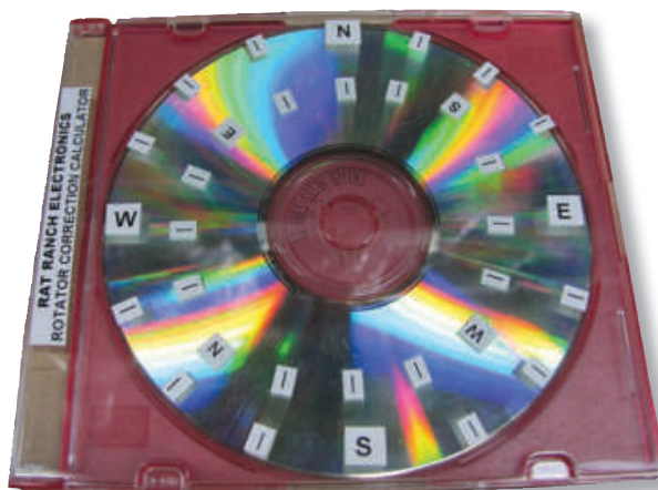
Figure 5 — If you’re having problems keeping your beam aligned, this handy calculator will help keep your aim true even if your rotator indicator isn’t. [Pat Bunsold, WA6MHZ, photo]
