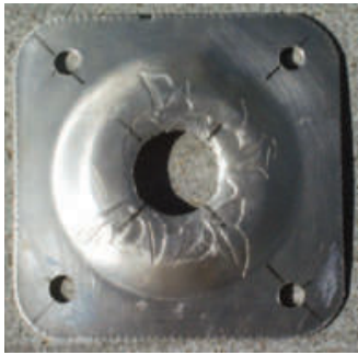
Figure 9 — A close up of what must be the most unusual guy ring I have ever seen. Made from an aluminum candy dish my spouse donated, it is very heavy gauge aluminum and has a floral design stamped into it.
