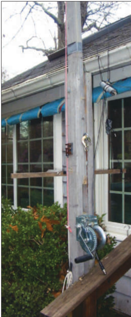
Figure 2 — Close up of the lower mast section. Note the boat winch, winch cable and snap hook used to safely raise and lower the mast.
