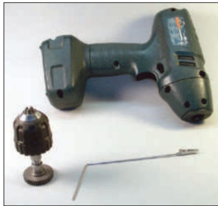
Figure 3 — Before discarding that worn-out drill, remove the chuck; it will make a great "third hand." [Van Johnson, KH6UX, photo]
