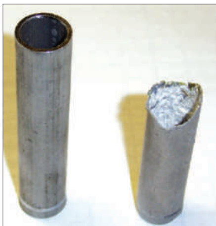
Figure 1 — Insect infestations in antenna elements can be much more than a simple annoyance. Many insects produce corrosive chemicals that can be very destructive to aluminum. Keep those end caps on. [Lawrence W. Stark, K9ARZ, photo]
