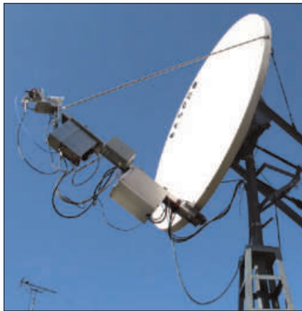
JA6CZD uses a 2.4-meter offset fed dish with a 30 W solid state power amplifier.
