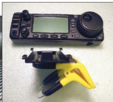
Figure 2 — These paint clamps were found at a home center for $3. They proved to be perfect for mounting the ICOM 703 remote head.
