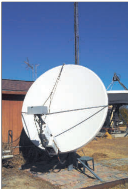
W5LUA uses 2.4-meter offset fed dish and a Travelling Wave Tube amplifier mounted on the feed support.
