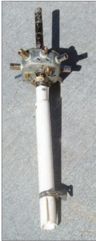
Figure 7 — In December 2007 QST, I wrote an article about the “Octopus Antenna.” This adaptor fits it to the new mast, which is somewhat larger in diameter.
