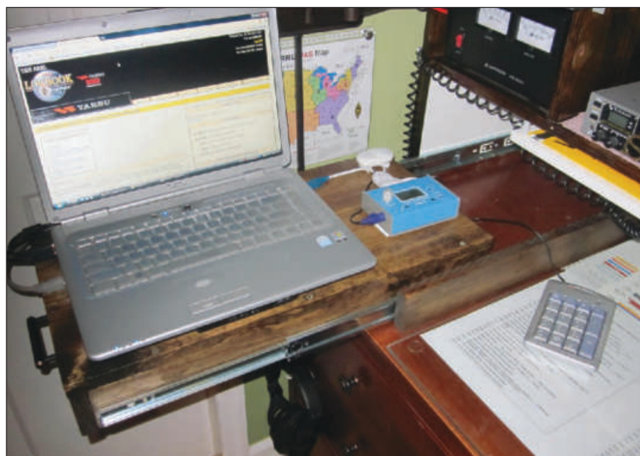
Figure 4 — The computer sits on a wooden box mounted on drawer sliders. It can be slid out for operating and then back in when not needed.
