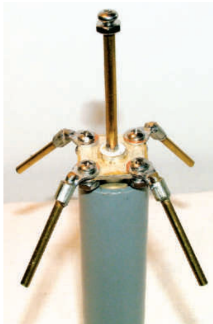
Figure 1 — Close up of the 1/4 wave drooping ground plane for the 1200 MHz band.
