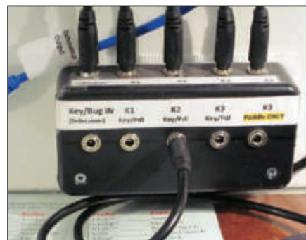
Figure 6 — This homebrewed key cable patch panel places all the key inputs in an accessible location.
