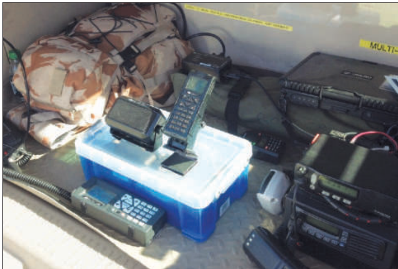
Figure 1 — Everything from BGAN satellite to HF ALE was used during the workshop. Barrett ALE gear was used to establish NVIS communications with regional sites. [Photo courtesy David Witkowski, W6DTW]
