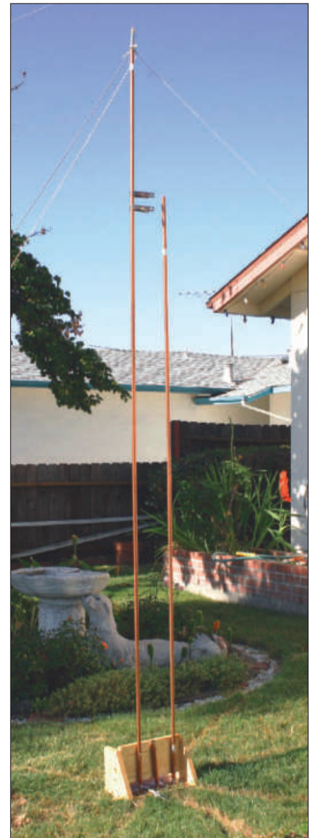
Figure 5 — View of the 10-12 meter coupled resonator monopole, one of the smaller antennas used to validate the design process. It had a bandwidth of 17.7%
