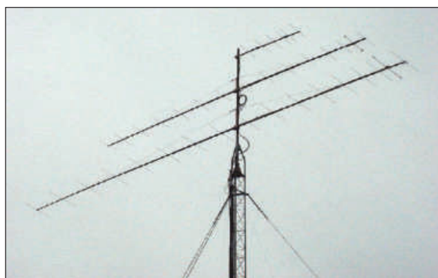
Figure 4 — W5UWB's 222 MHz antenna array for the record breaking 222 MHz m/s contact on December 14. The bottom antenna is a 17 el 2 meter (recently replaced with a 21 el 8wl). The middle antenna is the 222 17 el at 54 feet. The top antenna is 1/2 of the 11 element 222 with which he set the E s record by contacting W6QIW on February 14, 2000. [John Butrovich, W5UWB, photo]
