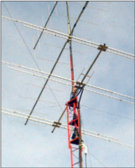
Figure 2 — Close-up view of the two band antenna. Note the beta match on the 10 meter driven element.
