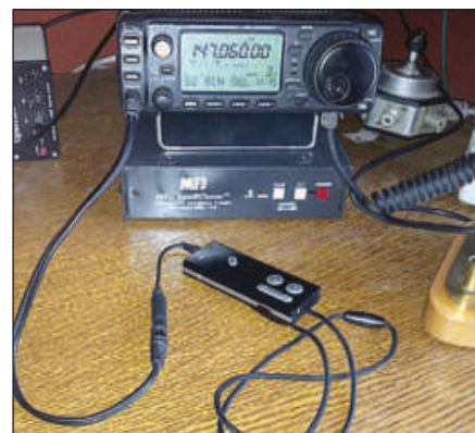
Figure 2 — Modern Bluetooth enabled hearing aids permit the user to interface their devices to a variety of external audio sources, including your transceiver. [Don Pomplun, K2BIO, photo]
