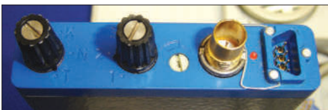
Figure 2 — This is a top view of the PR-35. From the left are the function control, channel selector, squelch control, antenna connector and accessory connector.
