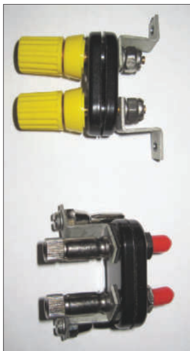
Figure 8 — Here are the two window line adapters, one for an MN-2700 tuner and the other for an MFJ RF ammeter. [Evan Rolek, K9SQG, photo]
