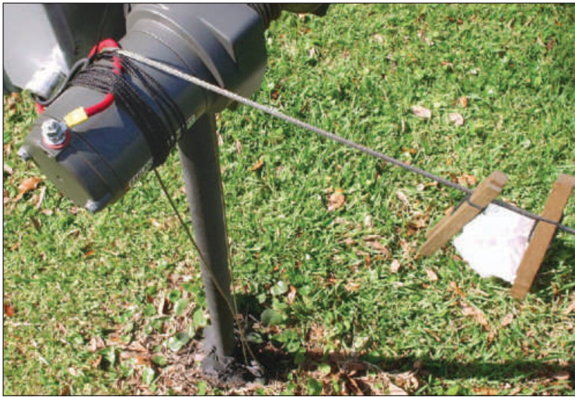
Figure 5 — In “clothesline mode” the cable runs from its taped point on the tower, over the top of the winch and down to the post pulley. This keeps the cable well above ground when not in use. [Pat Hamel, W5THT, photo]
