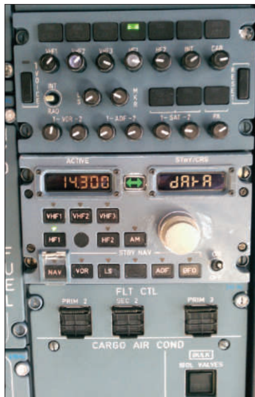
A close up of the radio control panel on the flight deck. Ron can operate on 160 through 12 meters, but is limited to USB or AM only.
