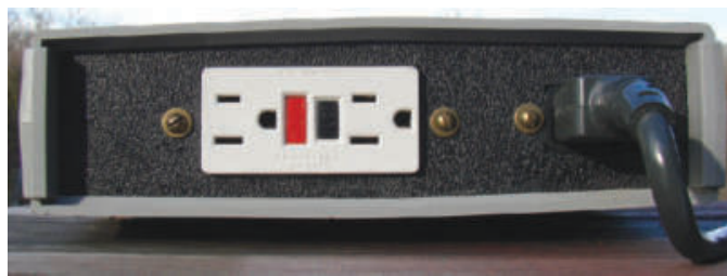
Figure 3 — Socket side view of the overvoltage protection device. The input power is supplied on the right, while the GFCI sockets provide power to protected devices.
