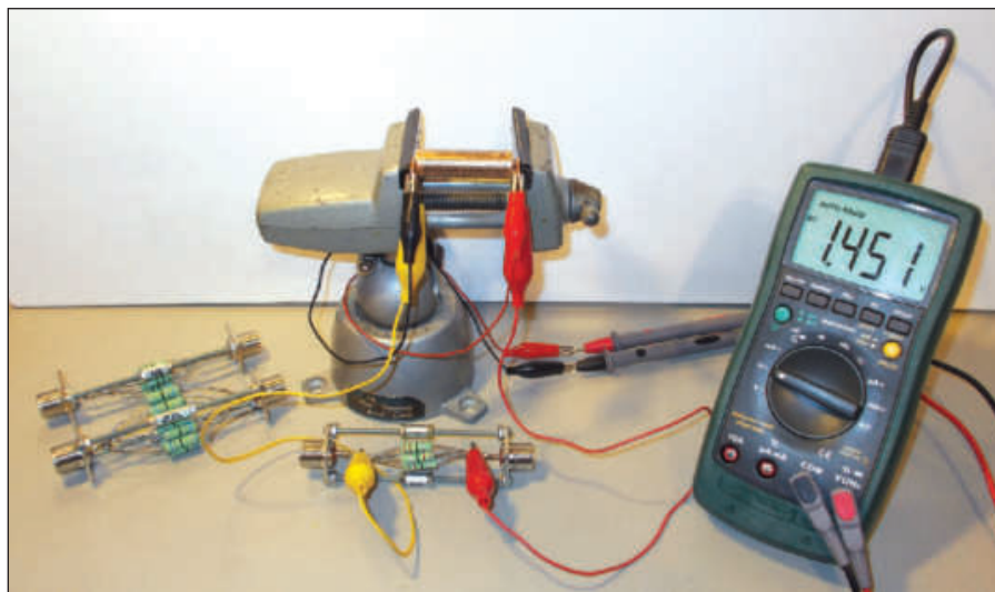
Figure 1 — The test setup for battery load tests. Loads are constructed from multiple resistors in parallel. The battery is held between two copper pennies in a vise with insulating jaws. Clip leads are used to connect the battery, load and logging DMM.
