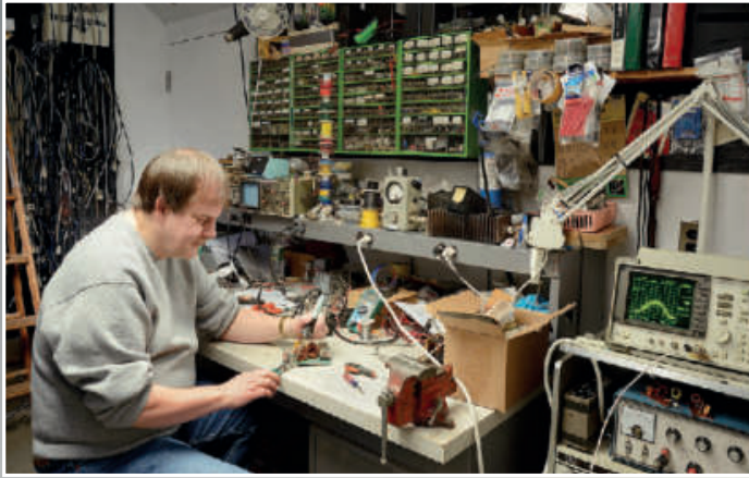
W1AW engages in building and repairing as well! The station's workshop contains most of the necessary tools and components to accomplish these activities. W1AW station operator Scott Gee, WB9RRU, is tackling a relay board that will be used in an antenna switching project.
