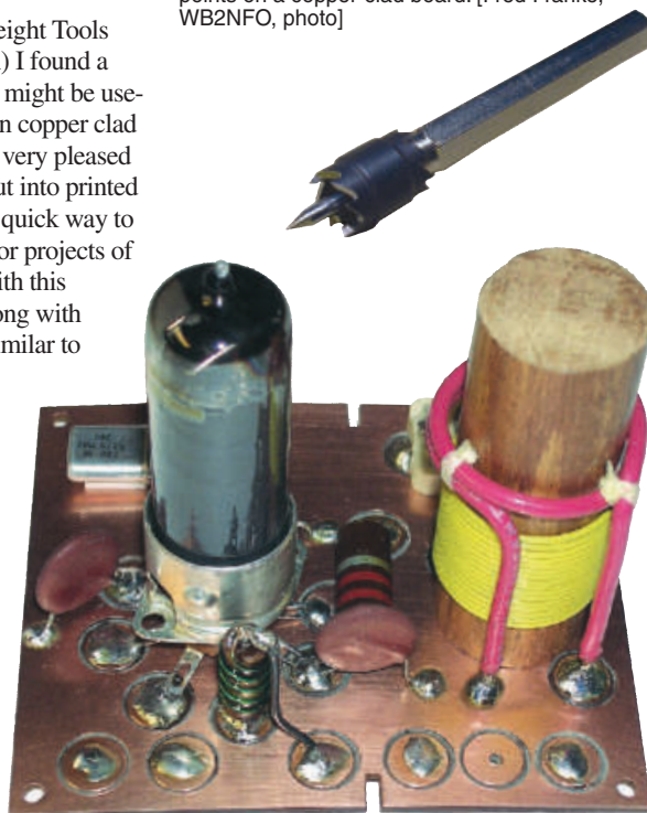
Figure 7 — The cutter makes 8 millimeter diameter connection “pads” in copper-clad boards allowing for quick and easy circuit construction. [Fred Franke, WB2NFO, photo]
