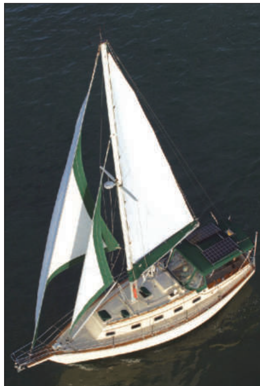
The Brisa del Mar at sail. Note the solar panels at the stern.
