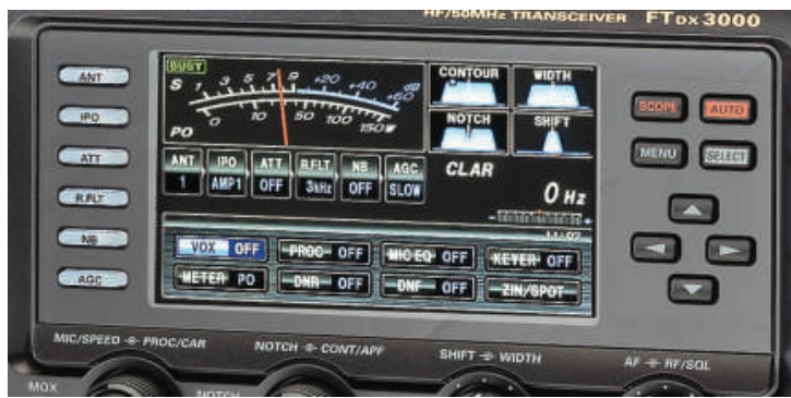
Figure 4 — The FTdx3000's TFT display includes a virtual analog S meter. Icons offer visual information on various DSP filter and control settings at a glance. When the band scope is active, it replaces the information at the bottom of the display.
