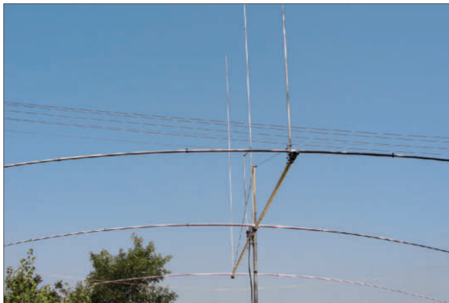
The Garden Beam used in the backyard of Tomi Pekarik, HA7RY. For best results, the mast extension supporting the boom guys should be non conductive.
