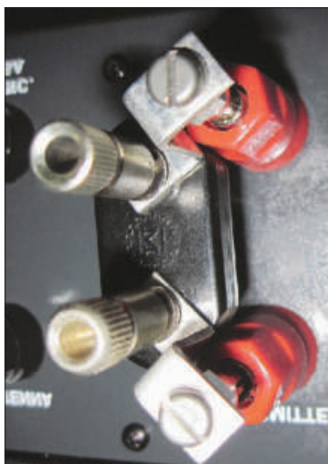
Figure 9 — Here is the adapter installed on the RF ammeter. [Evan Rolek, K9SQG, photo]
