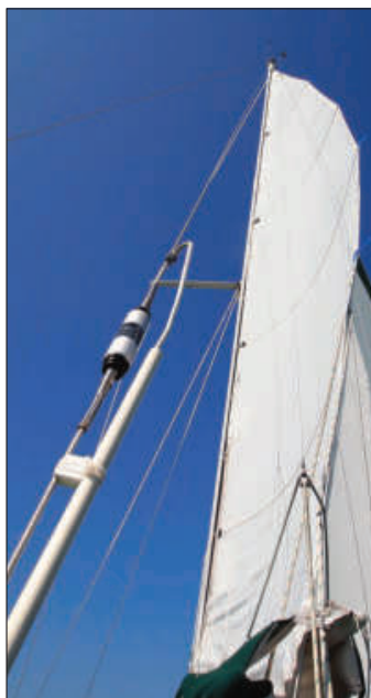
WQ3W's seagoing antenna along an insulated portion of the backstay.
