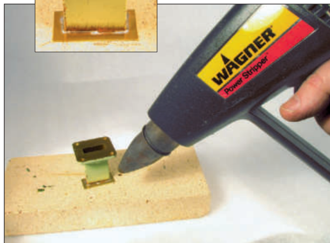
Figure 2 — A heat gun can be used to solder larger assemblies.
