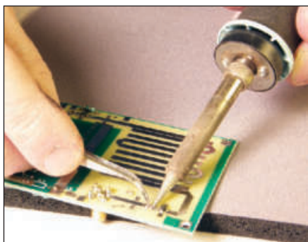
Figure 4 — You can use tweezers to hand solder surface mount components. A mouse pad provides a non-slip base.
