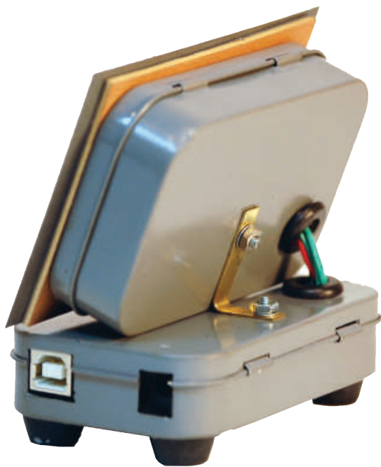
Figure 5 — Put the #4-40 mounting bolts for the bracket through from the inside to keep them from interfering with the Arduino headers.
