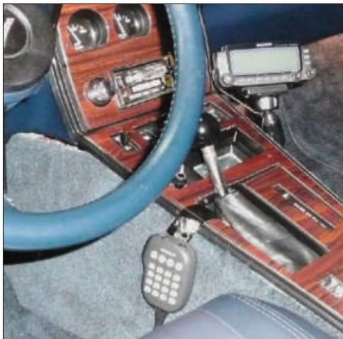
A flexible mount near the center console holds the TM-700 control head. The microphone is nearby.
