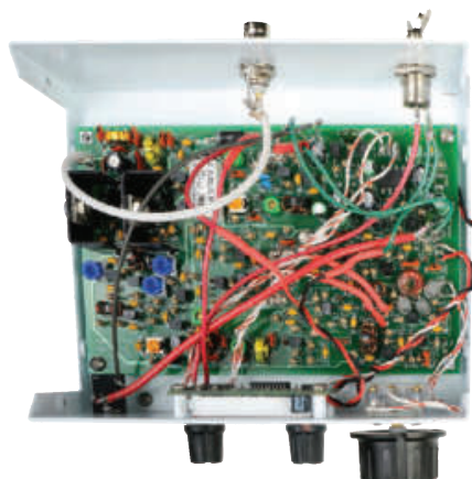
Figure 3 — One side of the completed KD1JV digital dial, showing the surface mount parts. The penny gives an indication of how tiny this PC board and components are.
