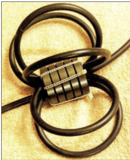
Figure 1 — My six turn balun, too big to fit inside a 4 inch diameter PVC pipe.
