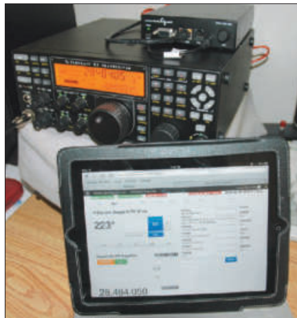
The RemoteHamRadio K3/0 with the Remote Rig interface and the Apple iPad I was using at the time.
