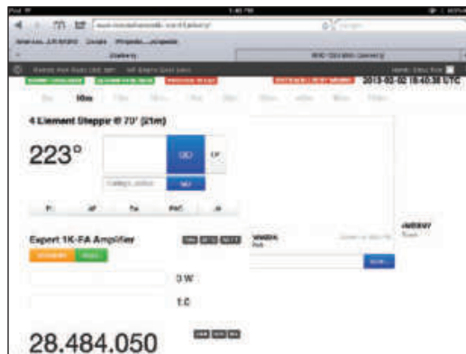
The RemoteHamRadio console screen. You select your stations and control their antennas and amplifiers here. There is also a "chat" window so that you can exchange messages with other operators.
