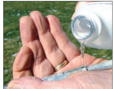
Figure 5 — A little rubbing alcohol applied to the junction of two stuck antenna elements can soften whatever impurities have become lodged between the sections, allowing them to be more easily separated. [Lorraine Wilkinson, W7RFC, photo]
