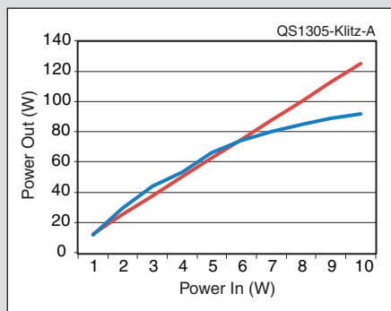
Figure A — Power output versus input, as measured in the ARRL Lab. A straight line (red) is shown for comparison.
