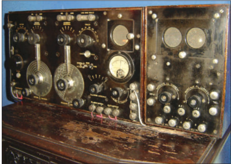
Figure 1 — This is the IP-501 receiver and matching two stage audio amplifier I discovered in Cecil’s basement and restored. It was used aboard the United Fruit Company ship S. S. San Jose .
