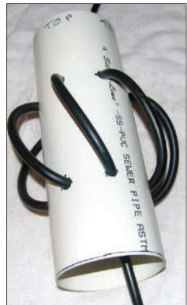
Figure 3 — A side view of the balun assembly.
