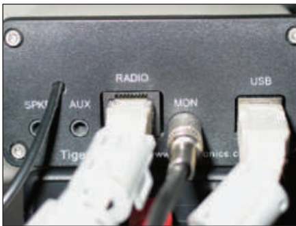
Figure 2 — Details of the additional cable attached to the rear of the SignalLink. A grommet would reduce abrasion of the cable jacket.
