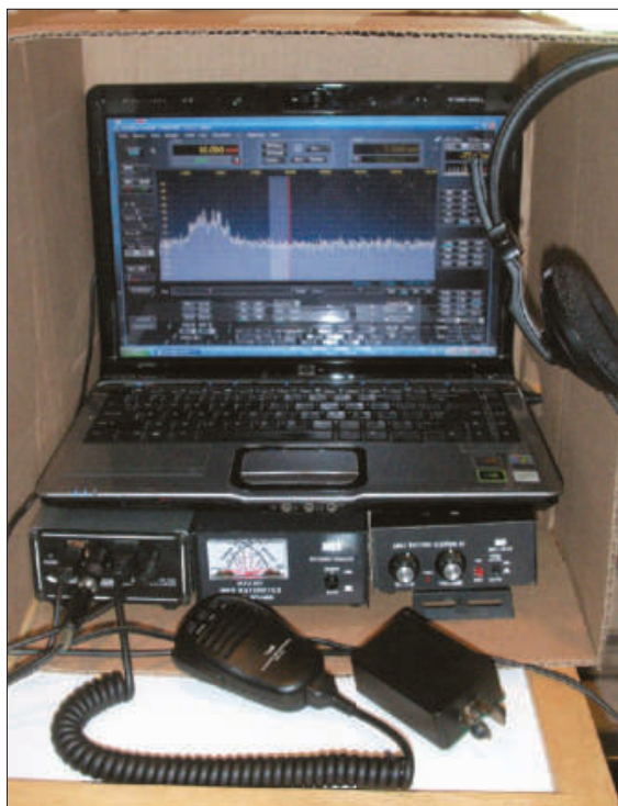
Figure 3 — The SDR transceiver teamed with a lightweight laptop computer and enclosed in a cardboard box light shield brings high tech to the mountain summits.
