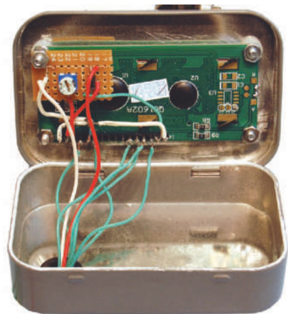
Figure 6 — Inside the display tin: The small piece of vector board in the top left of the photo holds the diode and trimmer as well as ground and power bus wires.
