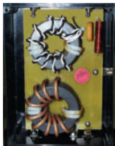
Inside of Matching Unit
