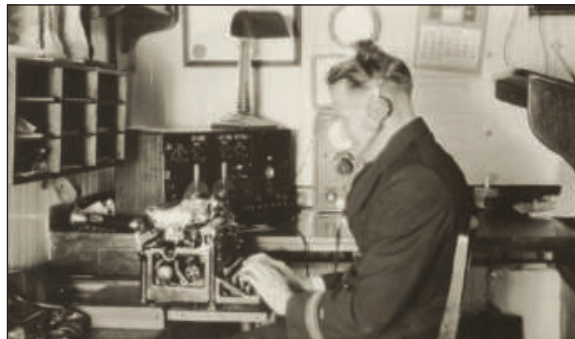
Figure 2 — Cecil Williams at “the mill” copying traffic. The receiver is the later model IP-501A. The calendar in the background suggests this photo was taken in July 1928 aboard the S. S. Santa Marta .
