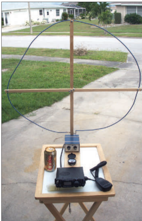
Figure 2 — This first attempt at a small loop theoretically should not have worked but stations in New Mexico and North Dakota didn't know this.
