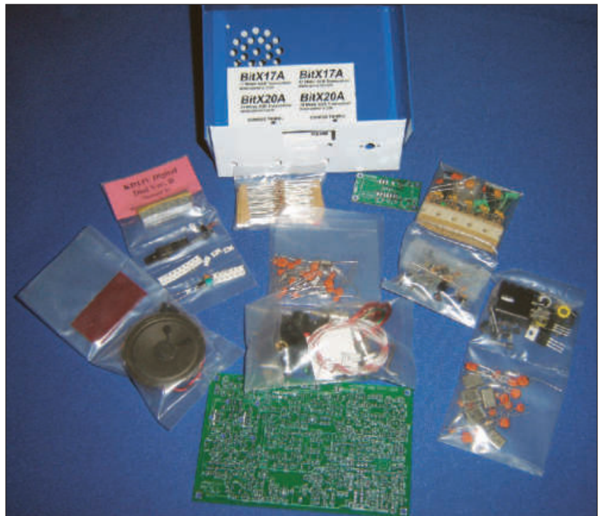
Figure 1 — Contents of the Hendricks BitX17A 17 meter SSB transceiver kit package. The material came well packed in thick, clear plastic envelopes.
