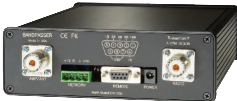
Figure 5 — The AS-419 Bandpasser offers several options for automatic filter switching via application of 12 V dc to the appropriate pin on the REMOTE jack or as part of a ShackLAN network. The rear panel network connector type has changed since this photo was taken. Newer versions have a pair of 6-pin modular jacks for the network connection in place of the green screw terminals.
