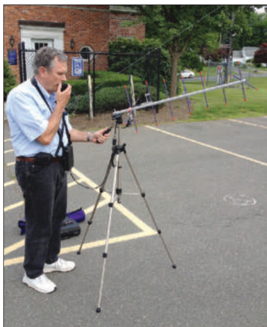
Mark Spencer, WA8SME, using an Arrow 146/437-10 antenna to make satellite contacts from the W1AW parking lot.
