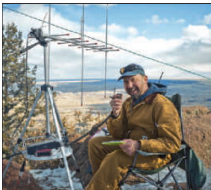
You don't need large antennas to enjoy a VHF contest! Stu Turner, W0STU, had great fun in the 2011 ARRL January VHF Contest with a 6 meter dipole and a small dual-band Yagi for 144 and 432 MHz. Of course, his location at the top of Mount Herman in Colorado helped his QSO rate! [Stu Turner, W0STU, photo]
