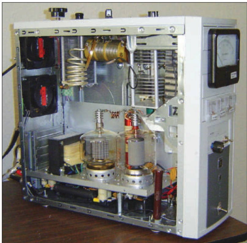
Figure 4 — This amplifier uses two 4-400A tubes to generate 600+ W on 80-10 meters. It uses an external power supply to provide 2500 V. The filament transformer is installed next to the tubes. [Richard Calhoun, W6DZT, photo]
