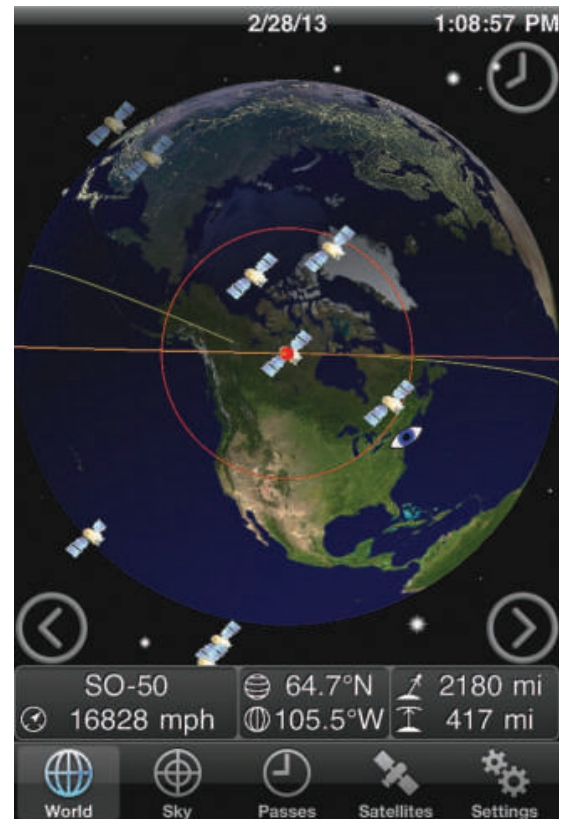
A glimpse of the GoSatWatch app for the iPhone and iPad showing the position and footprint of Saudi-OSCAR 50.
