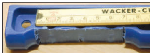
Figure 2 — Notch cut into the tennis ball thrower to accommodate the fishing reel mount.
