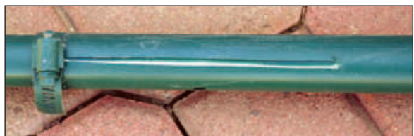
Figure 1 — A slot is cut in the wall of the lower tube and a screw clamp is used to compress the lower tube on the upper one holding them together. Green paint was applied to help conceal the antenna. [John Marshall, WA7BSR, photo]
