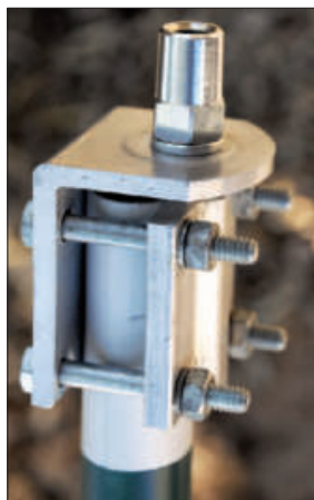
Figure 1 — A slot is cut in the wall of the lower tube and a screw clamp is used to compress the lower tube on the upper one holding them together. Green paint was applied to help conceal the antenna. [John Marshall, WA7BSR, photo]
