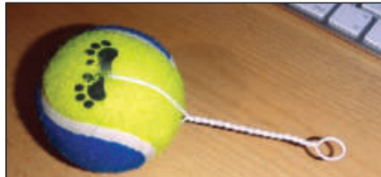
Figure 4 — A tennis ball prepared with the wire pigtail and eyelet.
