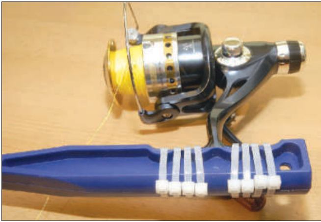
Figure 3 — The cable tie method of securing the reel to the tennis ball thrower handle.
