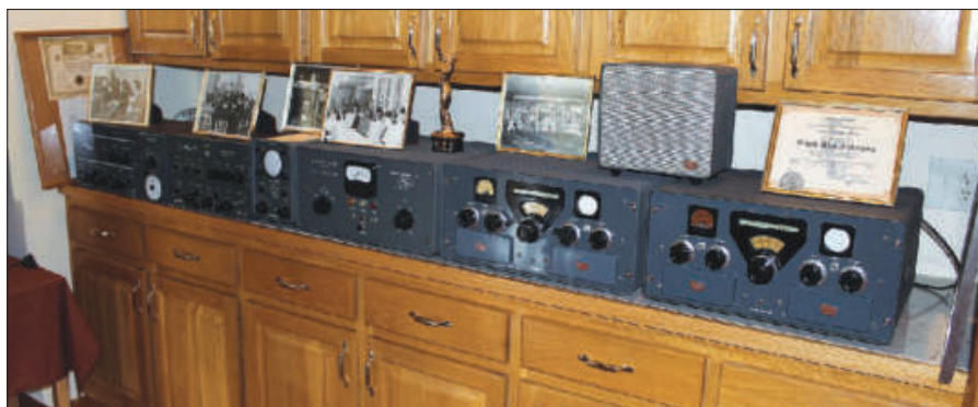
A Central Electronics transmitter lineup: 10B exciter, 458 VFO, 20A exciter, MM-1 monitor scope, 600L amplifier, 100 V exciter and 200 V exciter. All units shown are from Wes Schum's personal collection. [George Maier, W1LSB, photo]
