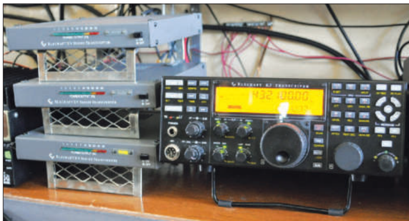
Figure 5 — Using modified paint roller screens to separate stacked equipment improves air flow and cooling while also eliminating a cluttered look in your shack. [Sebastian Acosta, W4AS, photo]
