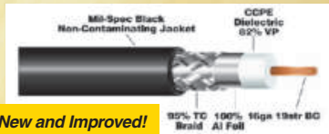
218XATC RG8X (240UF) Foil+TC Braid Non-contaminating Direct-Burial Ultra-Violet Resistant Jacket. W/SILVER-TEFLON PL259 & WEATHERPROOF HST each end.
