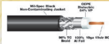
25400F 400-FLEX (RG8/U TYPE) FLEXIBLE LOW LOSS Non-contaminating Direct-Burial Ultra-Violet Resistant Jacket. W/SILVER-TEFLON PL259 & WEATHERPROOF HST each end.
