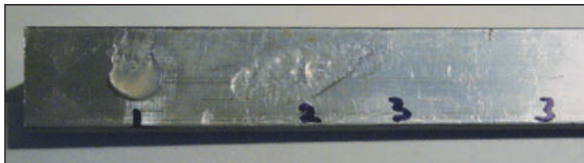
Figure 1 — Here are three different levels of HSC on an aluminum bar. Number 1 is a big blob that will inhibit heat transfer. Number 2 is a big smear (sometimes looks like ridges), which is better but still too much for good heat transfer. Number 3 shows a correct application where the HSC is almost invisible. [Phil Karras, KE3FL, photo]
