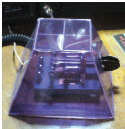
Figure 5 — This small trapezoidal shaped plastic bin is inexpensive and can be easily modified to protect your key or paddle from dust, dirt or spills. [Bill Parker, KA3IXF, photo]
