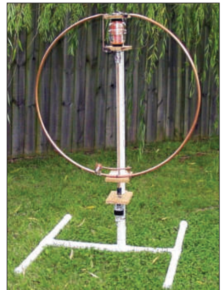
Figure 1 — The author's small magnetic loop antenna. A stepper motor is used to drive a vacuum variable tuning capacitor to resonate the loop at the operating frequency.
