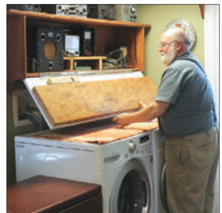
Figure 4 — Here I am lowering the door. The workbench top is closed against the back of the door.
