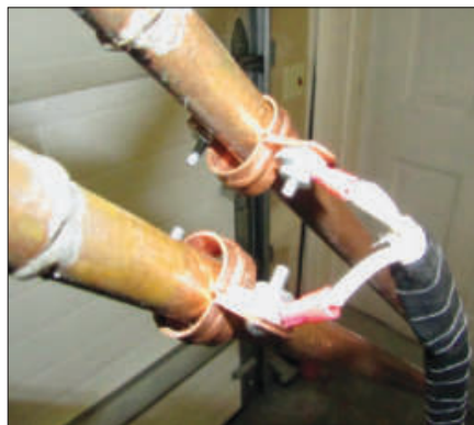
Figure 4 — Detailed view of the connection of the loop balun to the Q section.
