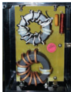
Inside of Matching Unit
