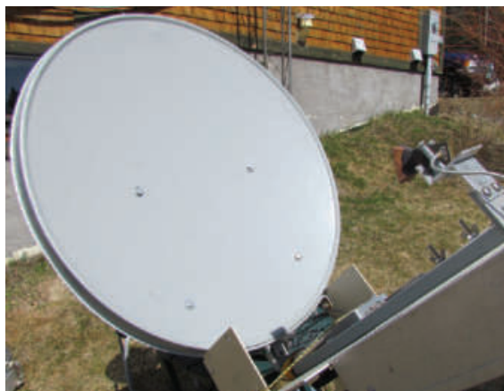
Figure 3 — An offset fed dish is peaked for sun noise when the shadow of the feed is at the bottom of the dish's edge.
