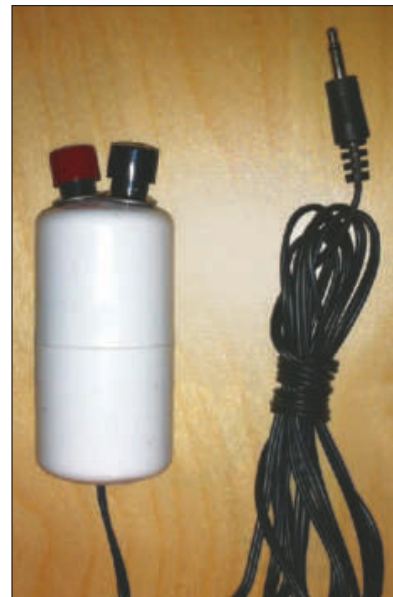
Figure 7 — The completed PTT switch fits nicely in the palm of your hand. The black button functions as a regular PTT while the red button is a push-on, push-off type for those long ragchews. [Thomas Nolan, W3EX, photo]
