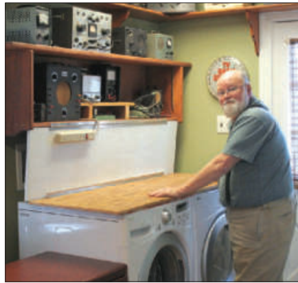
Figure 6 — The “Murphy bench” is ready to go. Note the power strip below the piano hinge.
