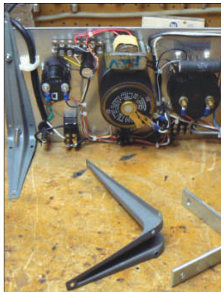
Figure 6 — Angle brackets make a solid and steady support when working on equipment panels. [Steve Gilbert, K1SG, photo]
