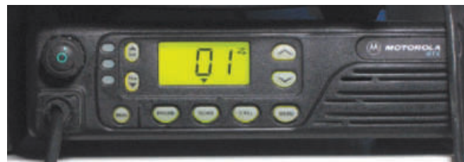
Figure 1 — The author's 900 MHz band Motorola GTX 900 scanning all channels.
