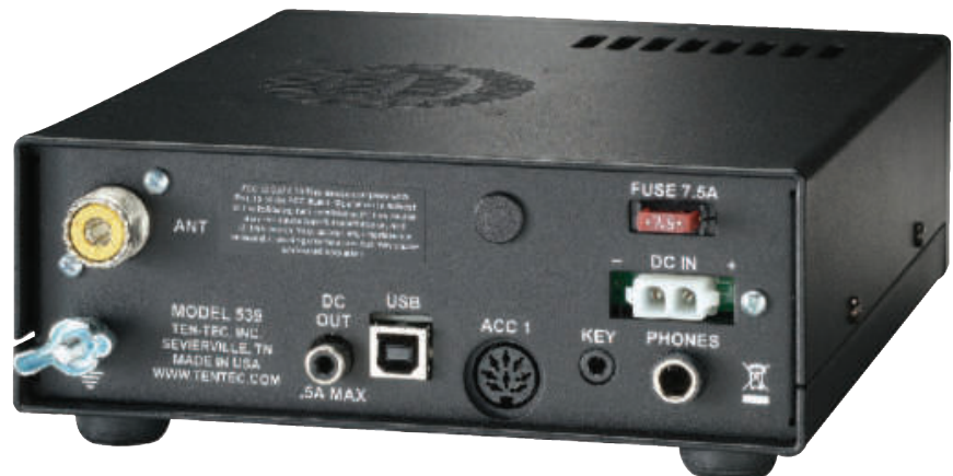
Figure 1 — The TEN-TEC 539 rear panel showing the available connections.
