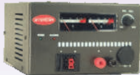
JTPS35BCMA $139.95 35 amp with meters, variable, battery backup and Anderson Connectors
