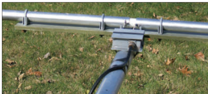
Figure 3 — A balun transformer inside the grey box feeds the driven element.
