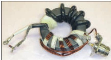
Figure 5 — The balun transformer, shown with a 22 \Omega test load attached to 22 \Omega coax cable winding input, is wound with trifilar #14 AWG enameled wire on an Amidon FT-240-61 core. Amidon part from www.amidoncorp.com/ft-240-61 .
