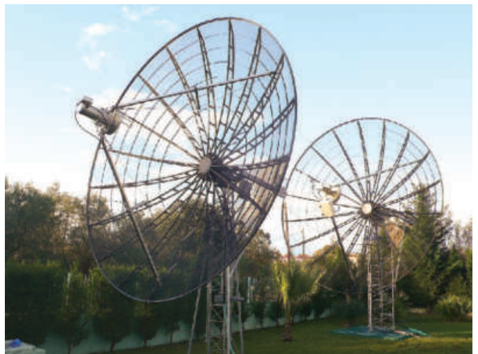
The 20-foot dishes Jimmy Vitorakas, SV1BTR, uses on 432 MHz, 1.2 GHz and 2.4 GHz to place at the top of the All Band, CW Only category year after year. [Jimmy Vitorakas, SV1BTR, photo]
