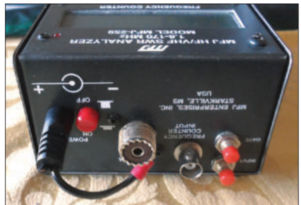
Figure 3 — By inserting the appropriate dc plug into the external dc jack, you can disable the internal batteries preventing accidental discharge and possible corrosion damage. [Mat Breton, AB8VJ, photo]
