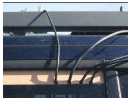
Figure 5 — A small piece of wood or rigid insulation is easily shaped and notched to make a feed line pass-through for your mobile installation. [Alex Burr, K5XY, photo]
