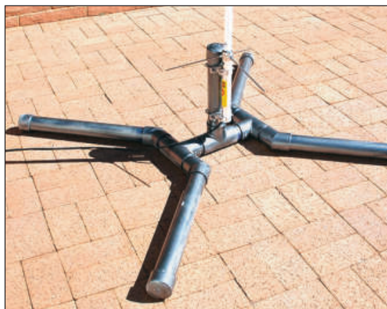
Figure 4 — This PVC mount is simple and inexpensive to build. It is adequate for small, low wind-load antennas. [Ed Toal, N9MW, photo]
