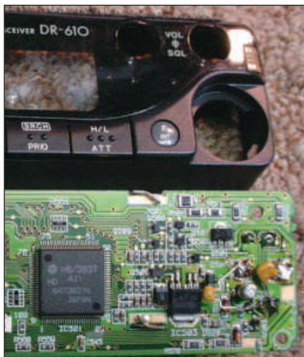
Figure 1 — The capacitors, visible on the right, are mounted on the back of the control head circuit board, behind the rotary encoder. [Kirk Ellis, KI4RK, photo]
