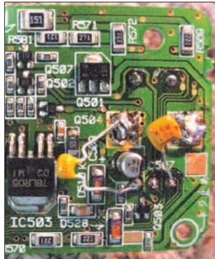
Figure 2 — This is a close-up view of the capacitors mounted to the back of the encoder. [Kirk Ellis, KI4RK, photo]
