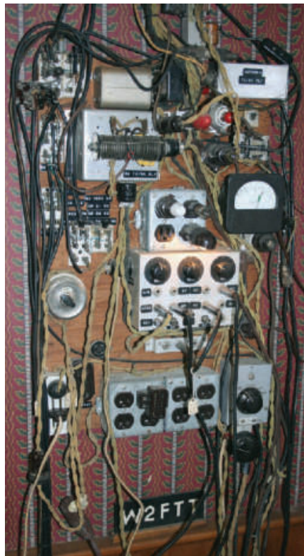
Figure 6 — Here is Earl's relay and control panel, which was rescued by Al Klase, N3FRQ. The panel was still live and Al had to cut the power when we came to remove it. [Al Klase, N3FRQ, photo]
