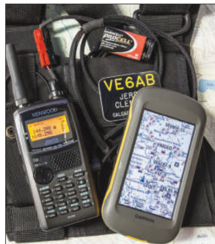
The Garmin Montana and a Kenwood TH-D72 transceiver. [Jerry Clement, VE6AB, photo]
