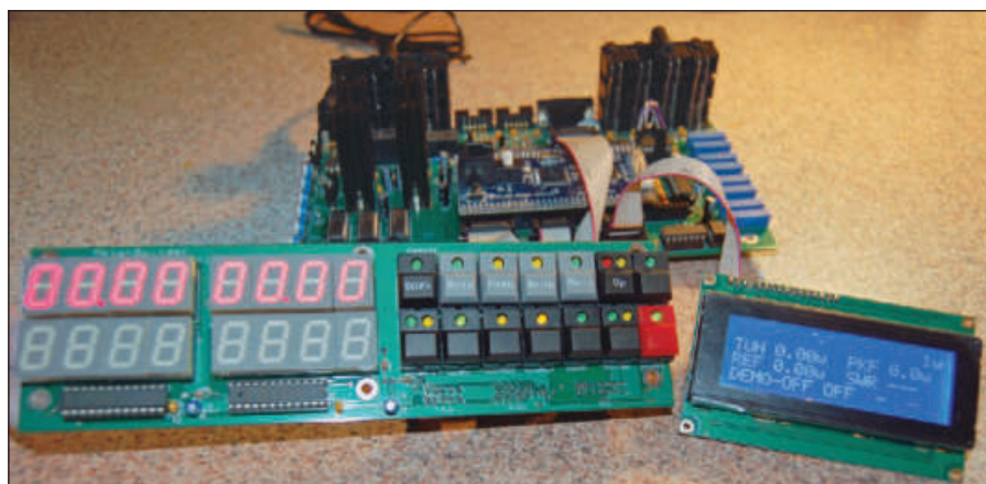
Figure 7 — The assembled circuitry, ready for the initial checkout and testing.
