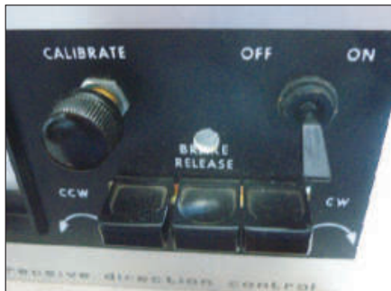
Figure 1 — View of the front panel showing the added LED (D4) indicator that shows that the brake is disengaged.
