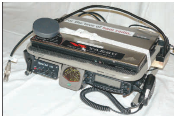
Figure 3 — Folded up and ready to travel, the digital station even has room for a gooseneck lamp. [Jon Rudy, K3QF, photo]
