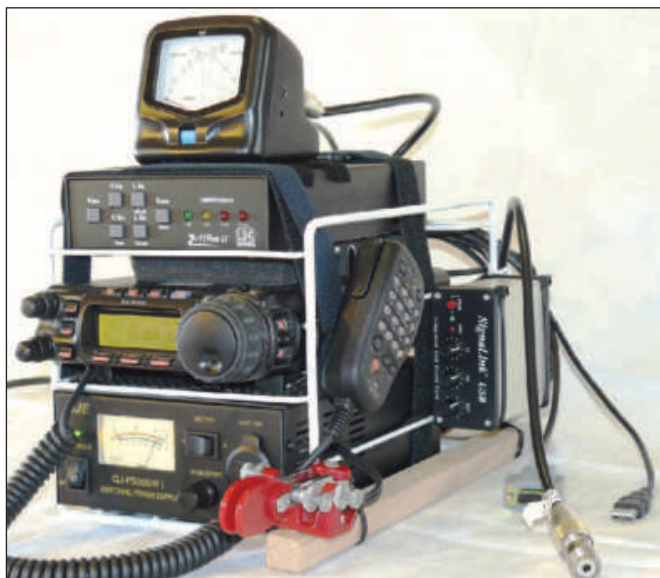
Figure 4 — A wrap rack provides a three tier frame to support a power supply, transceiver and tuner, with space on top for a wattmeter and room on the side for a SignalLink and paddle. [Jon Rudy, K3QF, photo]
