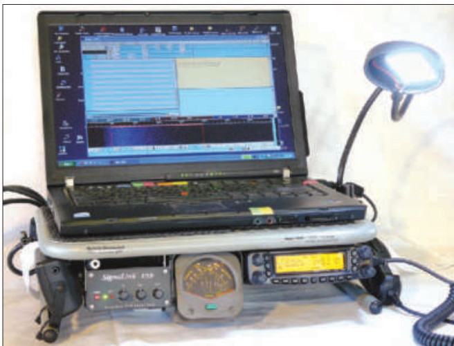
Figure 1 — An Allsop monitor stand makes a great base for a digital go-kit station. [Jon Rudy, K3QF, photo]
