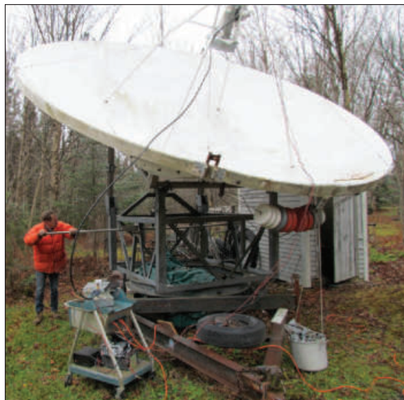
Figure 1 — Ready to go for EME on 1296 MHz. The equipment is on a moving cart to minimize feed line length. Rotation by W1AIM.
