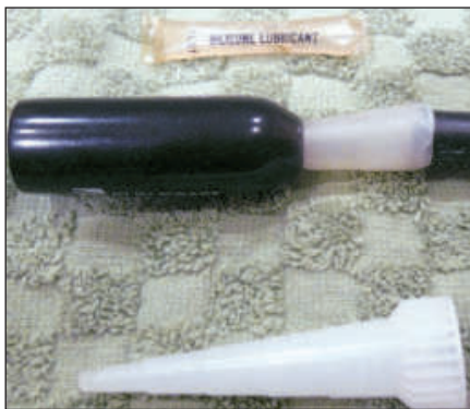
Figure 4 — The conical applicator tip from a tube of glue or sealant can be converted to a handy tool that makes fitting weather seal boots onto coax a simple job. [Michael Buck, K6BUK, photo]
