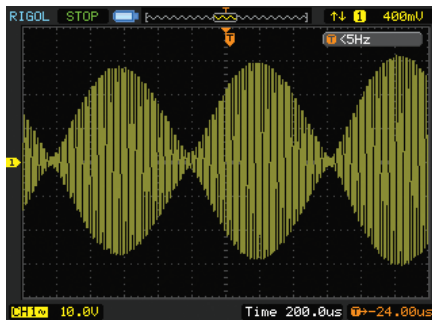
Figure 9 — Two-tone RF-modulated transceiver output measurement with the Rigol DS1052E using the same test setup as for Figures 4 and 5.
