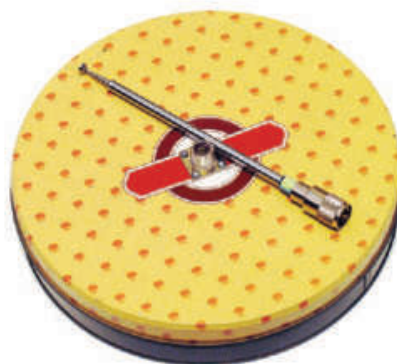
Figure 6 — Deluxe 10 inch cookie tin with telescopic whip in a UHF connector. Whip and coax are put inside the can for storage.
