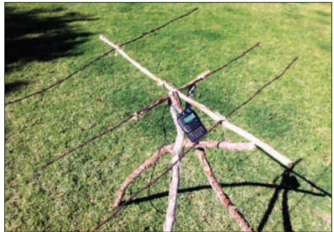
Figure 5 — The completed barbed wire beam on an Adirondack-style display stand.
