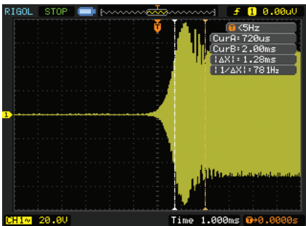
Figure 7 — A close-in view of the transceiver overshoot duration using the Rigol DS1052E.
