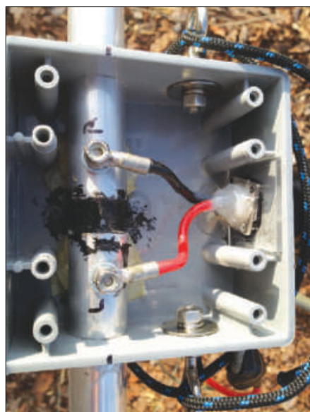
Figure 6 — The junction box. The end of the choke balun is at the top with the keeper in place. The black coating on the Delrin in the gap makes the connection more weather resistant. Silicon sealant is also used liberally on the box and on the trap ends where the tubing exits.
