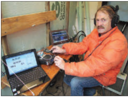
Figure 2 — W1AIM operating CW on EME. The laptop in the foreground calculates the Moon's position; the laptop in the rear displays the bandscope waterfall.
