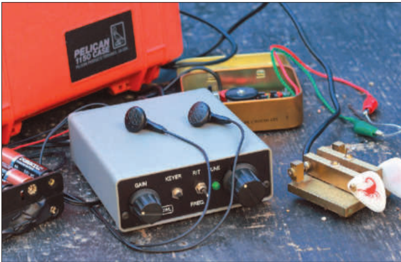
The Small Wonder Labs DSW-II transceiver is the centerpiece of the author's kayak QRP portable station.
