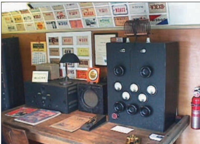
The original 1932 station. From the left: A 1932 Hammarlund Comet Pro receiver, speaker, coil box and the QSL card of the first owner, Dare Aucott, W3CRY, of Atlantic City, New Jersey; a well-made homebrew 300 W transmitter built by Joe Hoffman, W2DST, of New York. On the table and wall: the 1933 station log, license, lamp and chair of the late Earl Abbott, W2FTT, Manahawkin, New Jersey, and a collection of 1930s QSL cards from southern New Jersey hams. [John Dilks, K2TQN, photo]
