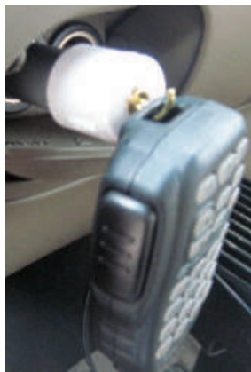
Figure 5 — A few pieces of PVC, some junk box parts and some sandpaper comes together to make a mobile mic holder. [Ted Pirolli, KD8HYT, photo]
