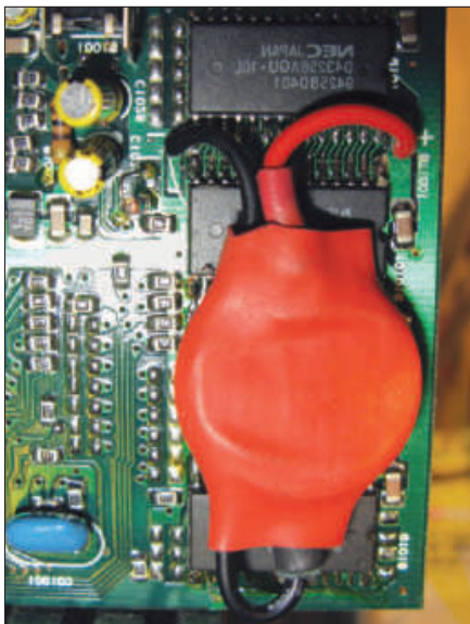
Figure 3 — The new cell, double insulated and installed on the DVR-2 board. [John Grout, KT4AD, photo]
