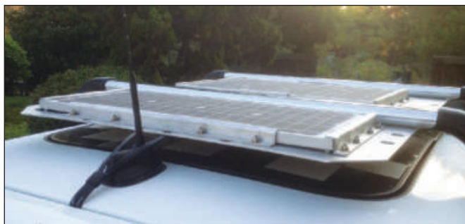
A close-up view of the solar panels with the wiring snaking into the rear hatch.
