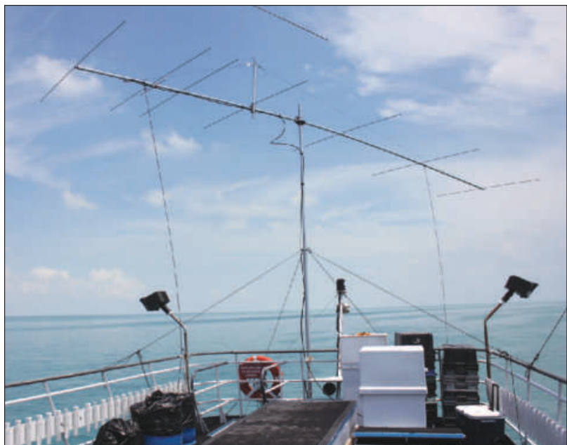
Figure 1 — K4N’s station #2 used this 6M7JHV Yagi. This antenna accounted for the majority of the contacts. [Marshall Williams, K5QE, photo]
