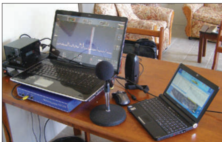
The primary station was a Flex-3000 Software Defined Radio, an Astron 20 A switching power supply, some powered speakers, and a Heil HM-12 microphone.
