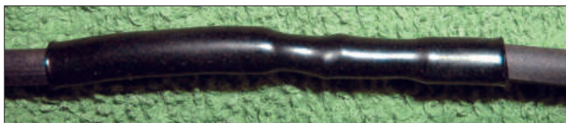
Figure 4 — Finish the splice with a piece of heat-shrink tubing for a neat and sturdy splice. [Frank Ingle, KG4CQK, photo]
