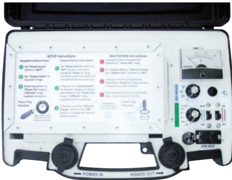
Figure 6 — The solar power system is completely contained in a modified pistol case. The rectangular area at left is the accessory box. The foldable solar panel stores underneath it.
