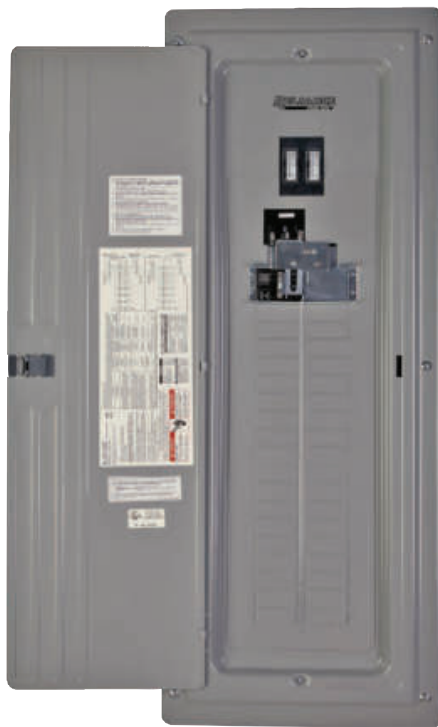
Figure 3 — One type of transfer switch is the whole house service disconnect switch. This box would go between the usual service entrance (circuit breaker) box and the input line. [Photo courtesy Reliance Controls Company]
