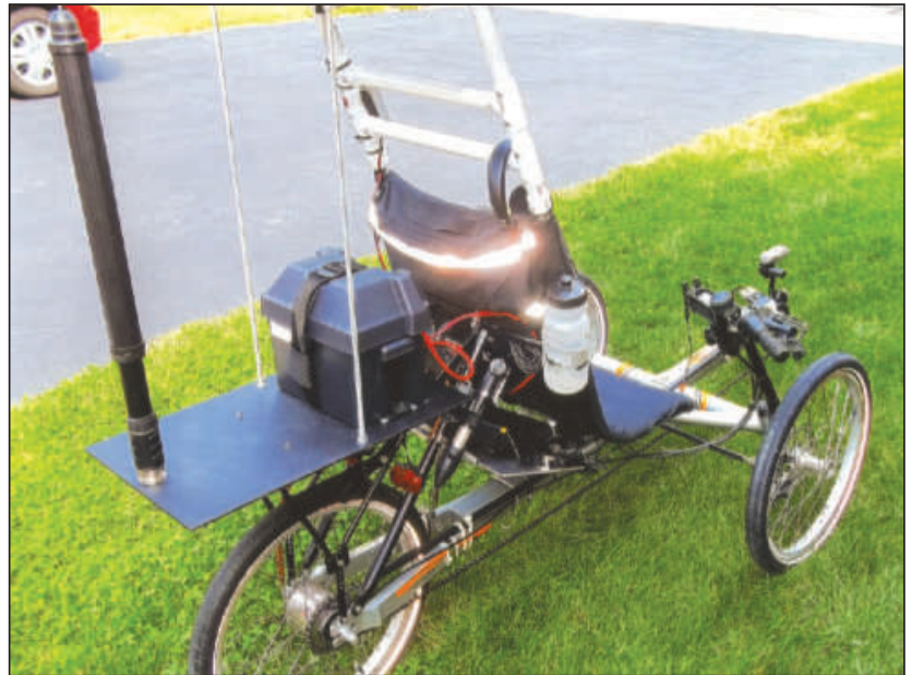
A view of the trike showing the rear panel and ATAS mobile antenna.
