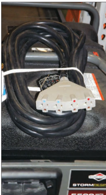
Figure 2 — An example of a specialized gen-cord used to get power from the generator to multiple loads. [Mike Gruber, W1MG, photo]
