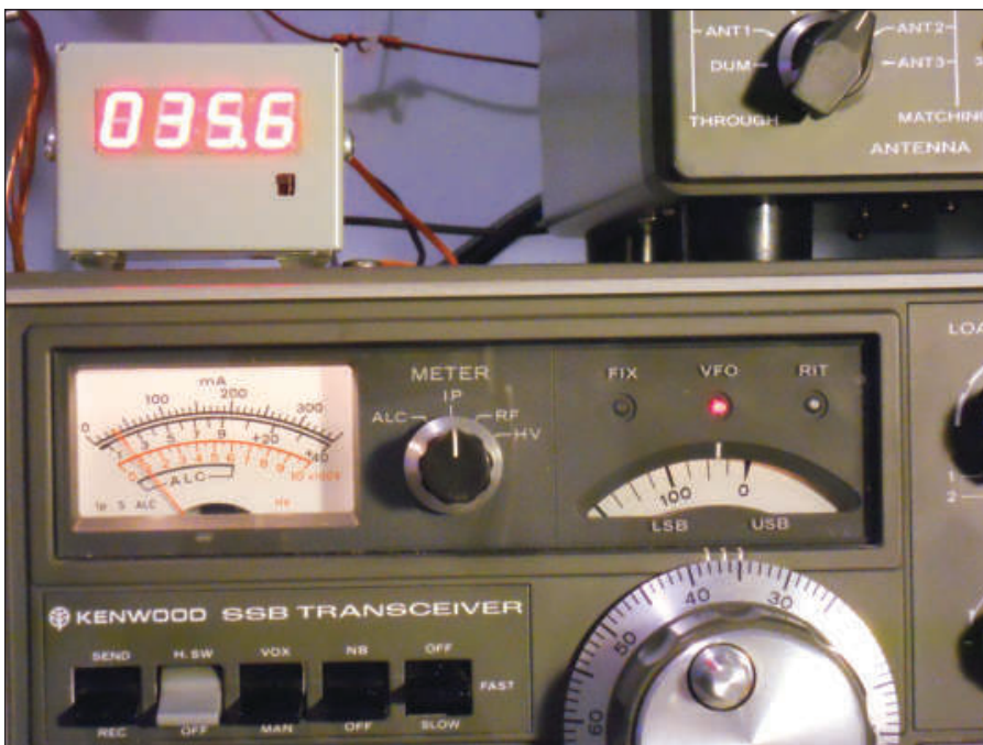
Figure 1 — The digital dial on top of my TS-520S transceiver. The analog dial shows .036 MHz. The digital dial gives a more precise .0356 MHz. Adding this to the BAND switch frequency gives the operating frequency.
