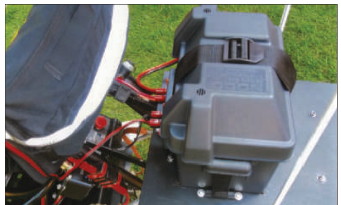
The battery is housed in a commercial enclosure with PowerPole connections.
