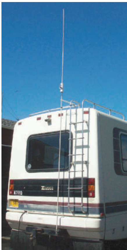
A variometer resonates the 75 meter band vertical antenna mounted on my mobile home.
