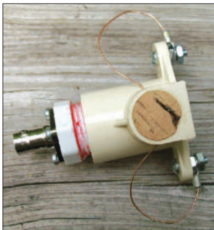
Figure 4 — The assembled center section for the dipole. [Ron Davis, WB5TGF, photo]
