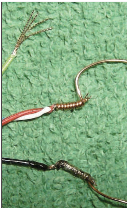
Figure 1 — Coil solid copper wire around the tinsel (red lead) then trim and tin the coil (black lead). The remaining solid wire pigtail can be trimmed off or used to make connections. [Frank Ingle, KG4CQK, photo]
