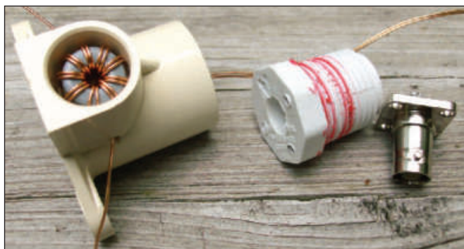
Figure 2 — A PVC shower fixture, a PVC plug, a balun and BNC receptacle make up the dipole center support. [Ron Davis, WB5TGF, photo]
