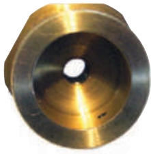
Figure 3 — Detail of the inside of a brass end fitting.
