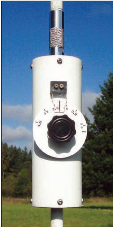
Figure 4 — An outer sleeve protects the completed variometer. You can also see my calibrated tuning knob.
