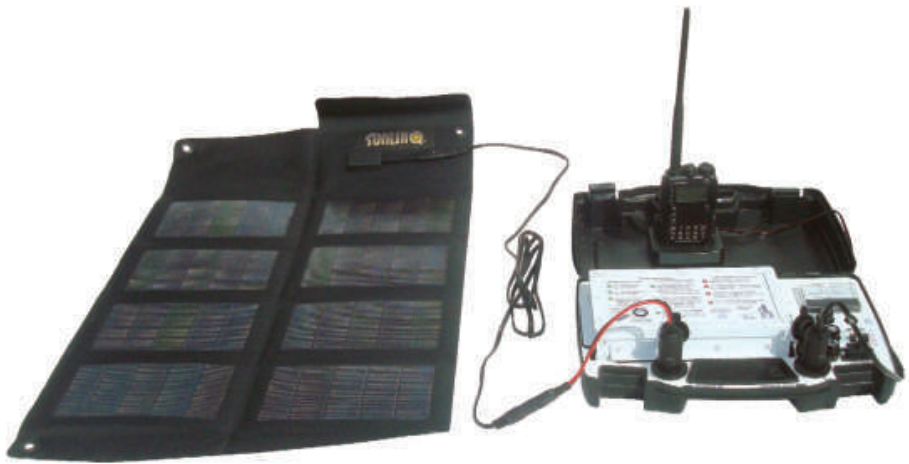
Figure 5 — The solar power system designed by the students. The solar panel is deployed and the system is charging the author's VX-8DR handheld transceiver.
