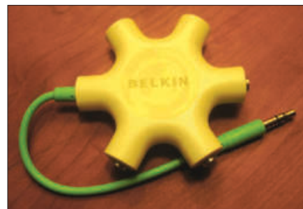
Figure 7 — The Belkin RockStar splitter is an inexpensive and neat method for connecting multiple accessories in your shack. [Bob Mayo, W2TAC, photo]
