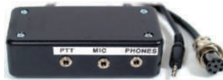
Figure 6 — The front of the completed computer microphone/headset adapter box. I added press-on labels for all the jacks later.
