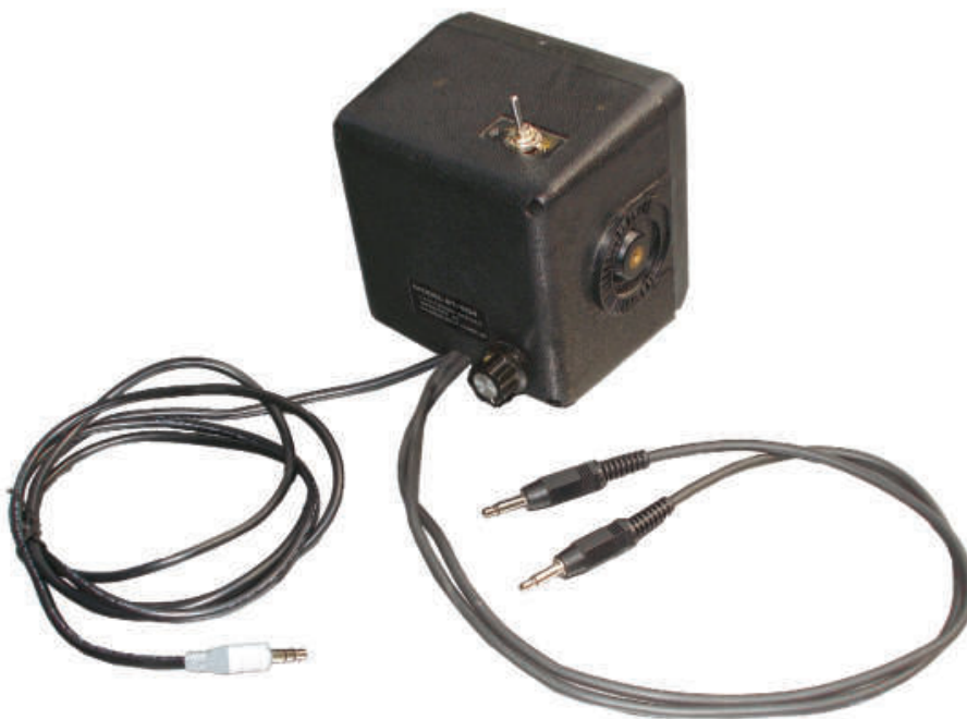
Figure 4 — The completed speaker with the volume control, on-off switch, and cables for connection to the radios and vehicle audio system (white connector). [Ward Silver, N0AX photo]
