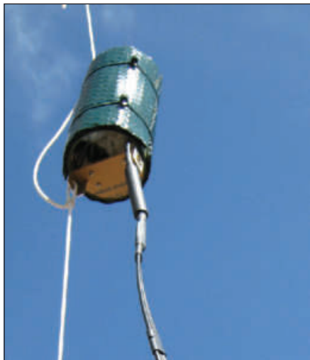
Figure 1 — Bubble wrap painted black encloses the video beacon package, and a J-pole antenna trails below. [Gary Miller, K7GGG, photo]
