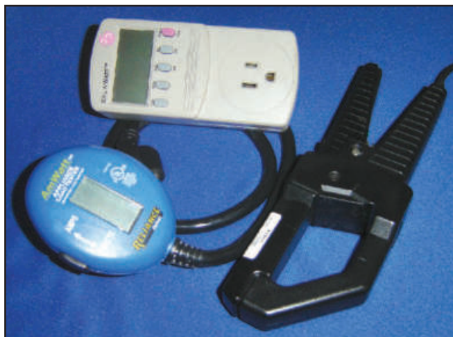
Figure 1 — These can help determine power requirements. Shown are an AmWatt™ Appliance Load Tester (bottom left), Kill A Watt (top) and clamp-on ammeter (right). [Bob Allison, WB1GCM, photo]
