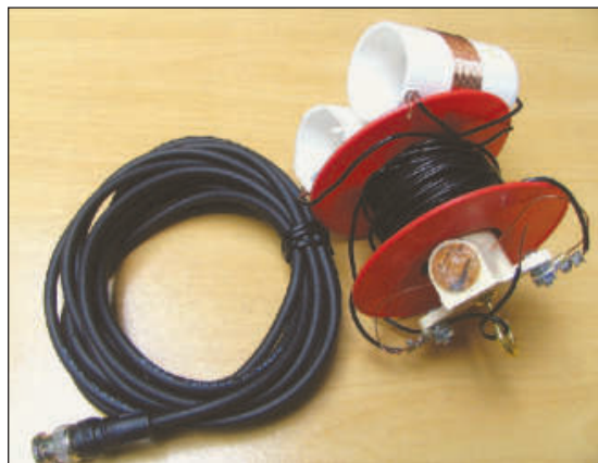
Figure 6 — My emergency 40 meter band grab-and-go antenna system. [Ron Davis, WB5TGF, photo]
