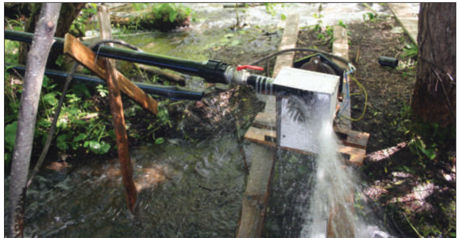
Figure 4 — The hydro generator at work. Since the water flows all the time, no batteries were required.
