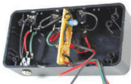
Figure 5 — The RadioShack circuit board fits neatly inside a small project box (RadioShack 270-1802). Here you can see the jack for the radio audio input, and the wiring straight through to the headphone jack. You can also see the back side of the microphone and PTT jacks. The 5 wires go to a microphone plug wired to match my radio.
