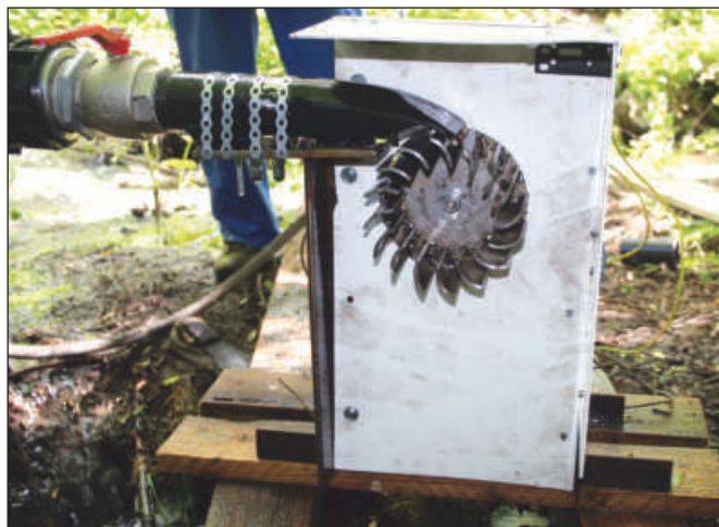
Figure 2 — A close up view of the hydropower generator the students designed to power their portable station.
