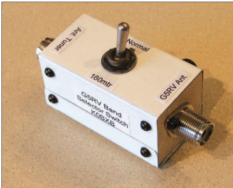
Figure 2 — Completed G5RV switch box.
