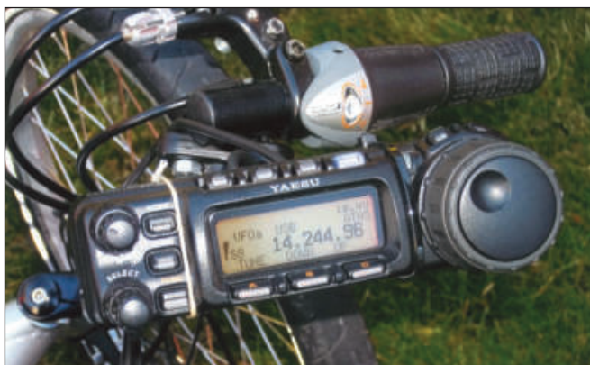
The control head of the Yaesu FT-857D transceiver attached to the right handlebar.
