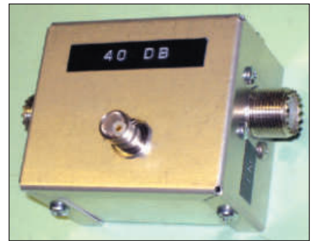
Figure 3 — The sampler uses a BNC connector for the 40 dB port and UHF connectors for the high power RF ports.
