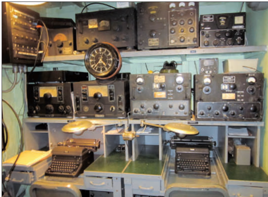
Figure 1 — Mills occupy prominent positions at the two local operating positions aboard the museum ship USS Slater . [Stan Levandowski, WB2LQF, photo]
