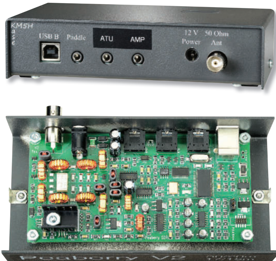
Figure 2 — The compact Peaberry V2 PC board makes extensive use of surface mount components.
