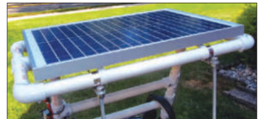
The trike's 20 W polycrystalline solar panel.
