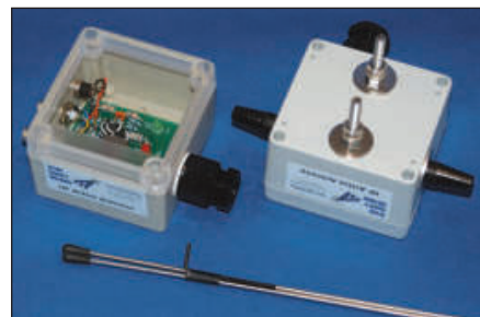
Figure 2 — The active antenna designed to provide calibrated signal strengths when used with the Sentinel SDR receiver for the noise campaign. [Chris Moulding, G4HYG, photo]
