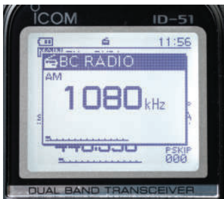
Figure 2 — The built-in broadcast band radio is a plus for public service operators who need to keep an ear on local news updates.
