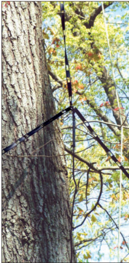
Figure 4 — Close up of the feed arrangement for the prototype ground plane. The six ferrite beads that make the common mode choke are shown below the feed point. A permanent antenna would do better with more structural integrity at the feed. The rope adjacent to the antenna is the halyard for a different antenna.
