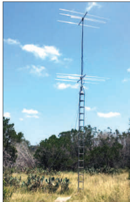
The AB5EB three-element 6 meter OWL Yagi array. [Mike Crownover, AB5EB, photo]
