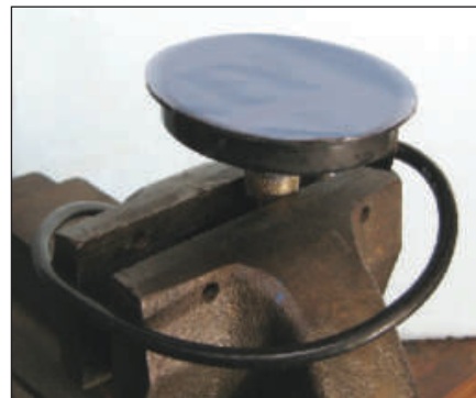
Figure 4 — An old bumper sticker, cut and trimmed to fit, protects your car's roof against scratches from your mag-mount antenna. [Phil Grant, N1YPS, photo]
