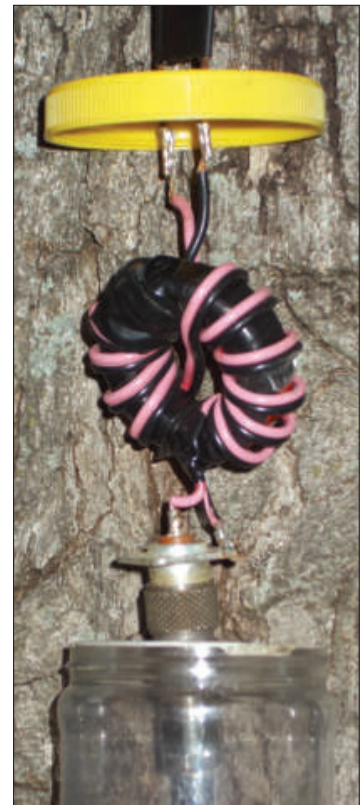
Figure 4 — A version of the balun with the crossover winding. Notice how the input and output connections are in line with the feed lines.
