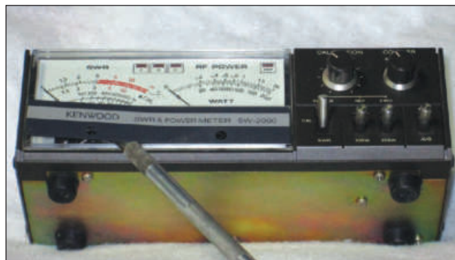
Figure 2 — Removing the name plate.
