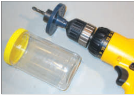
Figure 2 — Use a hole saw, chassis punch, or hobby knife to cut a hole in the bottom of the jar large enough for a PL-259 to go through. Use an awl or small drill to make two holes in the lid for the ladder line conductors. Drill small holes around the bottom of the jar for drainage.
