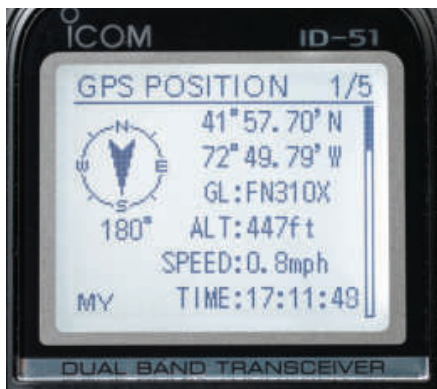
Figure 3 — The ID-51A features a built-in GPS receiver. The receiver is used to determine which D-STAR repeaters are closest to you. The transceiver can also use the GPS receiver to track your position and share the information over the network.
