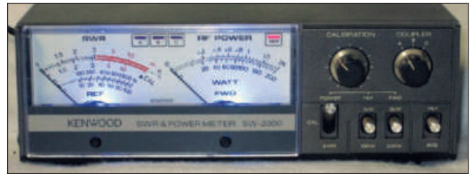
Figure 6 — The meter faces are now illuminated by long-life blue LEDs.
