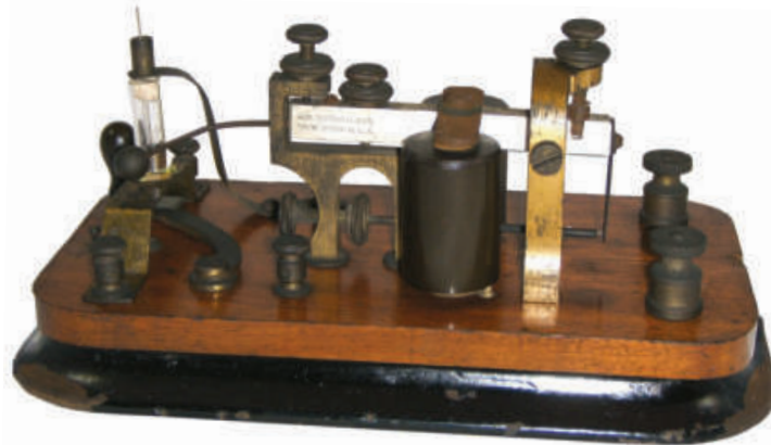
Figure 1 — This side view of the Massie coherer shows the glass tube of the coherer itself on the left and the de-coherer assembly that looks like a telegraph sounder.
