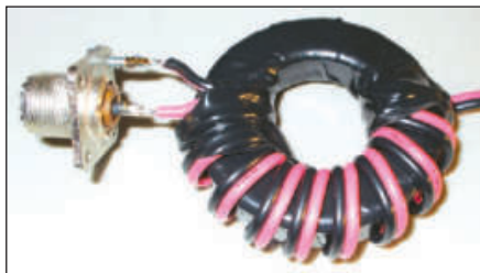
Figure 3 — A close-up of the balun showing the SO-239 connector with winding soldered to the sheet metal screw.
