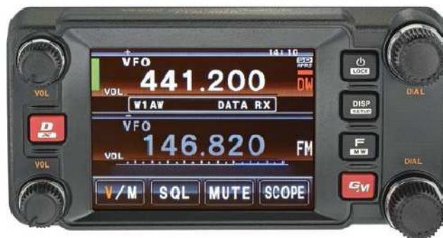
Figure 2 — The FTM-400DR set up for full rate data communication on Band A (top) and analog FM voice on Band B. There are independent volume controls and dial knobs for each band. The functions of the buttons along the bottom of the touchscreen can be changed by the user.
