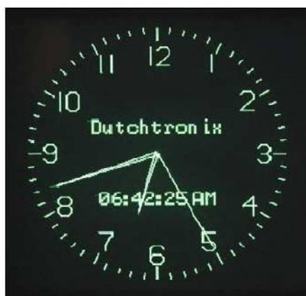
Figure 1 — Oscilloscope clock display generated by Jan de Rie's AVR Oscilloscope Clock available from SparkFun Electronics at www.SparkFun.com .
