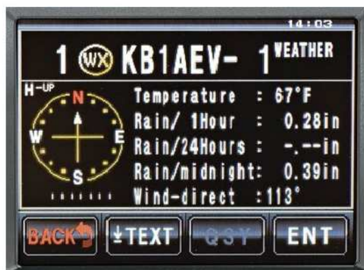
Figure 3 — The FTM-400DR receiving weather information via APRS.
