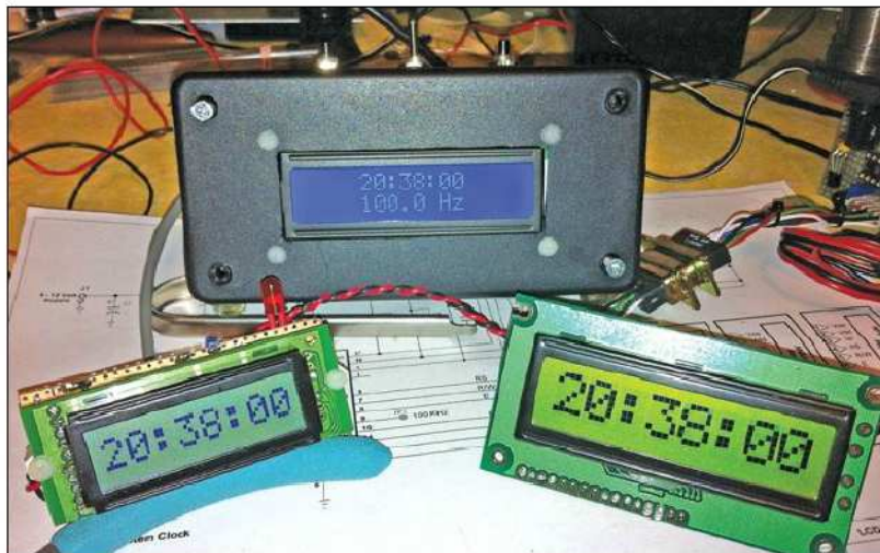
Figure 3 — Three different LCD module display options are available. [Billy Dollarhide, W5ET, photo]
