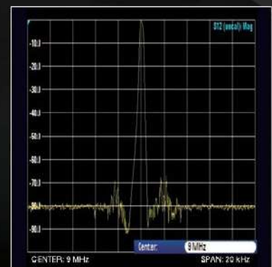
Characteristics of the Crystal Roofing Filter (300 Hz)
