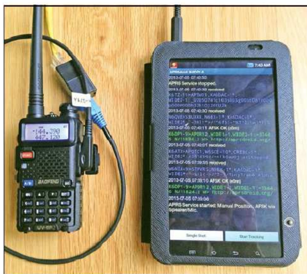
Figure 1 — The Baofeng UV-5R radio and Samsung Galaxy Tab Wi-Fi connected by cable with APRSdroid in action. [Daniel Yang, K6DPY, photo]
