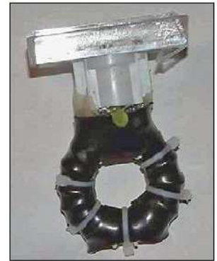
Figure 3 — A toroidal transformer (Mix 2 powdered-iron — T157-2 core) samples RF current, which is then rectified and displayed on a sensitive current meter.
