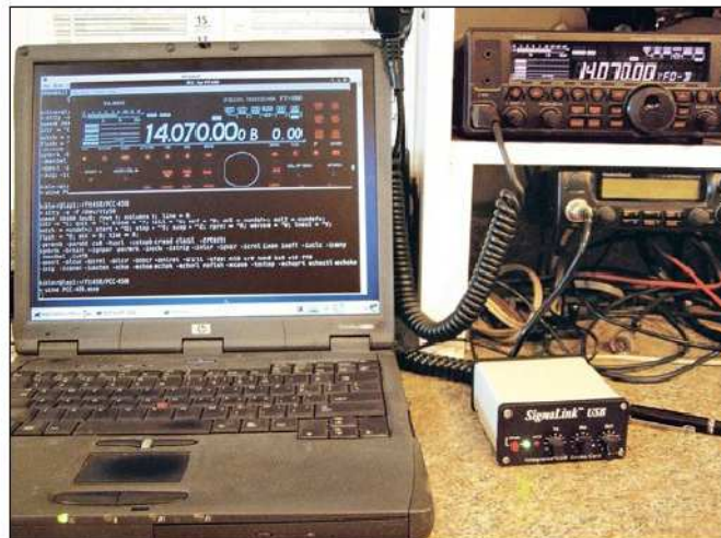
An old HP laptop using Linux Wine , a Windows emulator that is being used to run Windows Yaesu PCC-450 software, which in turn is communicating serially with an FT-450 transceiver and a SignalLink USB interface. All units are powered by two solar collectors and three solar batteries.
