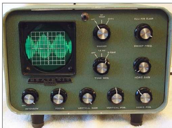
Figure 7 — Repurposed SB-610 with solid state CRT drive — oscilloscope mode.
