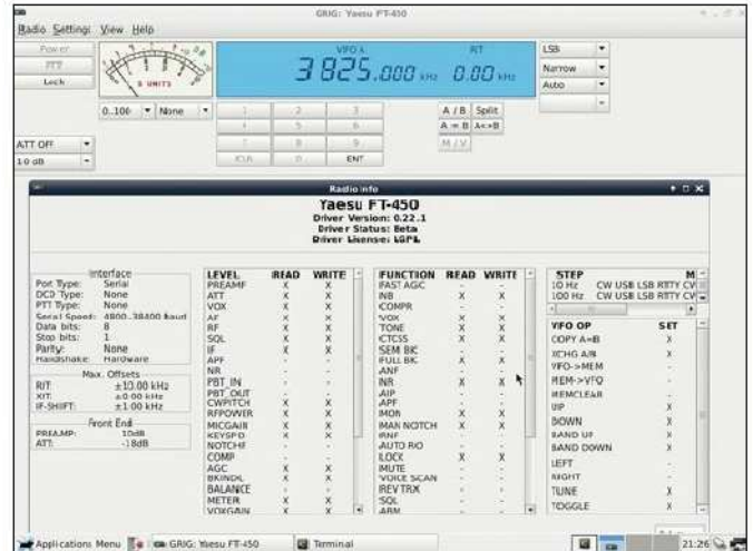
Grig Linux software controlling a Yaesu FT-450 transceiver.
