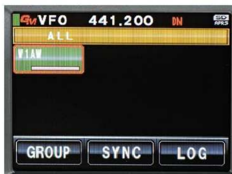
Figure 4 — In the Group Monitor mode, call signs of stations in range (W1AW) are highlighted in green.
