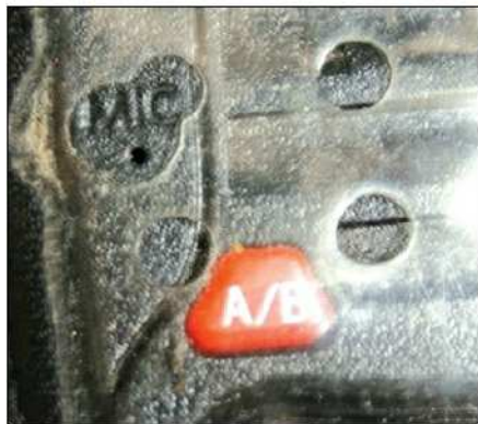
Figure 4 — Punching a “mic hole” in your handheld transceiver’s protective vinyl cover may solve that low audio problem. [Hal Rogers, K8CMD, photo]
