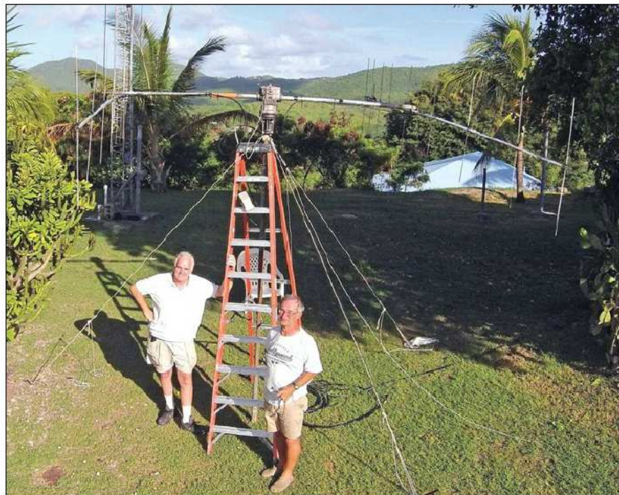
Figure 2 — Pete Rimmel, N8PR (left), and Bill Dzurilla, NZ5N, standing beside their two nine-element M 2 2 meter antennas mounted on an az-el rotator. [Mark Wohlschlegel, WC3W, photo]
