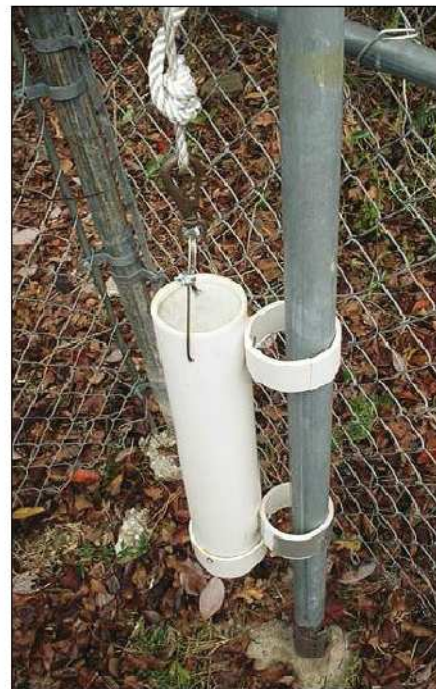
Figure 5 — A section of plastic pipe can be cut and glued to form an antenna counterweight, which is then attached to a section of mast to keep it under control. [Patrick Hamel, W5THT, photo]
