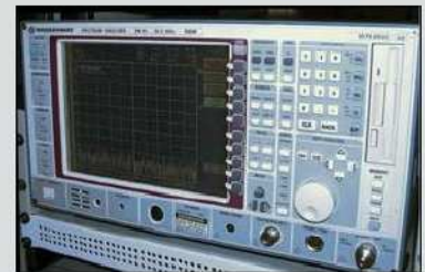
This Rohde & Schwarz FSEM spectrum analyzer can measure radio frequencies from 20 Hz to 26.5 GHz.
