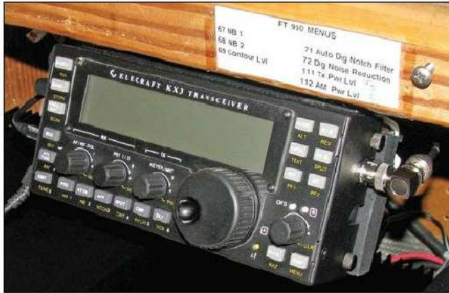
Figure 5 — The KX3, mounted to an under-shelf bracket, makes an excellent backup transceiver or primary rig for a “space challenged” shack. [Mike Lichtman, KF6KXG, photo]
