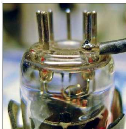
Figure 3 — Connect the varicap diode through C8 directly to Pin 7 (cathode) of V301.
