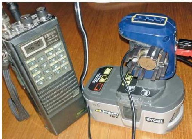
Figure 2 — An accessory battery tester is modified with the addition of a regulator and Powerpole connectors to convert electric tool battery packs for use with portable radios. [Wally Gardiner, VE6BGL, photo]
