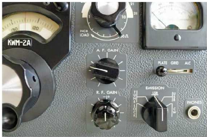
The new RIT function control is stacked with the RF Gain control.
