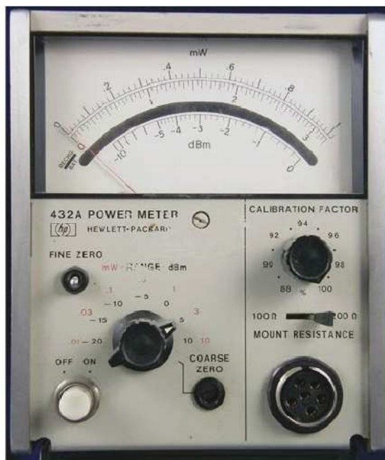
Figure 1 — Analog power meter with both power and dB scales. [Paul Wade, W1GHZ, photo]
