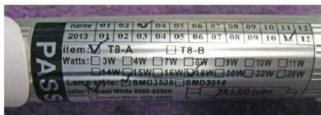
Figure 1 — The product label for one of the noisy lamps. [Andy Corbin, W4KDN, photo]
