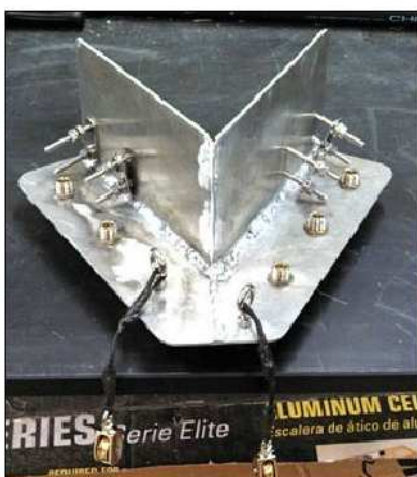
Figure 6 — The coax connector plate made from aluminum plates welded together at a 60° angle. [Dennis Klipa, N8ERF, photo]
