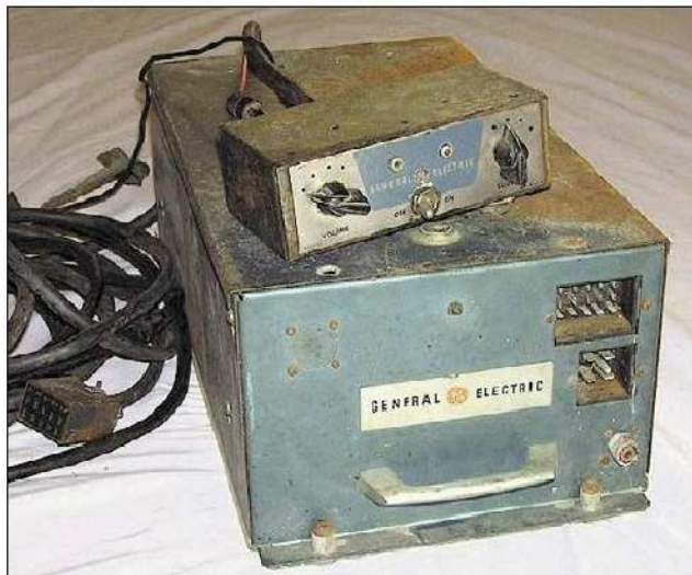
Knowledgeable hams turned surplus FM rigs like these into amateur FM transceivers.
