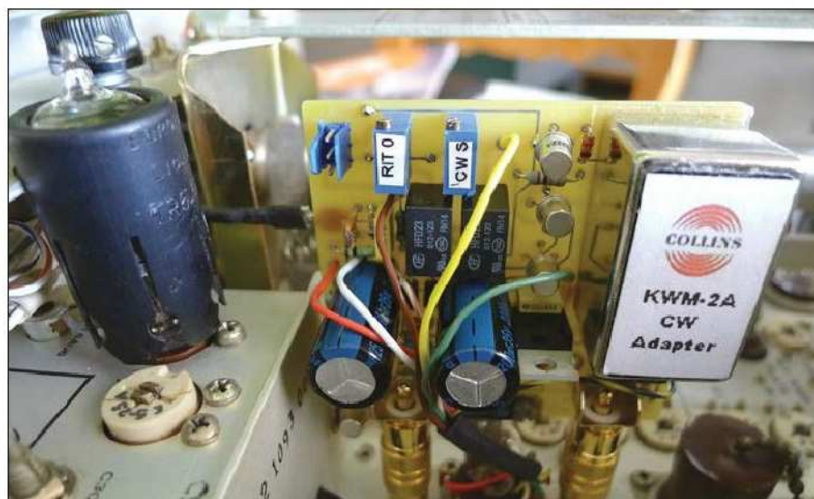
Figure 1 — The CW adapter plugs into the KWM-2A.
