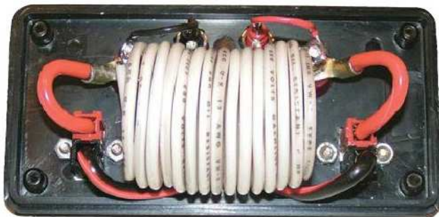
Figure 2 — The resistor is made from a 6-foot length of 12 AWG copper wire formed into a multiturn coil having an inside diameter of 1\frac{1}{4} inches. [David Warner, W7SZS, photo]
