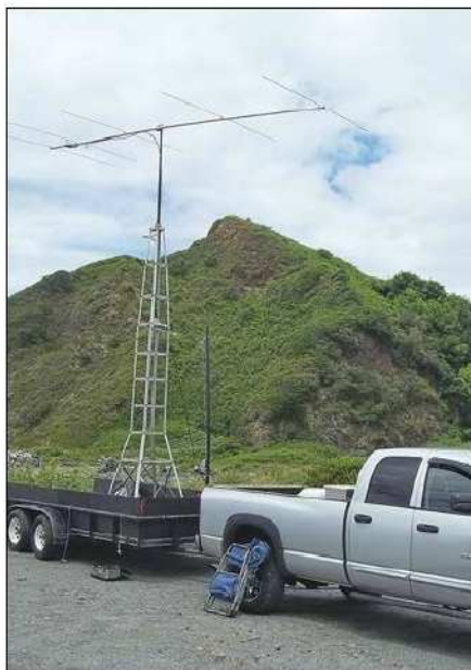
Figure 2 — Charlie's, K6CS, 16 foot car trailer together with his tower and beam. [Charlie Swim, K6CS, photo]
