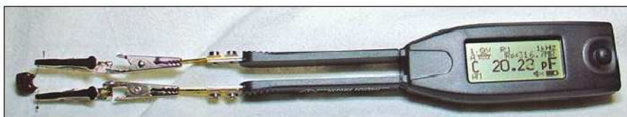
Figure 11 — The author's leaded component adapter.
