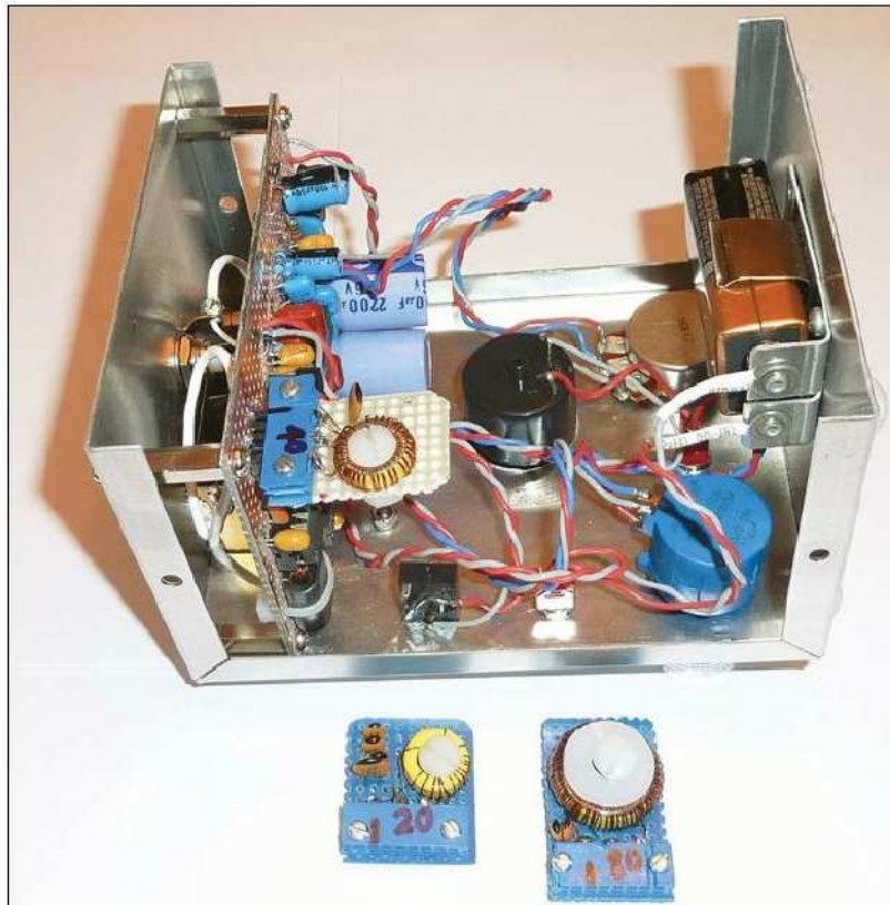
Figure 7 — Noise receiver inside view. The two modules are plug-in coils for 20 and 80 meters.
