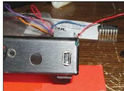
Figure 5 — Cutout on the KPC-3 back panel for the USB connector.
