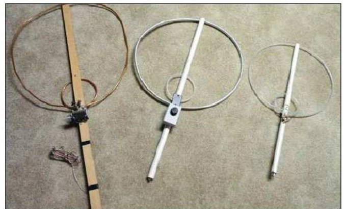
Figure 2 — Tracking loop antennas. Left to right: 24-inch copper loop, 20-inch aluminum loop, 16-inch #22 AWG wire loop with plastic tubing.
