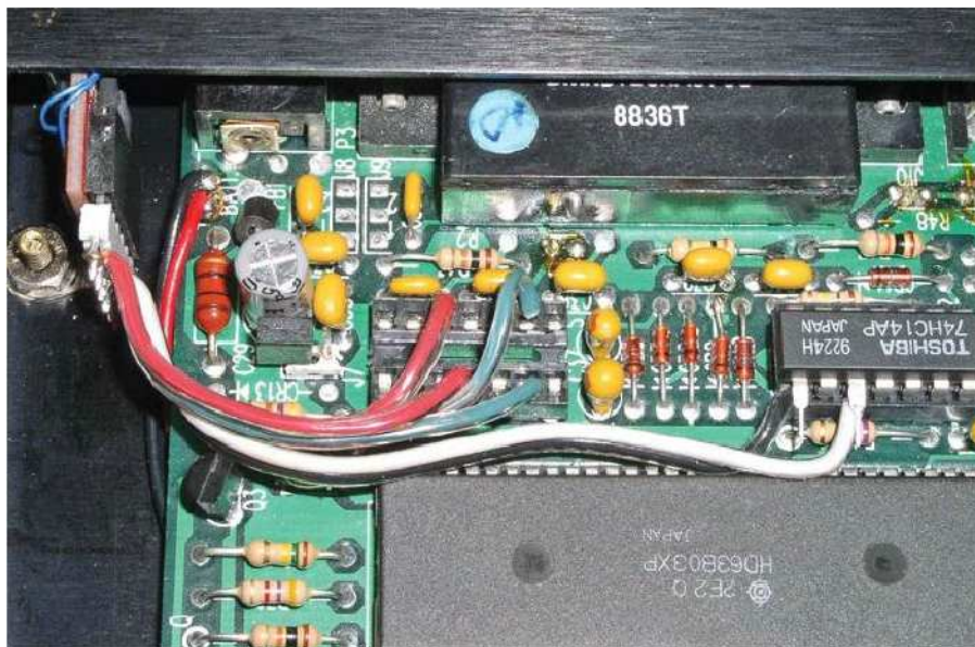
Figure 7 — Completed modification with solid conductor wires routed from the SparkFun board to U1 and U2 IC sockets.
