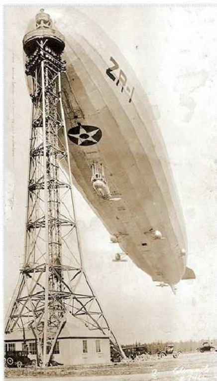
The USS Shenandoah was the first airship to be filled with expensive and rare helium; this was considered safer than the highly flammable hydrogen that had been used previously.
