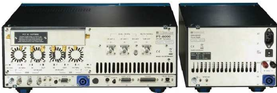
Figure 2 — The Hilberling PT-8000A rear panel, showing the available connections.
