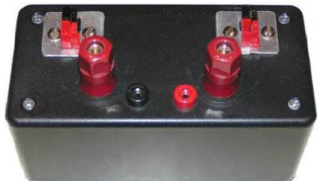
Figure 3 — The current shunt resistor mounted in a small plastic project box. [David Warner, W7SZS, photo]
