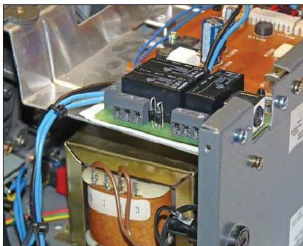
Figure 7 — The completed Rotorcard installed in a Yaesu G-800SA rotator control box.
