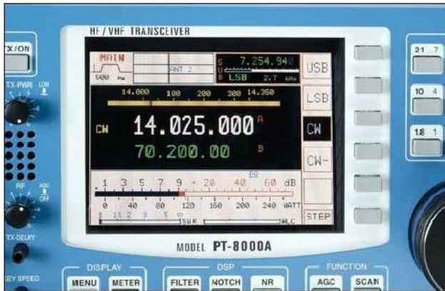
Figure 1 — The PT-8000A's colorful display prominently indicates the main receiver's VFO A and B frequencies, mode and filter bandwidth. The sub receiver frequency, mode and bandwidth are shown in the upper right corner. Metering functions (S meter, transmitter power, ALC, and SWR) are shown along the bottom. Along the right-hand side are soft buttons — button functions change to allow quick access to various settings and menu options.
