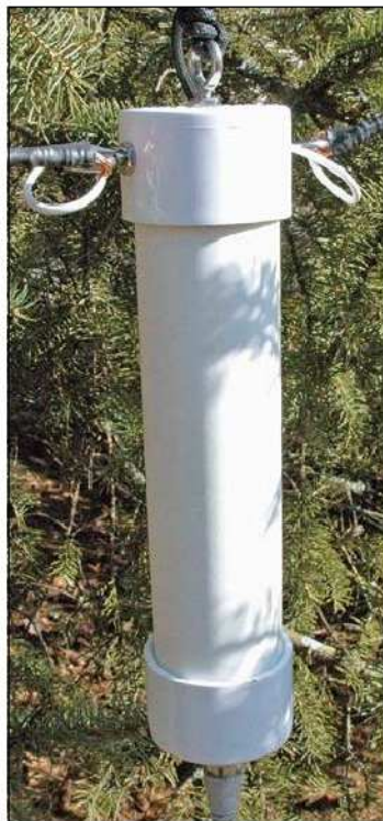
Figure 15 — The matching unit at 28 feet above ground.
