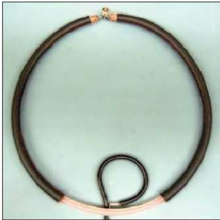
Figure 3 — The concept demonstration antenna that I built. This loop was resonant at 70 MHz. Note the small variable tuning capacitor at the top of the loop and the Faraday link coupling used to feed the loop at the bottom of the loop.
