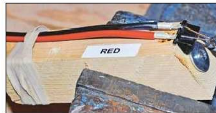
Figure 4 — This simple wooden jig simplifies the soldering of Powerpole connectors. [Dean Sheeley, KG7DKC, photo]
