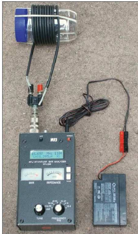
Figure 3 — Using an antenna analyzer to measure the inductance of a coiled-coax choke. The coil is wound around a 3-inch diameter peanut butter jar. The jacket at each end of the cable is stripped back about 1 inch to allow the braid to be made into a lead and connected to the analyzer using a binding post adapter.
