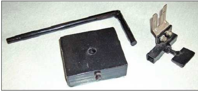
Figure 3 — While this stand is made from steel, wood could be used for simpler construction and a more pleasing look. [Leonard Gordon, KD7CLO, photo]
