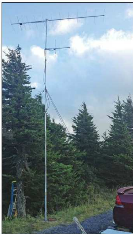
Sam, W8SPM, operated the VHF contest as a low-power portable from Spruce Knob, West Virginia in FM08. He used a Kenwood TR-751A transceiver running 10 W into this single 13LB2 Yagi. [Sam Maze, W8SPM, photo]
