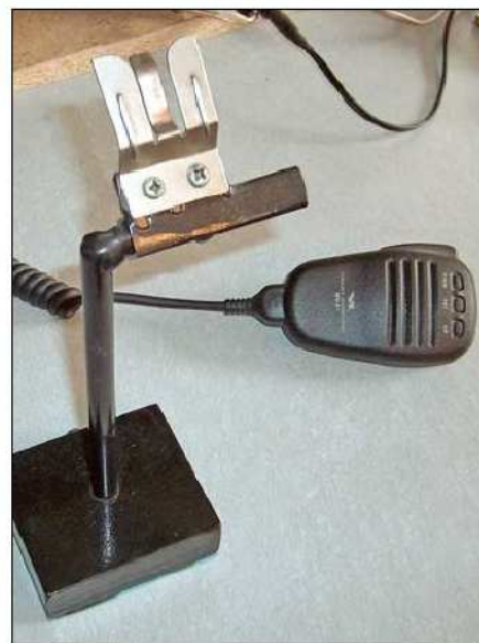
Figure 2 — This homebrewed stand allows the typical factory hand microphone to double as a desk mic. [Leonard Gordon, KD7CLO, photo]
