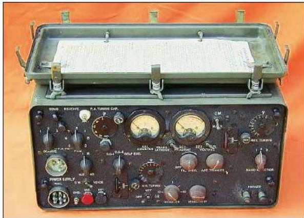
This is the transmitter/receiver part of the TBX-6 radio used by the Code Talkers. The transmitter portion is on the left and the receiver portion on the right. [Antonio Fucci, I8000PU SWL, www.radiomilitari.com , photo]
