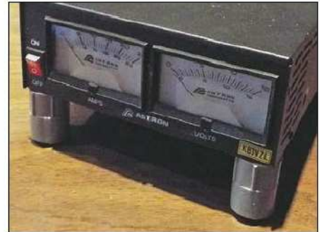
Figure 5 — With the addition of some short "legs," the power supply meters are now much more visible and more cooling air can flow underneath. [Richard Russo, KB3VZL, photo]
