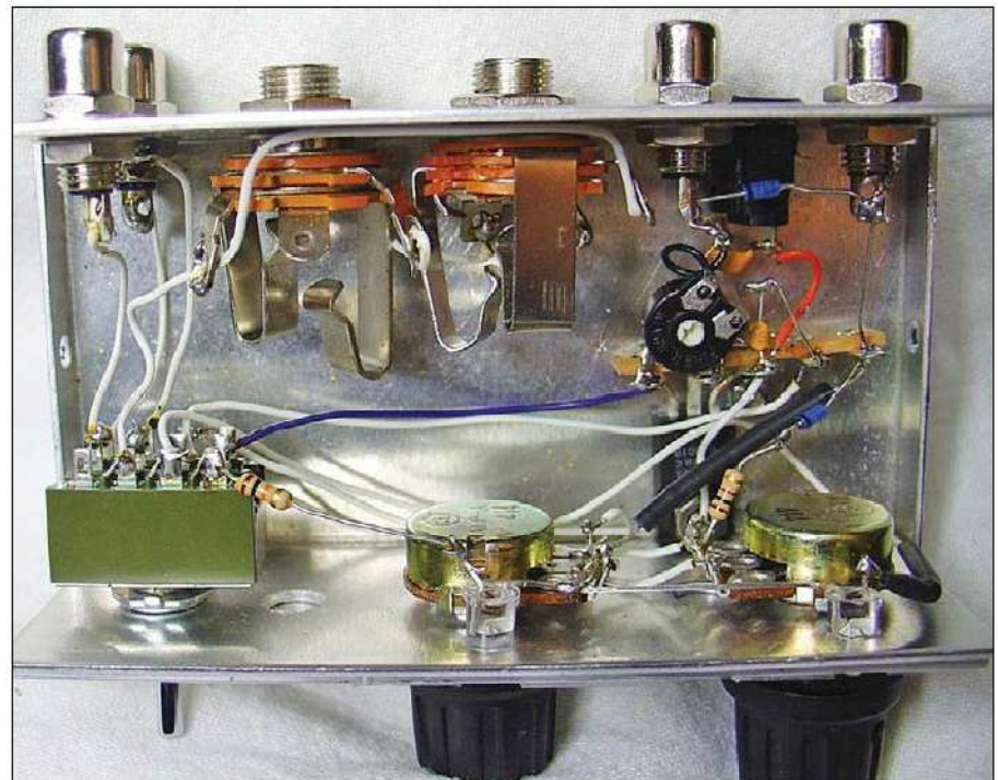
Figure 4 — Interior wiring and components are supported by solder lugs of panel mounted jacks and controls augmented by a five-lug terminal strip to mount the negative voltage regulator and its associated components.
