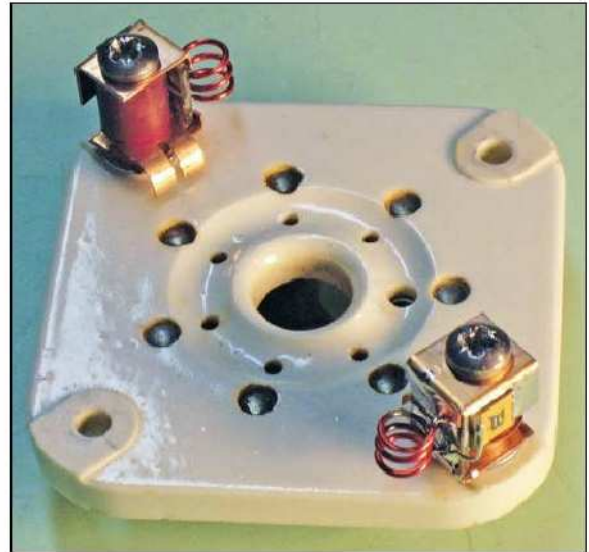
Figure 7 — Modified 8877 tube socket.
