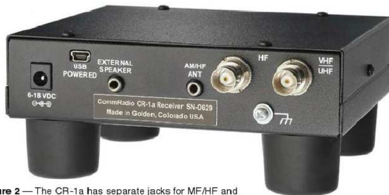
Figure 2 — The CR-1a has separate jacks for MF/HF and VHF/UHF operation. The AM/HF antenna jack is eliminated on current production units. The USB jack can be used to power the receiver and charge the internal Li-ion battery or for connection to an external computer.
