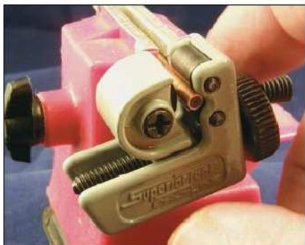
Figure 3 — Start preparing the semi-rigid coax by scoring with a miniature tubing cutter.
