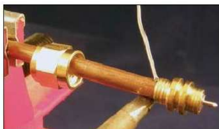
Figure 5 — Solder the SMA connector to the semi-rigid coax. Work as quickly as possible to prevent excess heat from damaging the Teflon dielectric.
