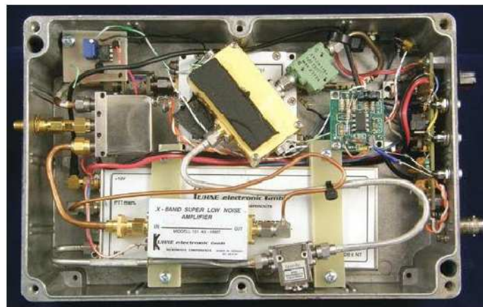
Figure 2 — Bottom view of a modular transverter for 10 GHz. Note the semi-rigid coax and SMA connectors linking the various modules.
