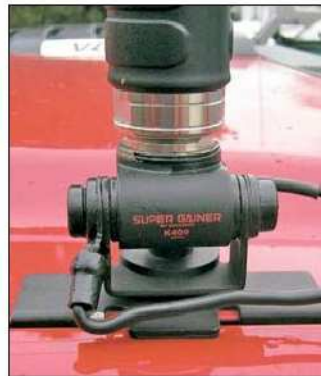
Figure 4 — The thick black ground wire was added when the original VHF antenna was replaced with the ATAS-120A. This functioned well on all bands except 15 meters. [John Wittmann, N1YV, photo]
