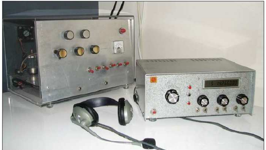
Figure 1 — Hybrid transmitter (left) and VFO/receiver (right). The transmitter knobs upper row (left to right) are Band Selector (optional), and Microphone Level; knobs lower row (left to right) are Load Capacitor, Plate Capacitor, Metering Selector (optional); switches (left to right) are Tone, 12 V, TR, 500 V, 250 V, Power off/on; input jacks are Auxiliary (left), and Microphone (right).
