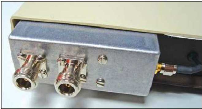
Figure 5 — Master unit bias T mounted on the rear of the case.
