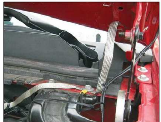
Figure 5 — The black ground wire and additional grounding braids were needed for the ATAS-120A to operate on the HF bands. [John Wittmann, N1YV, photo]
