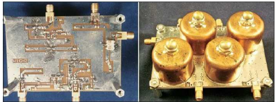
Figure 1 — Top and bottom views of a 3456 MHz transverter that uses pipe-cap filters.
