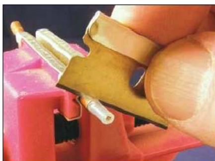
Figure 4 — With the copper jacket removed, trim the Teflon dielectric square with a razor blade.
