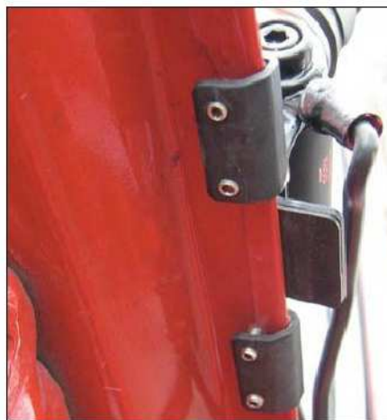
Figure 6 — In addition to all the added ground wiring, the setscrews of the K400 mount must be in contact with bare metal for the ATAS-120A to tune across all the HF bands. [John Wittmann, N1YV, photo]
