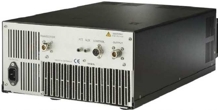
Figure 1 — The HLV-1100 uses Type N connectors for RF input and output, and a phono jack for PTT control. The CONTROL jack allows for remotely mounting the amplifier.
