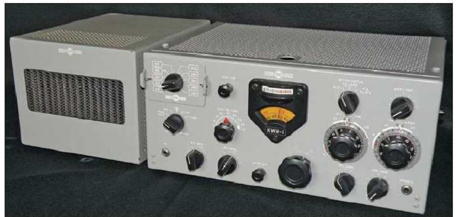
A Collins KWM-1 transceiver with matching speaker/power supply. [Mark Mumaw, NU6X, photo]
