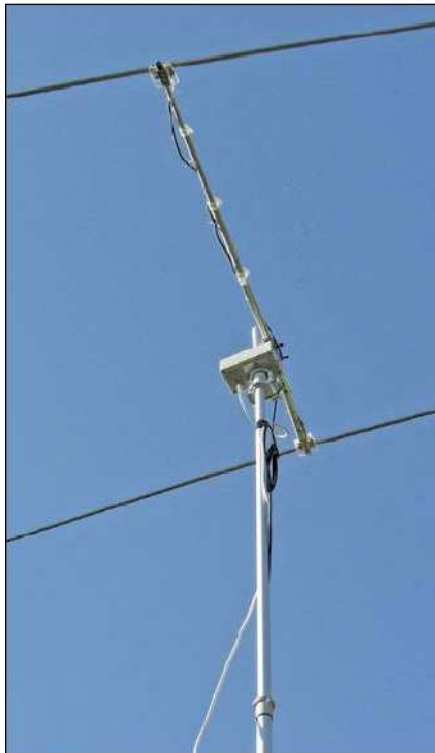
Figure 9 — The 12PR1A rotator installed on a temporary mast with a two-element 6 meter Yagi.
