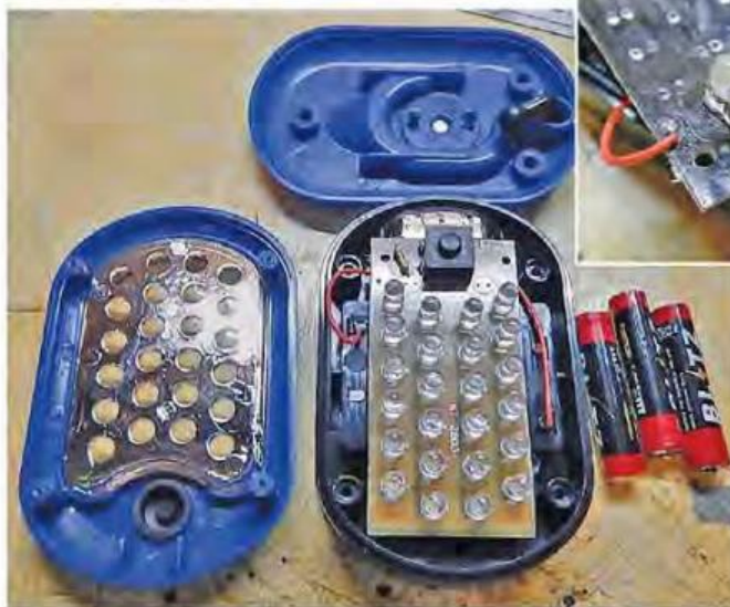
Figure 7 — The disassembled flashlight, ready for modification. [Joe Birsa, N3TTE, photo]
