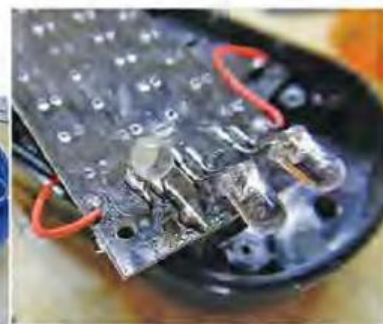
Figure 8 — The LED must be gently pried up in order to jumper from the LED/switch terminal to the other switch terminal using a small soldering iron. [Joe Birsa, N3TTE, photo]
