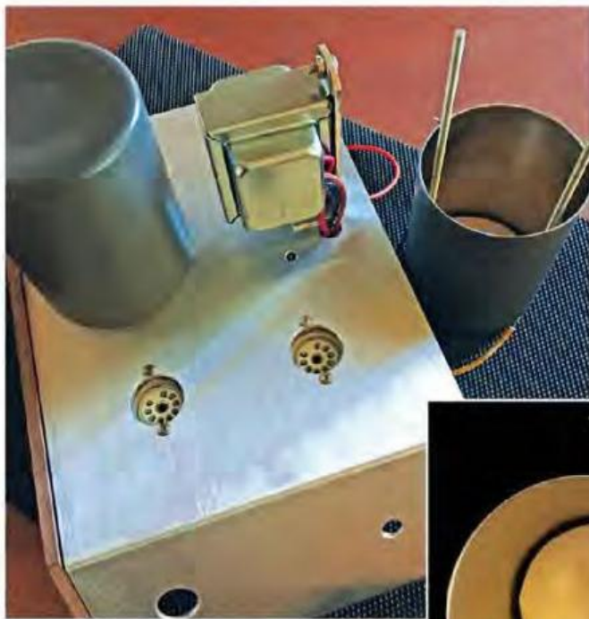
Figure 3 — Transformer covers fashioned from IKEA toothbrush holders. [Barry Shackelford, W6YE, photo]
