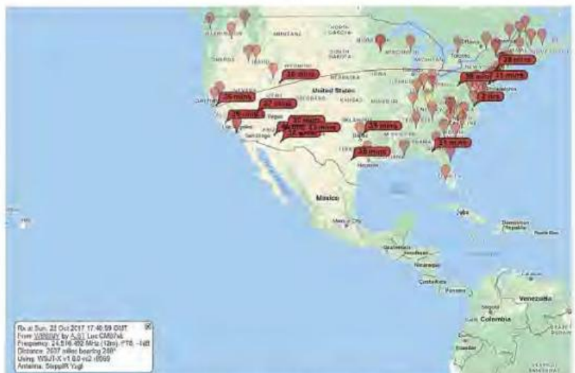
Figure 2 — PSKReporter showing reports of my FT8 transmissions on 12 meters. Notice that AJ6T has given my 20 W signal a nice -1 dB report (his report is visible in the lower left corner), but also notice that his report includes the fact that he is using a SteppIR Yagi antenna.
