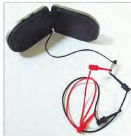
Figure 6 — The battery-powered audio amplifier, with mini grabbers for troubleshooting. [Bill Pellerin, KE5XV, photo]
