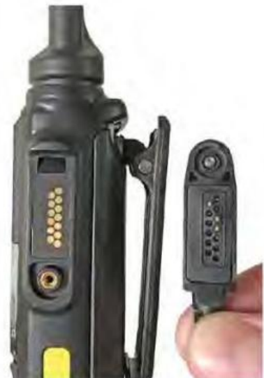
Figure 1 — The TYT MD-2017 speaker/mic connector (programming cable).
