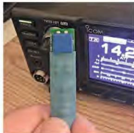
Figure 12 — Click2Tune fits easily in your hand. Just press the blue button and your transceiver will start generating a steady 10 W output.
