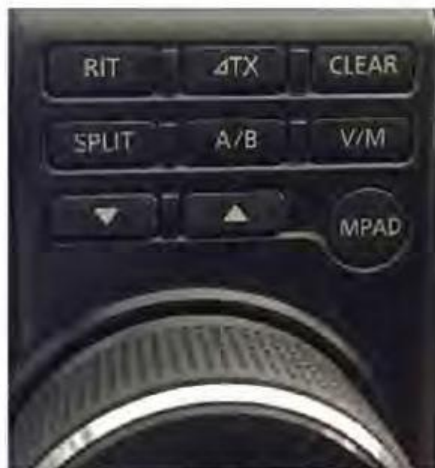
Figure 2 — Switching from one VFO to another is often as simple as pushing a button to toggle between VFO A or B. You can see the A/B button in this photo. Also look for the SPLIT button. This will allow you to transmit on one VFO frequency and receive on another.
