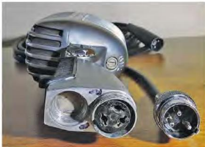
An example of an older Shure 55 with Amphenol 91-MC3 connectors and an "HML" impedance switch on the base of the microphone. [Jeanette Ellis, NP2C, photo]
