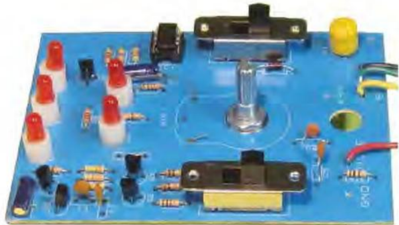
Figure 6 — The assembled board before going into the case. The transistor test LEDs and the OK LED are on the left, and at the right are the two DIODE TEST LEDs. At the upper right is a yellow eight-pin receptacle for small transistors. The transistor base current control is the potentiometer in the middle.
