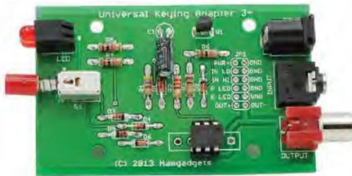
Figure 7 — The completed UKA 3+ PC board. All components, including jacks and switches, mount on the board, so no additional wiring is needed.
