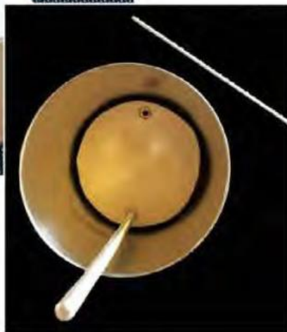
Figure 4 — A cemented plywood disc with threaded brass inserts provides a mounting means. [Barry Shackelford, W6YE, photo]
