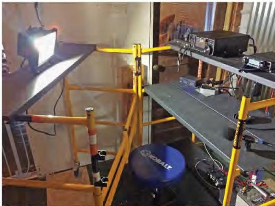
Figure 1 — Mounted Husky 1,000-lumen, 19 W, LED work light illuminates the operating position/platform at K1CE. [Rick Palm, K1CE, photo]
