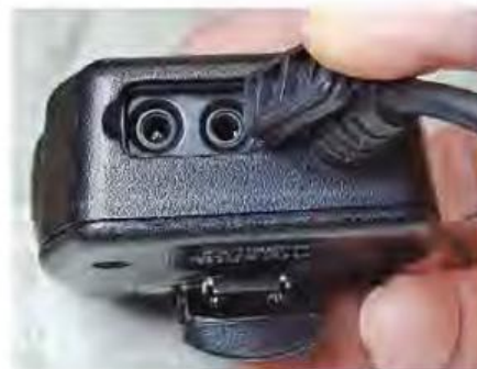
Figure 8 — The charging jack is on the left, and the 3.5-millimeter mono headphone jack is on the right.
