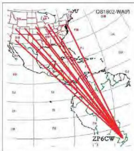
Figure 1 — Sporadic-E trans-equatorial propagation to Paraguay on March 10, 2005.
