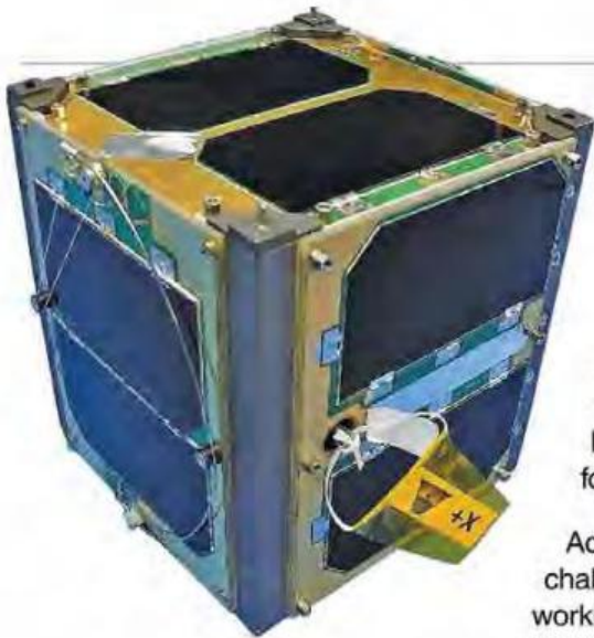
AMSAT-OSCAR 91 is a CubeSat that includes an FM repeater with an uplink on 435.250 MHz (67.0 Hz CTCSS) and a downlink on 145.960 MHz.
