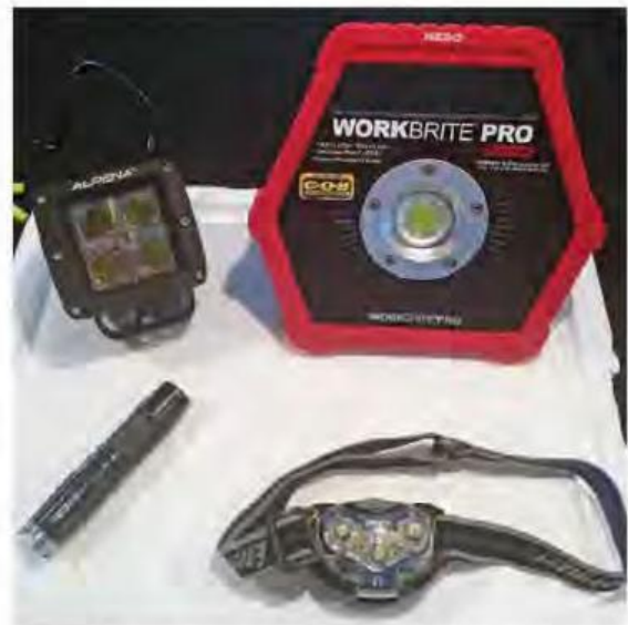
Figure 2 — Solutions for portable station lighting, clockwise: NEBO WORKBRITE PRO 630 lumen LED work light, Energizer 300-lumen LED headlamp, NEBO one AA LED flashlight, and Alpena QuadFire™ 1,400-lumen, 15 W four-LED light. [Rick Palm, K1CE, photo]
