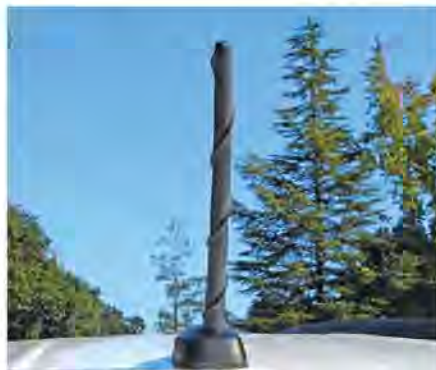
Figure 1 — Small electric field probe mounted on the rear roof of a car.
