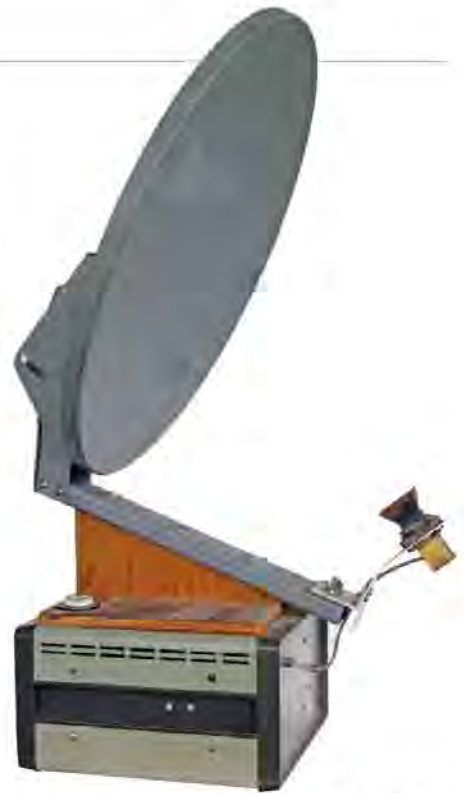
Figure 4 — An offset-fed dish with the dish mounted on top of the transverter for better weight balance. The tilt angle is set by a wooden wedge.
