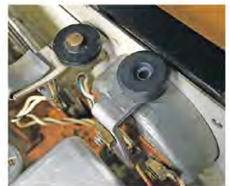
Figure 5 — A small magnet can correct a meter needle that rests above or below zero. [Peter Ravn, OZ8CTH, photo]
