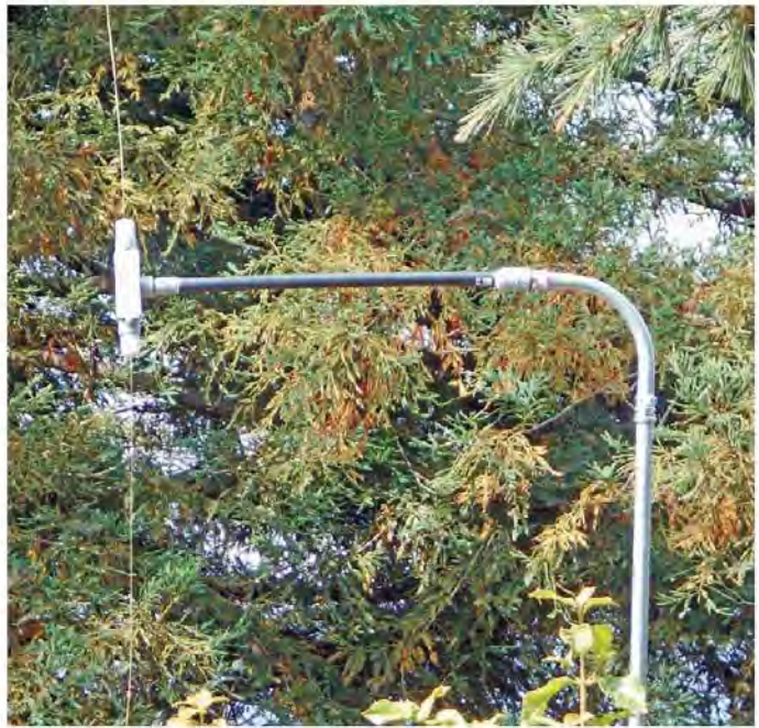
Figure 7 — Active dipole with preamp board inside the PVC T. Shielded CAT5 cable runs down the conduit.
