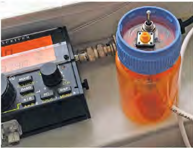
Figure 3 — The control “box,” with DPDT switch on top. [Monty Shultes, K2DLJ, photo]
