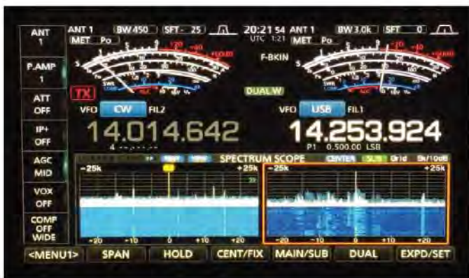
Figure 3 — If the two receiver frequencies are on different bands, or are too far apart to be shown on a single display, the spectrum displays can be separated, as shown here.
