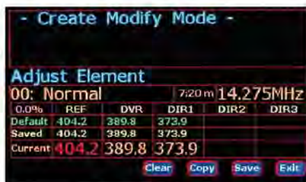
Figure 10 — CREATE/MODIFY screen for a three-element antenna.
