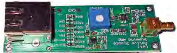
Figure 4 — Preamp board (left) and summing amplifier (right) boards are connected with shielded CAT5 cable.
