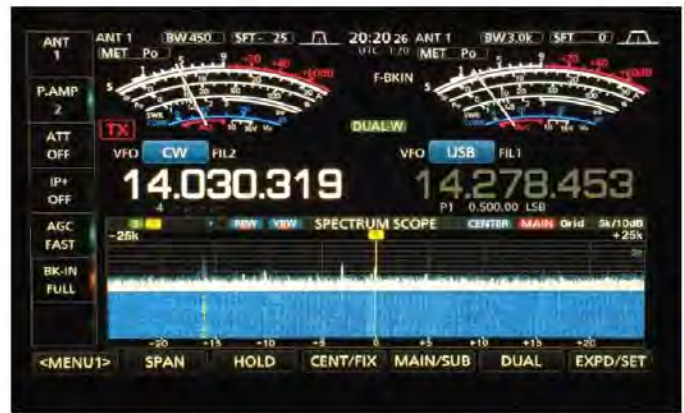
Figure 2 — A waterfall display can be added below the panadapter spectrum display. The waterfall often makes it easier to spot weak signals.
