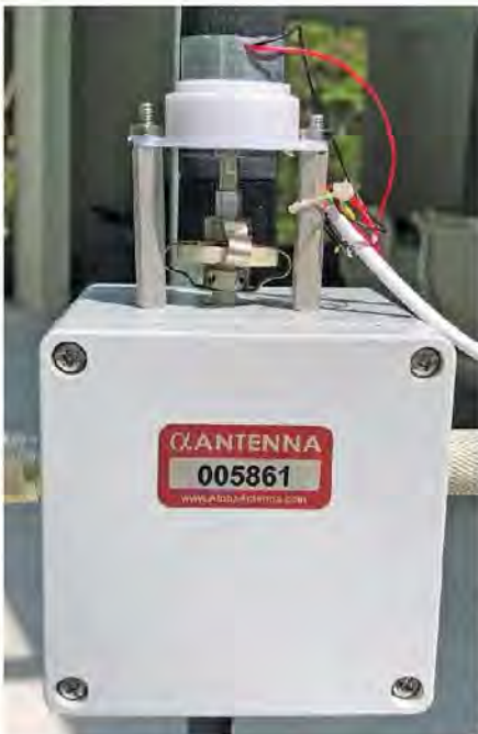
Figure 4 — The completed motor attached to the capacitor box. [Monty Shultes, K2DLJ, photo]
