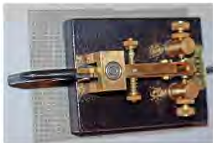
Figure 1 — A CW key placed on non-slip tape designed for rugs stops sliding during sending. [Lionel Booth, N5LB, photo]
