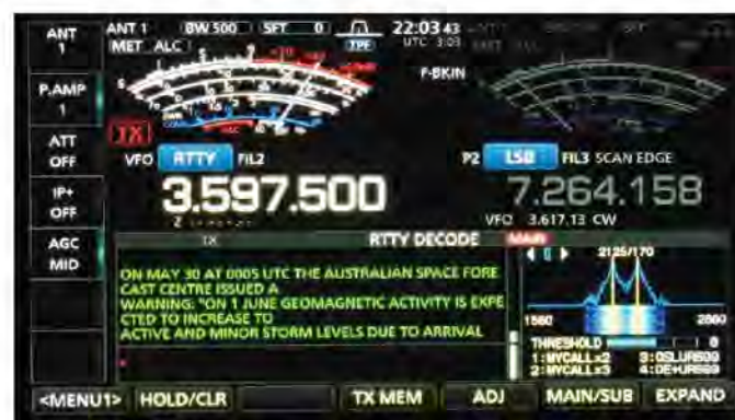
Figure 8 — The IC-7610 decoding the W1AW RTTY propagation bulletin. Note the two-tone tuning indicator and the open panel for use as a type-ahead buffer.
