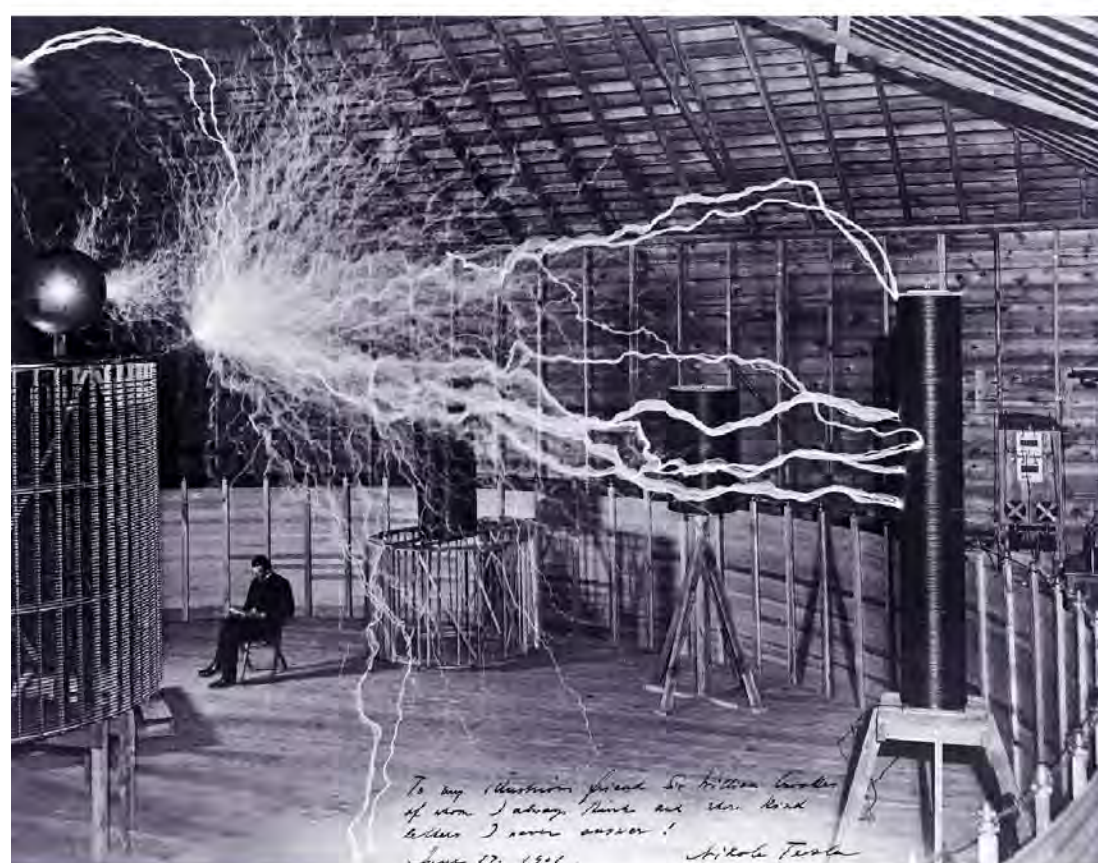
Sparks emitted from Tesla's high-voltage generator at his Colorado Springs lab around 1899. The voltage was exaggerated through double exposure by photographer Dickenson V. Alley. [Dickenson V. Alley, Wellcome Collection gallery, photo]
