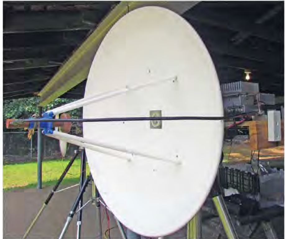
Figure 1 — Fred Stefanik's, N1DPM, prime-focus 10 GHz dish. Note the long feed line from the electronics behind the dish.
