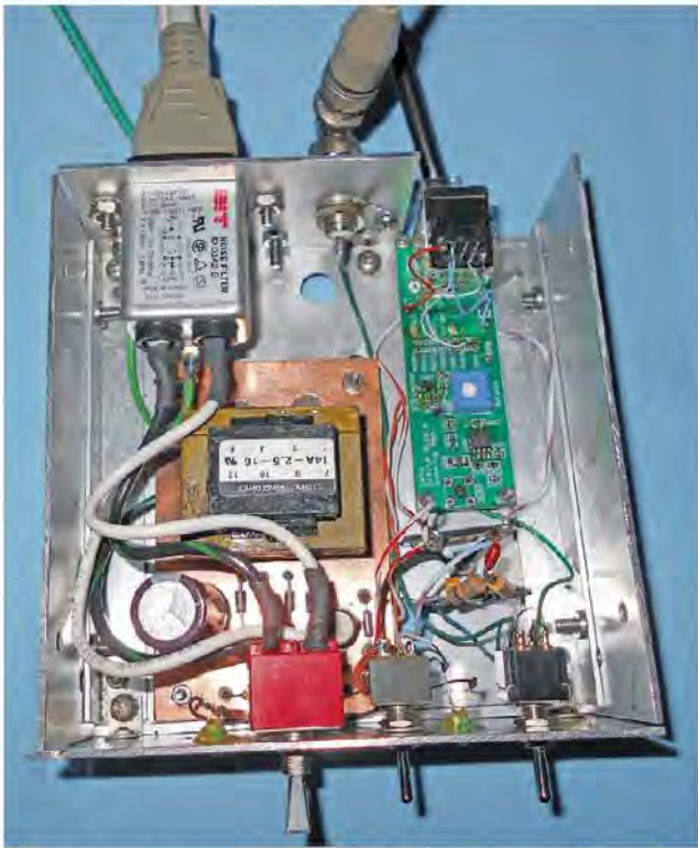
Figure 6 — Summing amplifier mounted in an aluminum box. A small linear power supply is on the left. A 550 kHz low-pass filter is visible below the summing amplifier PC board.
