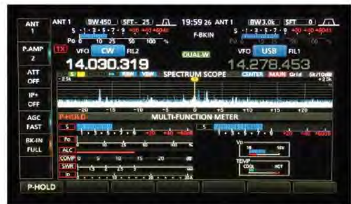
Figure 4 — A more compact bar graph of a selected meter at the top of the display allows more room for the spectrum display, or all meter choices can be viewed simultaneously, as shown here.
