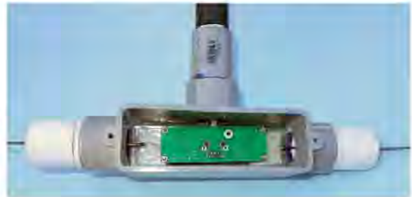
Figure 5 — Preamplifier mounted at the dipole feed point.
