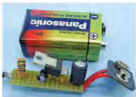
Figure 8 — A comparison of the stripboard power supply to the 9 V battery it's replacing. The stripboard circuit is enclosed in a piece of clear heat-shrink tubing for protection. [Don Dorward, VA3DDN, photo]
