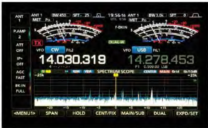
Figure 1 — A close-up of the IC-7610 display showing the virtual analog meters and a single spectrum display.
