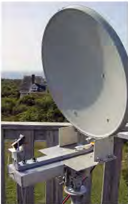
Figure 3 — An offset-fed dish with the transverter mounted under the feed horn. The feed line is short but the weight is not balanced. Note the bubble level at the base of the dish to indicate nominal elevation.
