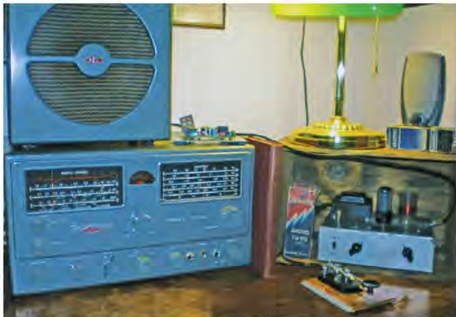
Figure 5 — T/R switch used with an Ameco AC-1 two-tube 15 W CW transmitter and a National NC-98 receiver.
