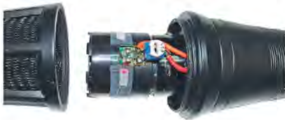
Figure 6 — The gain potentiometer installation. [Paul Dobosz, K8PD, photo]
