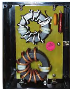
Inside of Matching Unit
