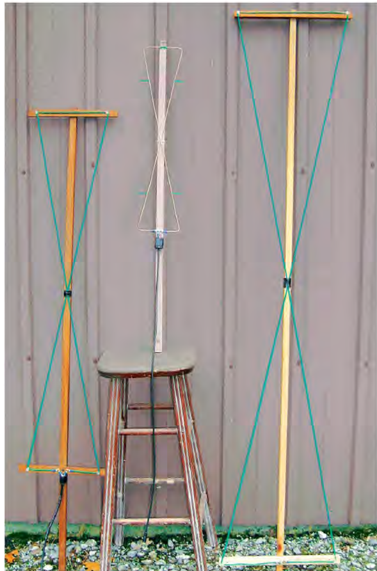
Figure 3 — From left to right, hourglass antennas for 222, 432, and 144 MHz. Only the 432 MHz antenna is made from bare wire.
