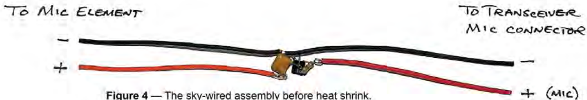
Figure 4 — The sky-wired assembly before heat shrink. [Paul Dobosz, K8PD, photo]
