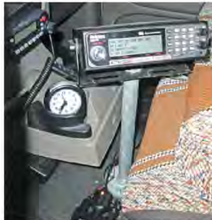
Figure 7 — The finished scanner mobile mount, made from inexpensive plumbing supplies. [Al Wasielewski, WA2VJL, photo]
