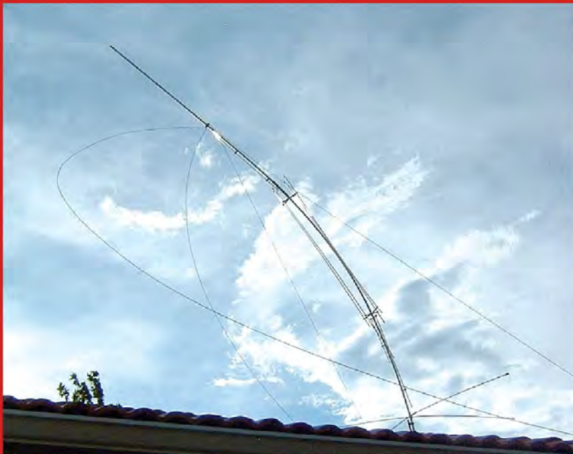
N5CFI also confronted Mother Nature's blustery winds in New Mexico a few years ago and received a valuable education about the importance of antenna guying.
