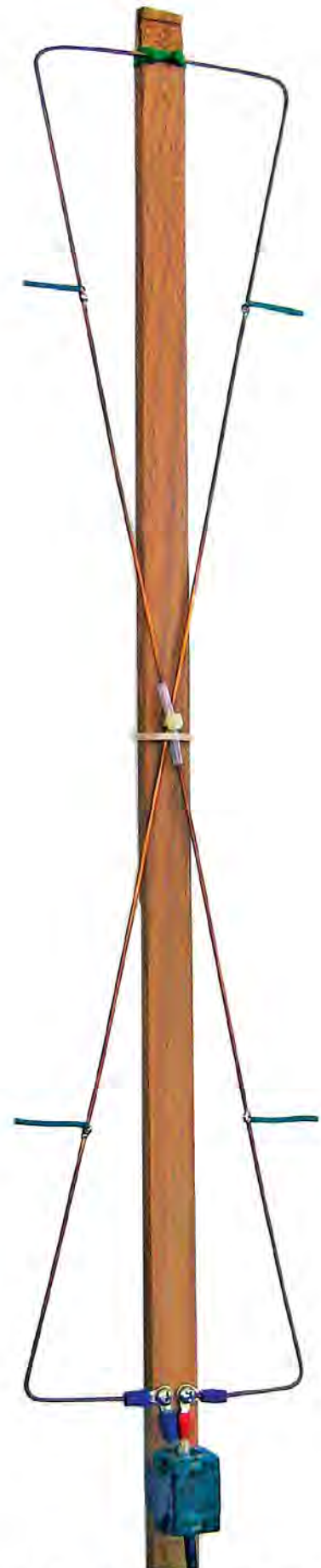
Figure 1 — A 432.2 MHz hourglass made from #14 AWG solid bare copper wire. Note the tuning flags and the clamp-on ferrite around the coaxial feed line and taped to the mast.
