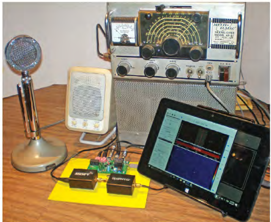
Figure 3 — A 1950s vintage Multi-Elmac AF-67 is paired with an Airspy SDR with the SpyVerter for HF reception.
