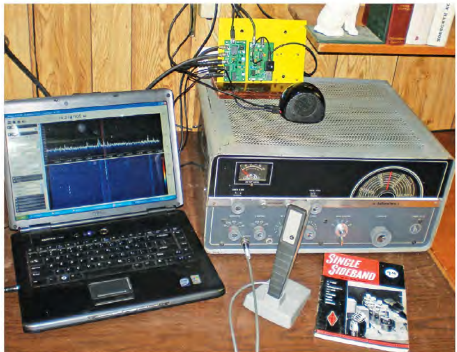
Figure 4 — A simple RTL-SDR is paired up with a Hallicrafters HT-37 transmitter for operation in AM, CW, and SSB modes.
