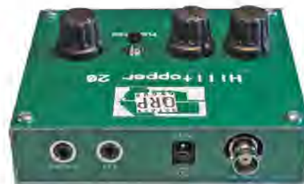
Figure 3 — Key, headphone, power, and antenna jacks are all on the rear panel.
