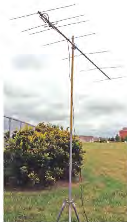
Figure 3 — N0JK's (EM28) portable Yagi used to make contacts on 144 MHz on September 24, 2018.
