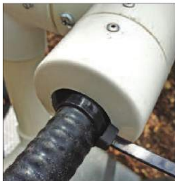
End cap and cable final assembly showing attachment method for waveguide.
