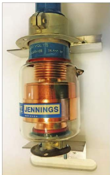
Figure 1 — Jennings 25 – 500 pF variable vacuum capacitor used to tune the loop to resonance.
