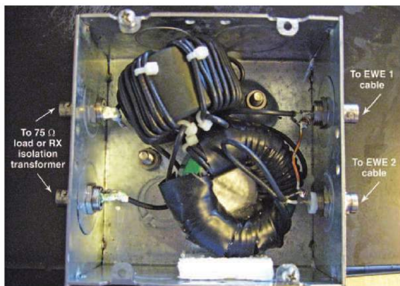
Figure 14 — Photograph of the opposing-phase common-mode choke.
