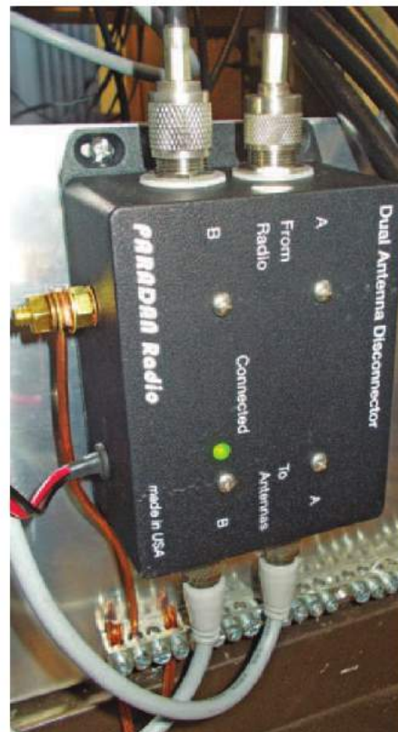
Figure 6 — The Paradan Radio Dual Antenna Disconnecter protection unit installed on a grounded rack panel. Cables at the top connect to the amplifier outputs. Cables at the bottom routed to the nearby 2 × 6 antenna switch are also bonded to the rack. The panel is grounded to the station perimeter ground with a short length of #6 AWG wire.
