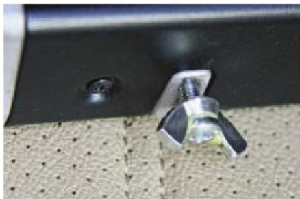
Figure 1 — The wing nut installed for tool-free removal and installation. [Joe Hopkins, K4BKI, photo]
