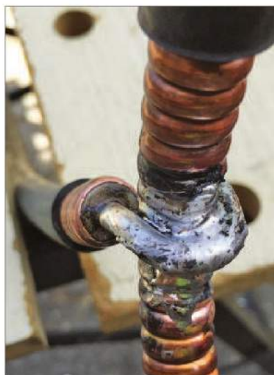
Secondary loop soldering arrangement.
