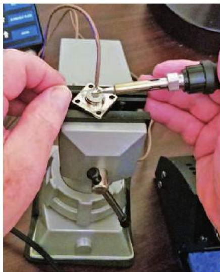
Joe Lynch, N6CL, soldering one end of a VHF loop antenna to the center conductor of a PL-259 coax connector.
