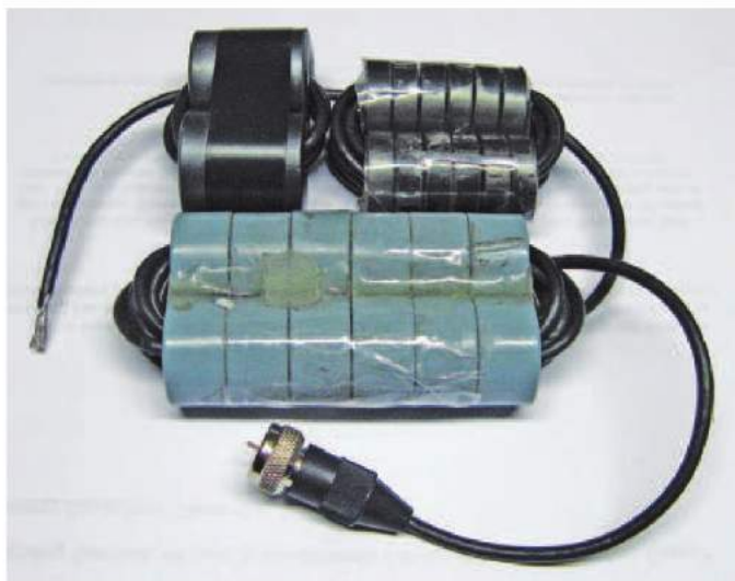
Figure 15 — Photo of the coaxial common-mode choke, used on each antenna termination.
