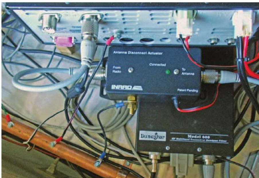
Figure 5 — The single-line INRAD DCA protection unit installed at the back of the reviewer's Kenwood TS-590S transceiver. Power is supplied from the TS-590S antenna tuner connector. Both the radio and disconnect unit are connected to the station ground bus (see text). A more effective location would be at a station's grounded entry point for feed lines with a short connection to the ground system.
