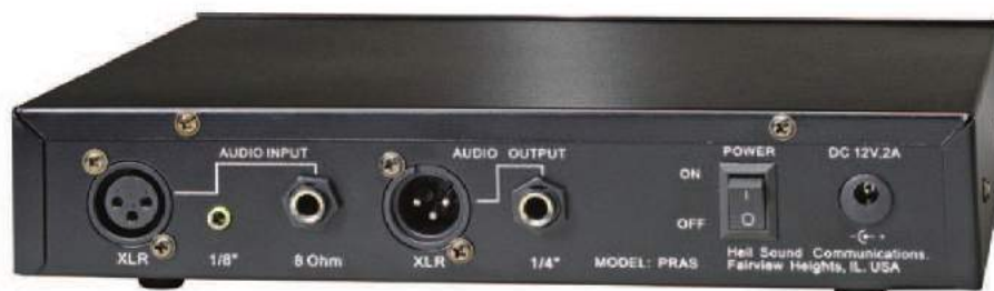
Figure 8 — PRAS rear panel, showing the connections described in the text.
