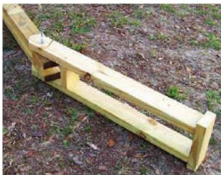
Figure 3 — This wooden fold-over antenna support allows for easy antenna work. [Karl Schwab, KO8S, photo]
