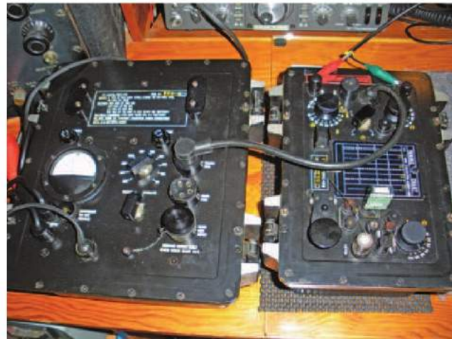
Joe, KA4WJB, made four contacts using this T-784A. This unit (later designated GRC-109) first appeared during the Cold War and was intended for use by CIA agents. Joe said, "The rig even has a built-in key." [Joseph Scoglio, KA4WJB, photo]
