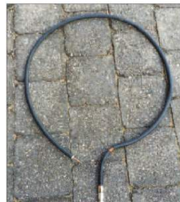
Secondary loop construction. The loop diameter should be 35.43 inches.
