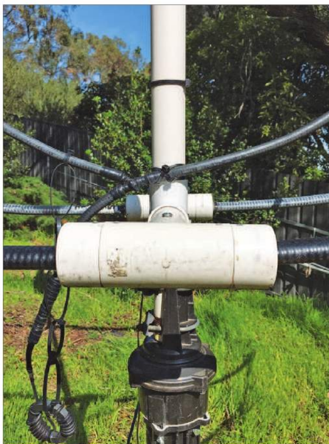
Side view of the secondary loop placement relative to the primary loop element. Start with the secondary loop 4 inches above the main loop.
