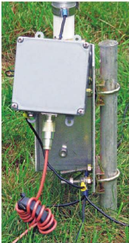
Figure 12 — A ferrite in-line choke is installed on the coax feed line to minimize common-mode current effects.
