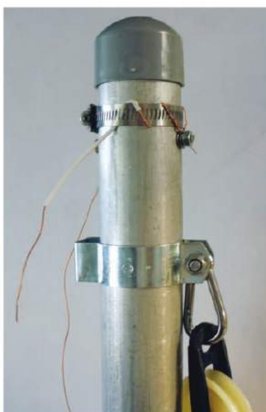
Figure 4 — The thin wires attach to the pole with a hose clamp, using soft sleeves to protect the wires.
