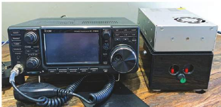
Figure 6 — The control box is to the right of the transceiver under the power supply. The two buttons activate loop tuning, while the potentiometer sets the tuning speed.
