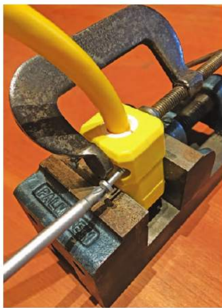
Figure 6 — Use a vise and C-clamp to close the clamshell while screwing the halves together. [Barry Shackelford, W6YE, photo]
