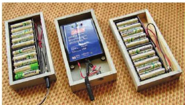
Figure 3 — The author's homemade wooden boxes help protect the battery holders (left and right) and solar panel controller (center) from being knocked around during handling. [Charles Hooker, VE3CQH, photo]
