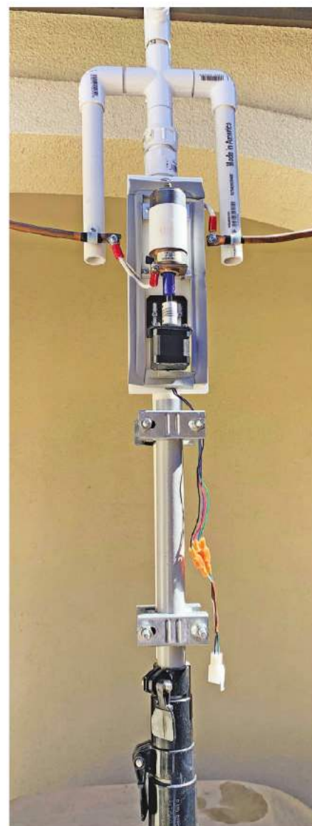
Figure 3 — The stepper motor and coupling (blue) attached to the tuning capacitor assembly, and the lower portion of the loop.
