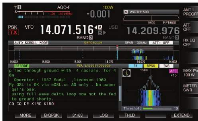
Figure 8 — The PSK decoder screen shows up to seven lines of decoded text in green in the larger window, and two lines of text to be transmitted in white below that. The tuning indicator on the right can be switched to a vector scope. Note the small version of the band scope above the decode window, and the compact bar graph meter at the upper left.
