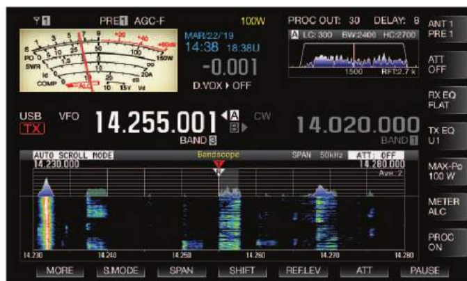
Figure 3 — The TS-890S display during SSB operation with the spectrum display/waterfall window set to show 50 kHz of the 20-meter band.
