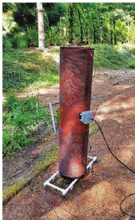
Figure 2 — The upper coil tunes the radiating element, and the lower coil tunes the radial system. Each coil is comprised of 95 turns spaced one wire diameter apart.
