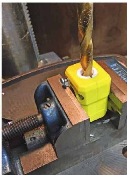
Figure 5 — Enlarge the diameter of the plug's clamping jaws. [Barry Shackelford, W6YE, photo]
