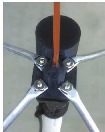
Figure 4 — Radials fashioned from 1/4-inch metal tubing and attached to the fixture with 6-32 hardware.
