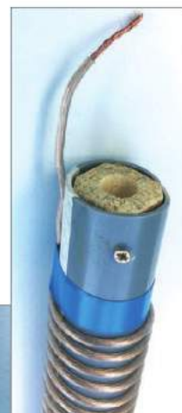
► Figure 3 — Drilled wooden insert installed in PVC pipe.
