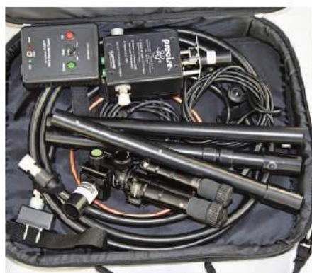
Figure 12 — The Deluxe HG-1 package in the supplied carrying case. The entire package, including antenna, mast, tabletop tripod, and controller weighs about 8 pounds.
