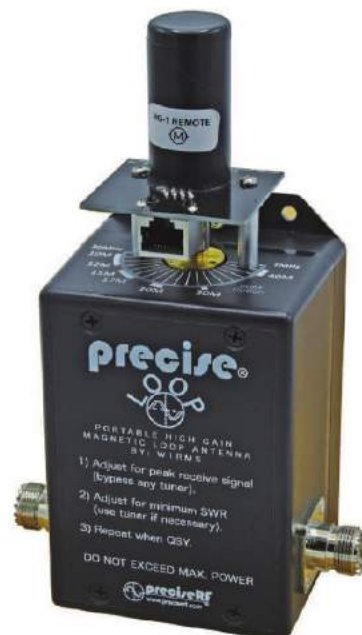
Figure 14 — The remote-control motor on the tuning box replaces the manual tuning knob.
