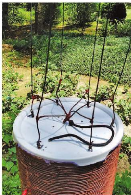
Figure 3 — The bottom of the cage structure attaches to the top of the coil form.
