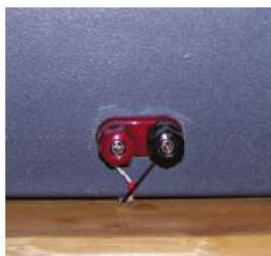
Figure 2 — The red and black binding posts on the rear of the speaker unit connect the speaker to the author's radio equipment. [Don Varner, WB3CEH, photo]
