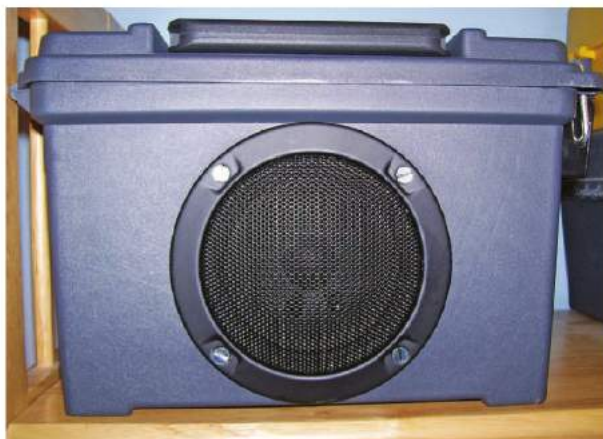
Figure 1 — The finished portable external speaker. [Don Varner, WB3CEH, photo]
