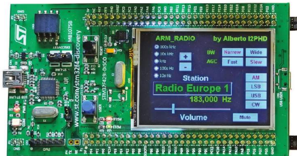
Figure 1 — Alberto di Bene's ARM Radio, an inexpensive software-defined receiver that covers 8 to 900 kHz. Full details are available at www.weaksignals.com . [Alberto di Bene, I2PHD, photo]
