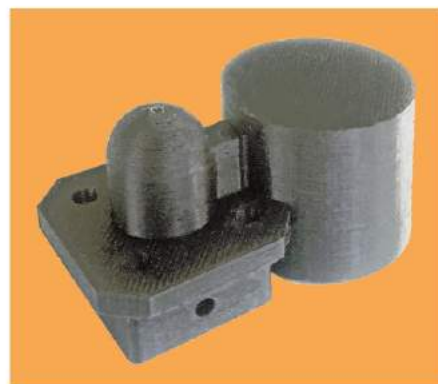
Figure 1 — Purpose-designed and 3D-printed plastic framework for an SO-239 VHF/UHF ground-plane antenna. The cylindrical cap at the right is sized to slip over the end of a 3/4-inch PVC pipe mast. Four ground-plane radials bolt to the horizontal member at the left of the mast-mounting cap. The SO-239 coax connector bolts to the radial elements through the bottom of the radial mount with the antenna's vertical element soldered to the connector's center pin and projecting through the dome of the small cylinder atop the radial mounting plate. Silicone is injected through the small hole in the side of the radial mounting plate for waterproofing.
