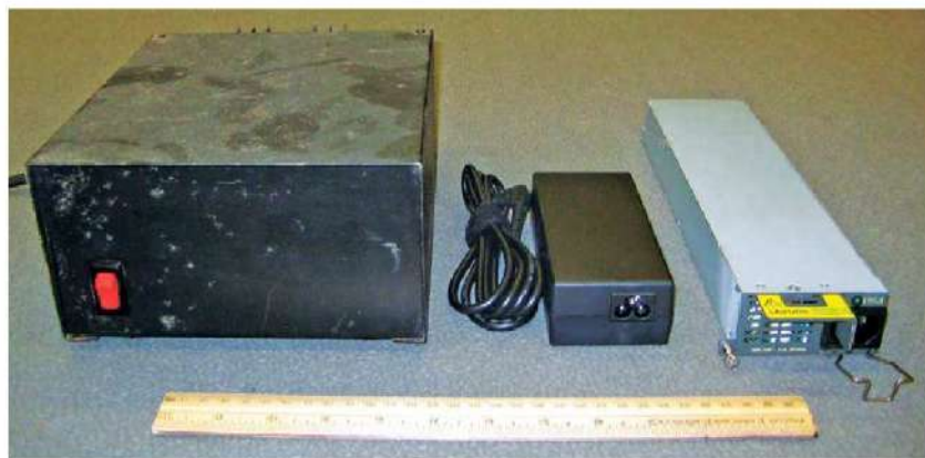
Figure 1 — Modern supplies use dc/dc switching to convert universal power input voltages both ac and dc into any required output voltage in only 10% of the space and weight of old 60 Hz supplies.
