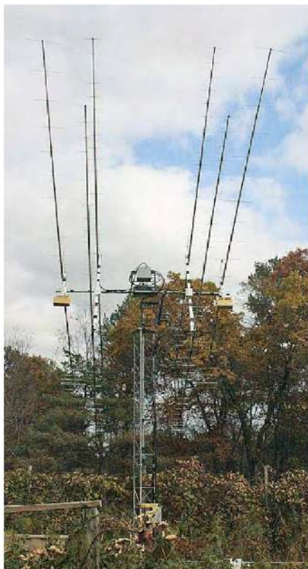
Figure 2 — Charlie's, NØAKC, 222 MHz EME array with two 222 MHz Yagis outside the inner four 70-centimeter Yagis. He has worked N9HF in Florida and K7ULS in Utah via EME with this antenna. [Charlie Betz, NØAKC, photo]
