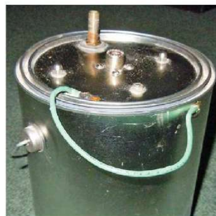
Figure 3 — A jumper wire soldered from the can to the lid got rid of the dummy load’s RF. [Al Forbes, KJ4YEV, photo]
