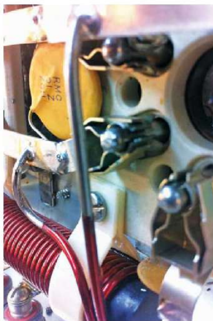
Figure 6 — The new spring clip compresses the pin holder tighter than before. [Dino Papas, KLØS, photo]
