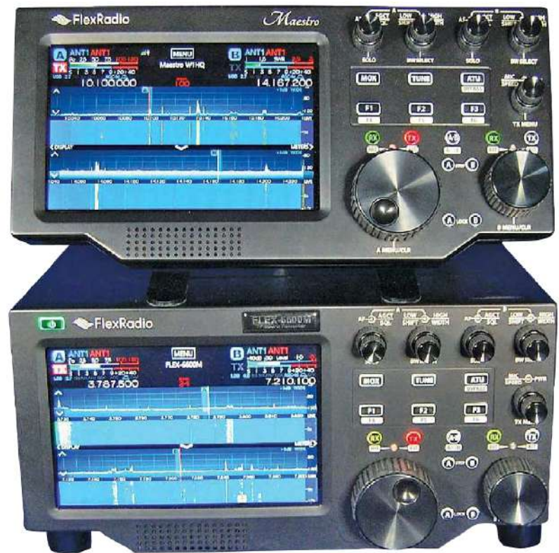
Figure 1 — MultiFlex operation with a Maestro (top) and FLEX-6600M transceiver connected to a single antenna. The Maestro receives 30 and 20 meters, while the FLEX-6600M receives 80 and 40 meters.
