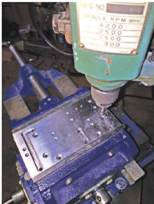
Figure 1 — A drill press used as a milling fixture.
