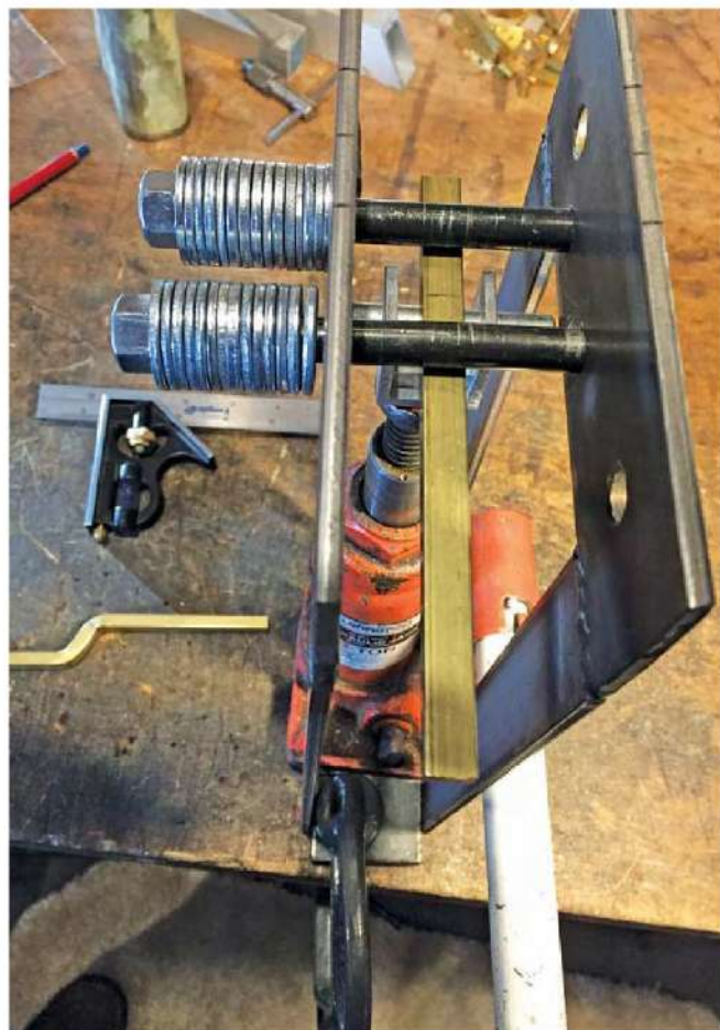
Figure 2 — A hydraulic jack mounted in a fixture for armature bending.
