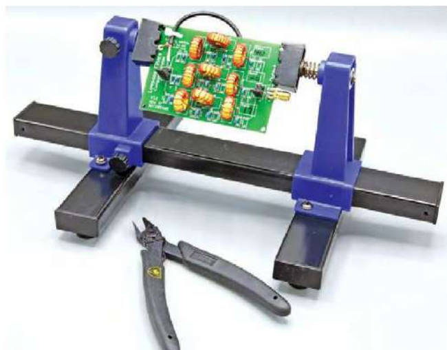
Figure 13 — The Aven Adjustable Circuit Board Holder resembles a lathe. The PC board is easily rotated.
