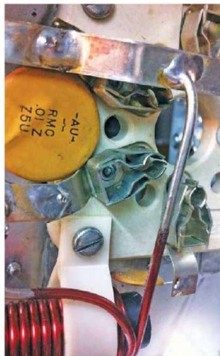
Figure 4 — The loose tube socket pin (compare the clip closure to the others). [Dino Papas, KLØS, photo]
