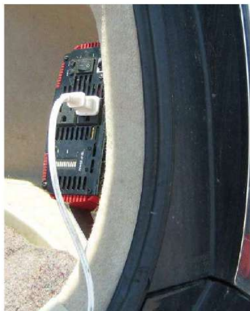
Figure 3 — Hybrids typically have 50 kW or more of HVDC generation capability. My Prius hack has outlets on the back for the 220 V dc hybrid power and for about 1,000 W from a 12 V inverter in the trunk.
