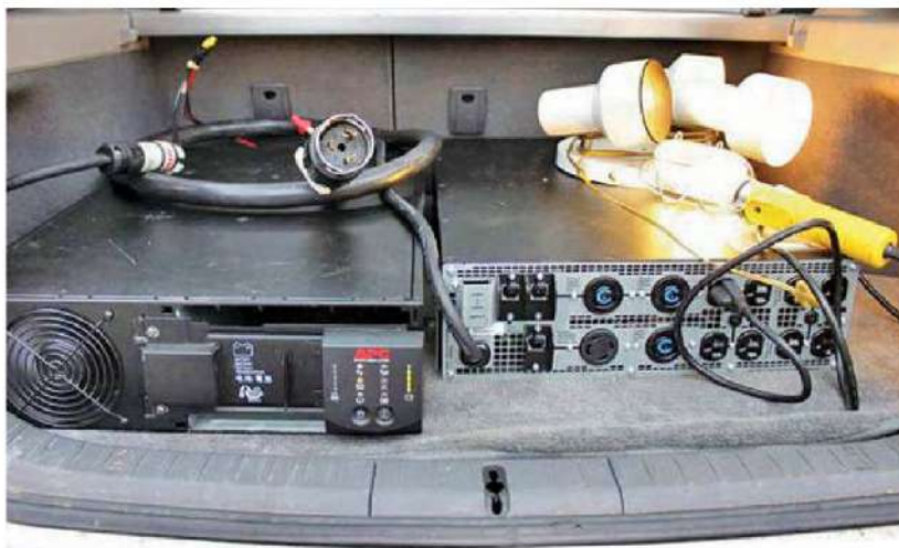
Figure 4 — Some rare data center UPS supplies take 192 V dc input to produce up to 6 kW emergency power, which is ideal when connected to the 200 V battery in a Prius, for example. [Doug Gaede, photo]
