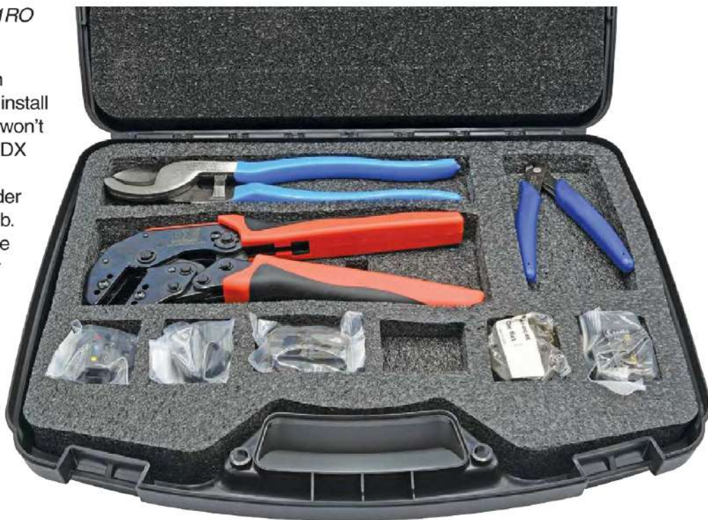
Figure 8 — The DX Engineering crimp tool and dies. The die for the Anderson Powerpole connectors is installed. The other dies (left to right) are used for RG-8 size coax, RG-8X and RG-58 size coax, and three sizes of insulated wire terminals. Another die for uninsulated terminals is included but not shown.
