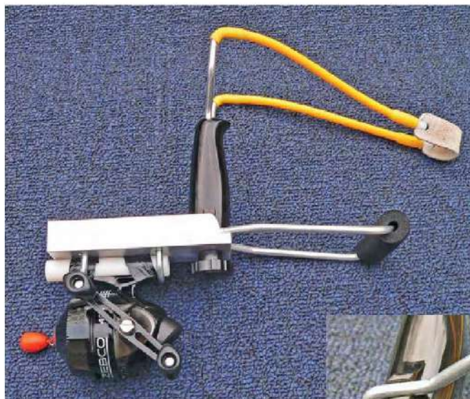
▲ Figure 1 — The finished slingshot launcher. [Steve Allen, KZ4TN, photo] ► Figure 2 — The press-in nut and knob screw. [Steve Allen, KZ4TN, photo] ▼ Figure 3 — The attachment of the reel to the aluminum channel. [Steve Allen, KZ4TN, photo]
