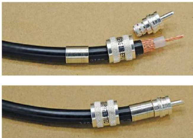
Figure 9 — Installing DXE Next Generation connectors on DXE-213 coax.
