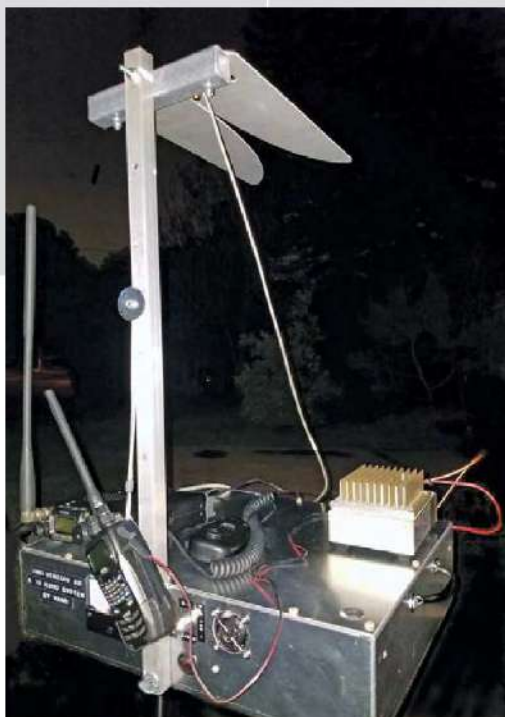
Wayne Overbeck, N6NB, built this 10-band Rover station, which covers 50 MHz up to 10 GHz. The wide-band Vivaldi antenna mounted on the unit covers 902 MHz through 10 GHz. Wayne secured the top spot in the Classic Rover category. [Wayne Overbeck, N6NB, photo]
