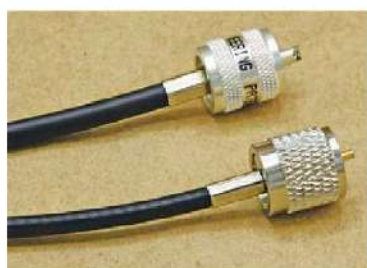
Figure 11 — A DXE Next Generation PL-259 installed on DXE-8X (top) and Amphenol 182100 PL-259 installed on DXE-58AU.
