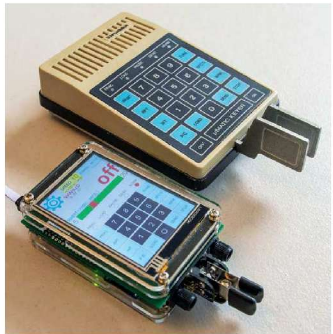
Figure 1 — The WW9JD Arduino-based μMatic2 Memory Keyer next to the original Heathkit SA-5010 μMatic Memory Keyer.
