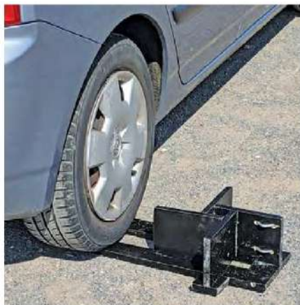
Figure 5 — To secure the support in the field, simply roll one of your vehicle tires onto the flat portion.
