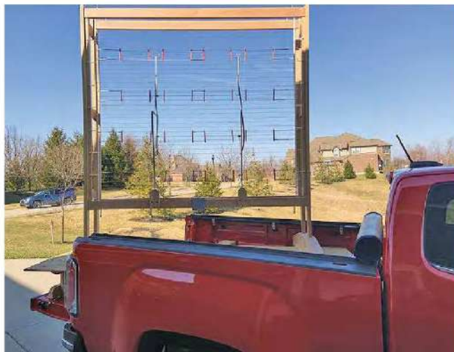
Figure 1 — A 432 MHz 4 × 2 curtain array built by Joe, WA8OGS, and Richard, WC8RK, pointing north toward Dayton, Ohio, for its first contact. The antenna is now an exhibit at the National Voice of America Museum of Broadcasting in West Chester, Ohio. [Joe, WA8OGS, photo]
