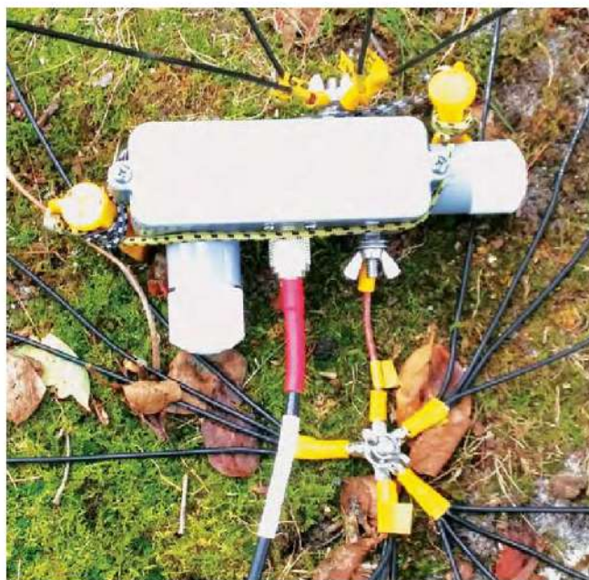
Figure 2 — Details of connections to the feed point. Note the optional use of a pigtail linking the radials to the feed point, simplifying the disconnection and reconnection of radials to the system.
