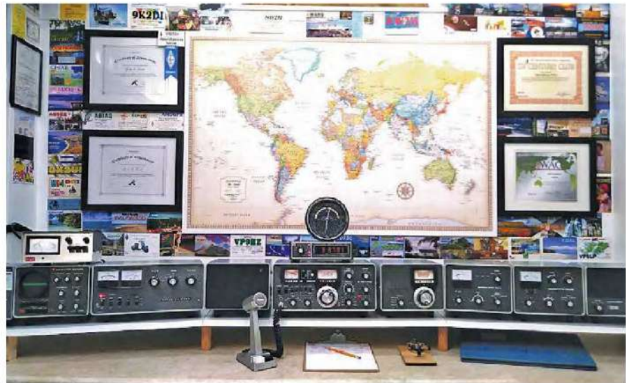
Figure 1 — Al Rabassa’s, NW2M, complete Yaesu station, which is fully operational. From left to right: YP-150 dummy load/wattmeter, YO-100 station monitor, FL-2100B 1,200 W amplifier, SP-101 desktop external speaker, YD-844 dynamic desk microphone, FT-101F transceiver, DD-1 digital frequency display, QTR-24 station clock, FV-101B remote VFO, FTV-250 2-meter transverter, FTV-650 6-meter transverter, SP-101PB external speaker with telephone patch. [Al Rabassa, NW2M, photo]
