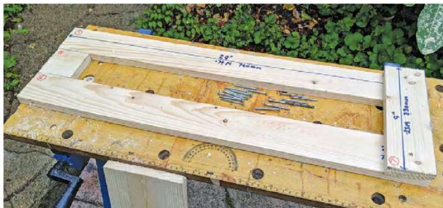
Figure 2 — Assemble the base using sections 5, 6, 7, and 8. Section 7 is raised and sits behind the inner tire wall when in use. Section 8 sits at the far end between sections 5 and 6. Prepare each screw by first drilling \frac{3}{16} -inch pilot holes.
