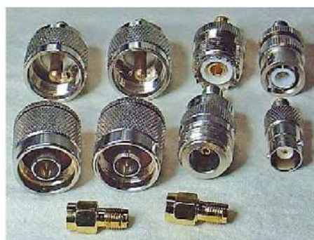
Figure 2 — The adapters purchased for NanoVNA use.
