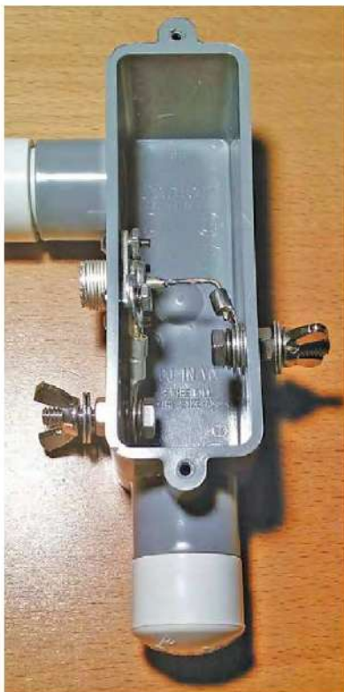
Figure 3 — Wiring and hardware detail of conduit box feed point.
