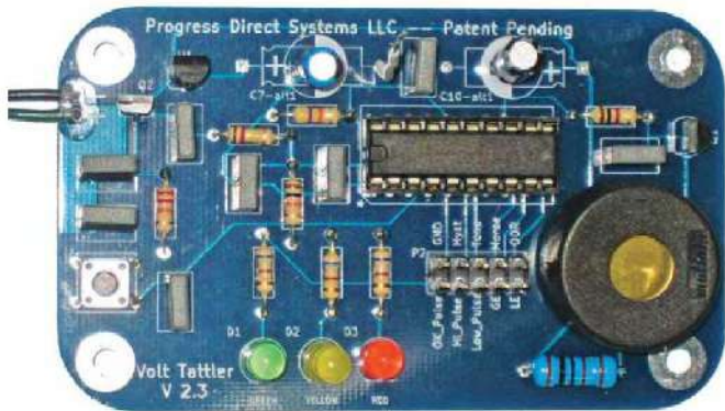
Figure 8 — The assembled Volt Tattler 2 PC board. The kit includes a two-pin header to connect leads from the voltage source to be monitored, but I found it convenient to solder wires to the PC board at the upper left. At the very top, under the letters LLC, is a wire connected to the common side for circuit measurements.
