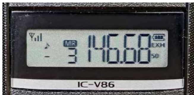
Figure 1 — The IC-V86 LCD conveys a lot of information about transceiver settings and status. The frequency display is a good size and very readable, but the other icons are quite a bit smaller.
