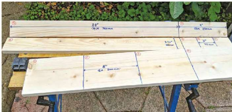
Figure 1 — All the wood parts are made by cutting the plank into numbered sections. Notice how the author marked the sections onto the board for easier cutting.
