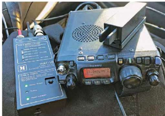
Figure 7 — The author's portable setup with the mAT-10 antenna tuner and Yaesu FT-817 during the CQ World Wide CW Contest, operating from Barnhart Prairie Preserve south of Champaign, Illinois. [Sean Kutzko, KX9X, photo]
