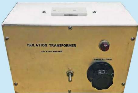
This enclosure holds a 150 W isolation transformer.
