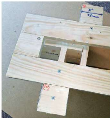
Figure 4 — Complete the assembly by attaching sections 9 and 10 to the protruding support sections. You can prime and paint everything if you wish.
