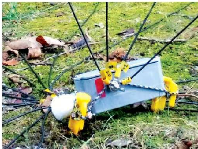
Figure 1 — Antenna elements departing the feed point at various angles. (Elements from left to right are for 20, 40, 30, and 60 meters.)
