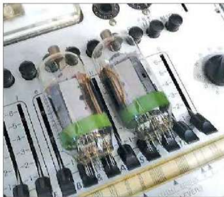
Figure 3 — An original pair of Toshiba green stripe sweep tubes used for RF power amplification from 160 meters through the 10-meter band. [AI Rabassa, NW2M, photo]
