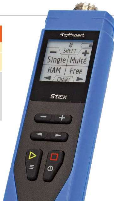
Figure 5 — The Stick 230 power-up screen and controls.
