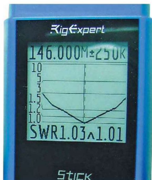
Figure 6 — SWR scan of 2-meter band-pass filter on the Stick 230 screen.
