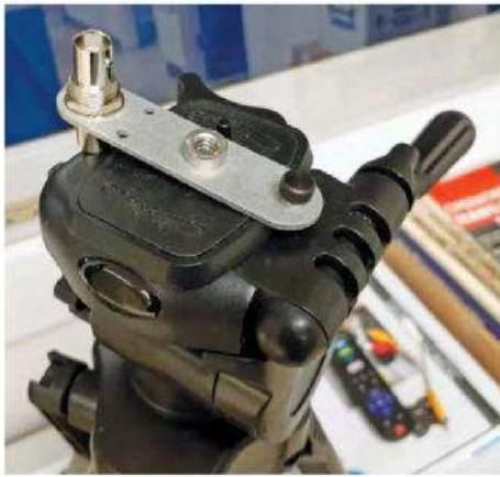
Figure 10 — The AXT1 Tripod Adapter is handy for mounting the antenna on a tripod, away from the operator, but it required a tripod without an integrated head.
