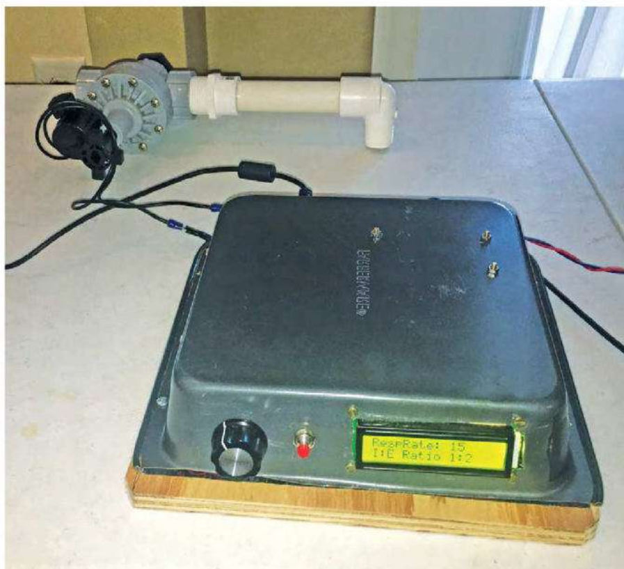
A mechanical ventilator control head, designed by medical professionals with the assistance of radio amateurs. [Photo courtesy of Dr. Gordon Gibby, KX4Z]
