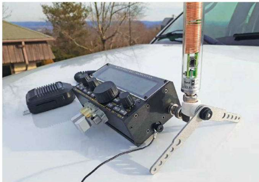
Figure 9 — The AX1 mounted on a KX2 transceiver with the optional AXB1 Whip Bipod.
