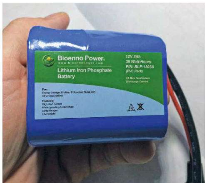
Figure 3 — This small 3 Ah lithium iron phosphate battery will provide energy for hours using any of the popular QRP radios.
