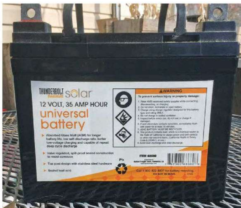
Figure 1 — A lead-acid U1 scooter battery is rated at 35 Ah capacity.
