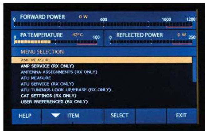
Figure 2 — The ACOM 1200S offers a number of menus for configuring and using the amplifier.
