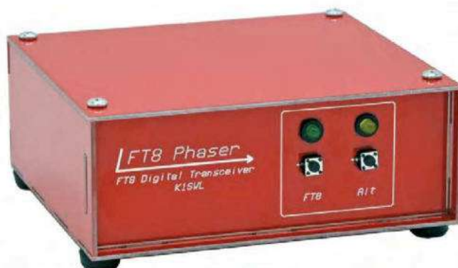
Figure 5 — The Phaser enclosure front panel includes switches and LED indicators for selecting the standard FT8 frequency or alternate (user-programmed) frequency. (Note that the TRANSMIT indicator LED incorporated into the latest version could be mounted on the front panel as well.)
