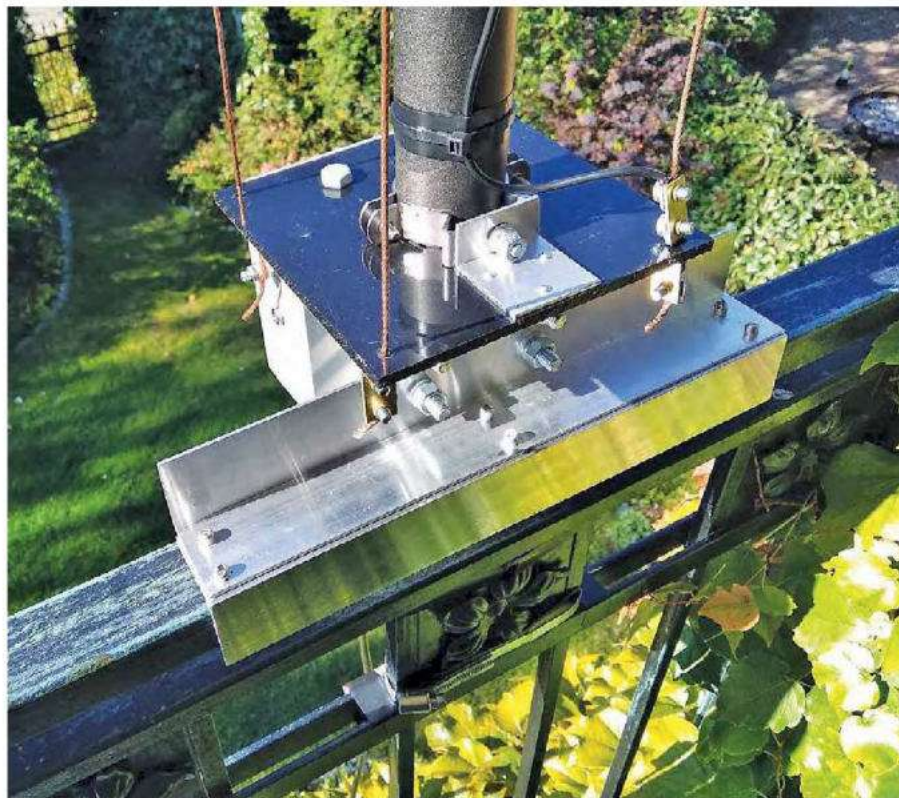
Figure 3 — Details of the mounting plate and the railing mount of the antenna.
