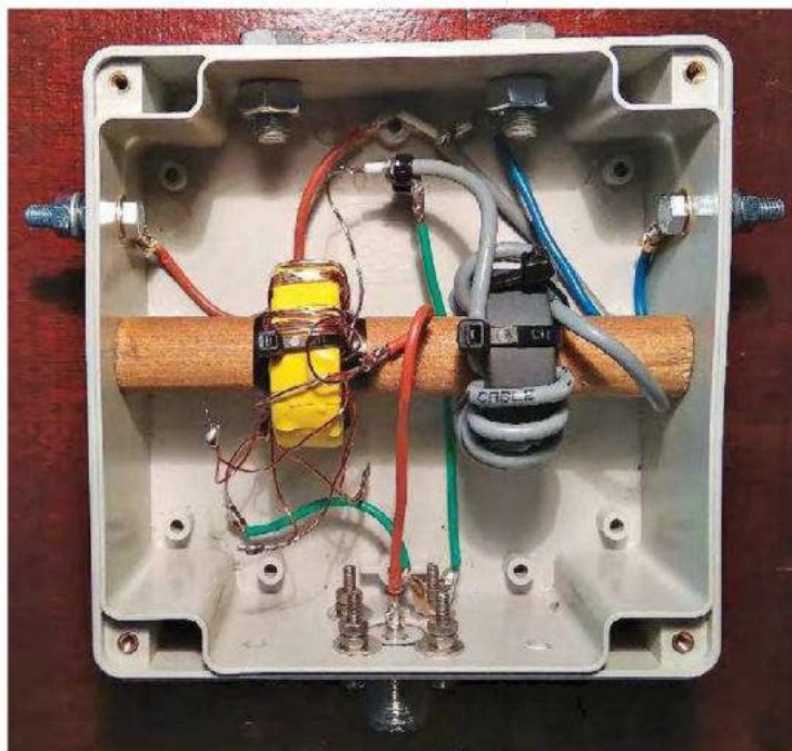
Figure 5 — The matching network box houses transformer TR1 and common-mode choke TR2. The core for TR1 is taped with yellow electrical tape.
