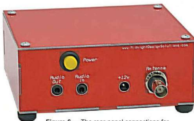
Figure 6 — The rear-panel connections for AUDIO IN/OUT, ANTENNA, and POWER.
