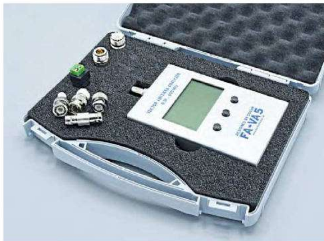
Figure 4 — The FA-VA5 with optional case, various optional adapters, and the optional high-quality four-piece calibration kit (at the lower left).
