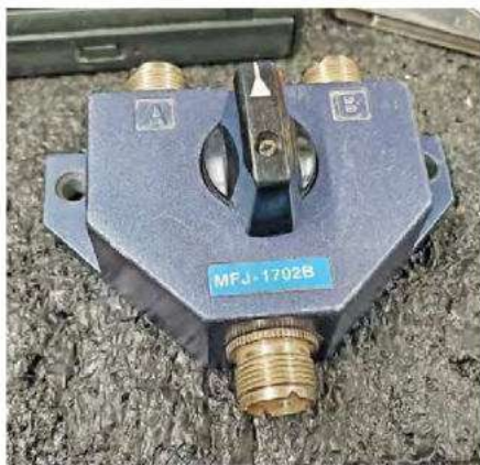
Figure 4 — The MFJ-1702 coaxial switch has a common port switched between two separate ports. [Clint Millett, VE3CMQ, photo]
