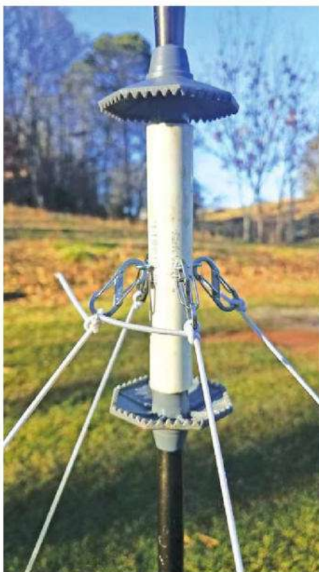
Figure 1 — A close-up of the center coupling arrangement shows the 3D-printed components at each end of the PVC section. Carabiners attach guy lines to the screw eyes.
