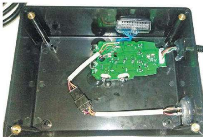
Figure 7 — The clone MH-48 PCB and new wiring, shown inside the new controller housing.
