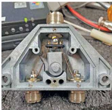
Figure 5 — A rubber O-ring washer across the connections increases the holding tension. [Clint Millett, VE3CMQ, photo]
