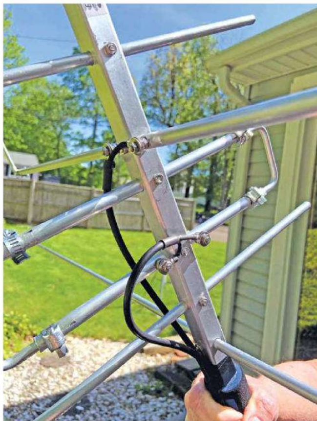
Figure 13 — In this close-up view, you can see the separate feed lines attached to the driven loop elements. You can also see the sliding end sections and hose clamps.
