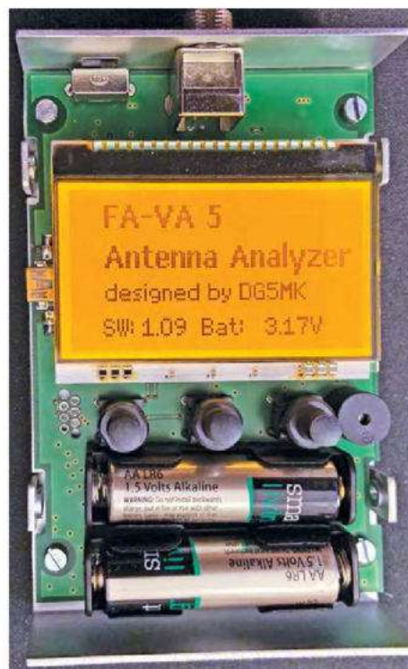
Figure 5 — FA-VA5 startup screen, along with an interior view of the completed kit.
