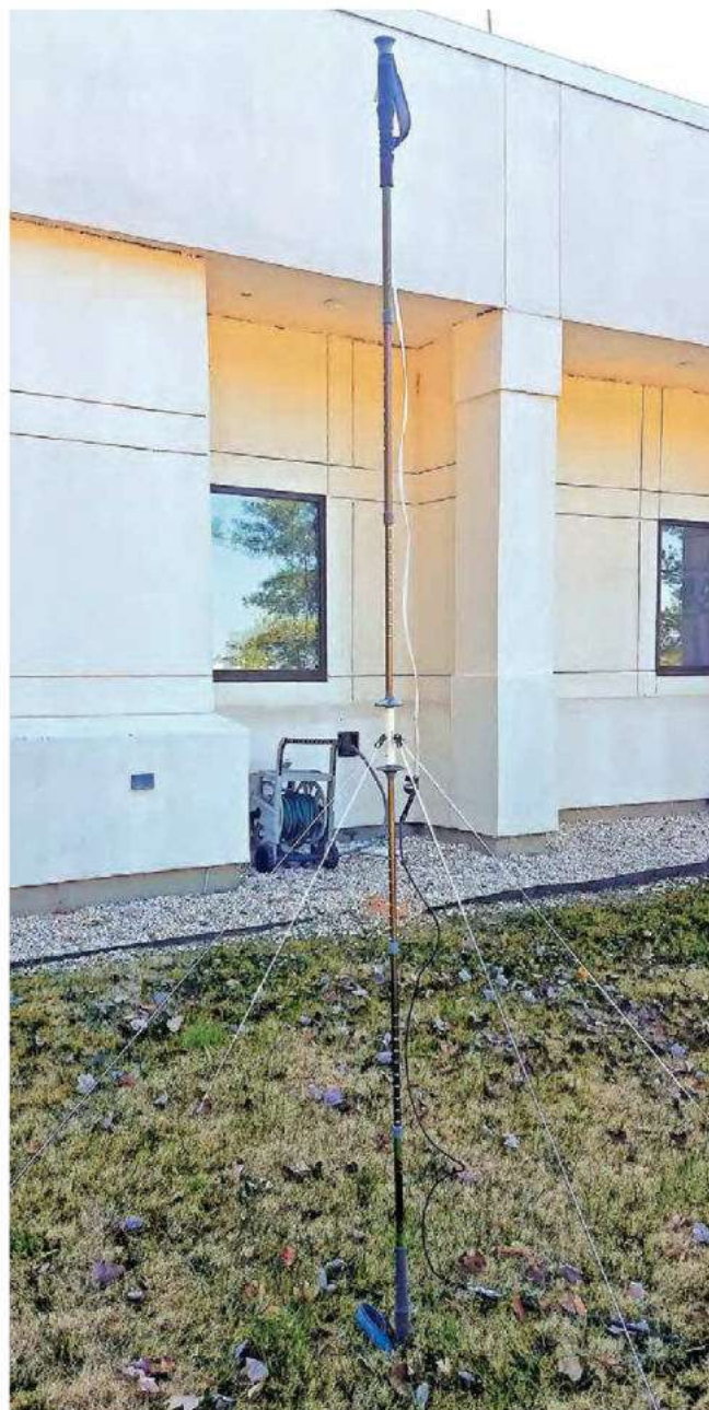
Figure 2 — The mast system is shown supporting a twin-lead rollup VHF J pole at the 2019 SKYWARN™ Amateur Radio Recognition Day at the Greenville-Spartanburg, South Carolina, National Weather Service office.
