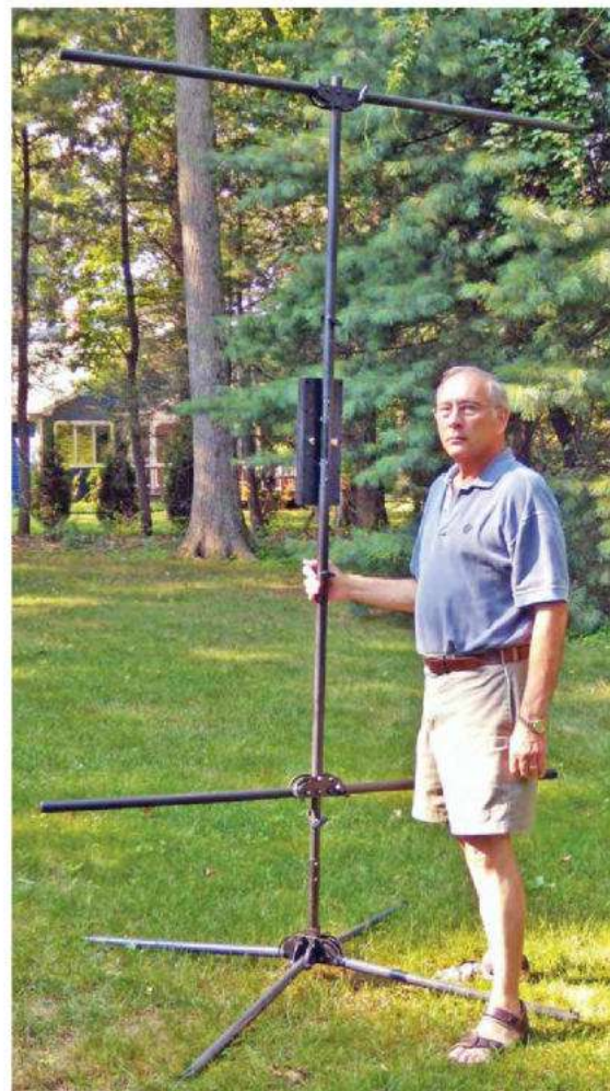
Figure 1 — W1ZR adjusting the Transworld Adventurer antenna. This is a possible solution for antenna-restricted areas, because it can be easily moved, disguised, or broken down when not in use. [Nancy Hallas, W1NCY, photo]
