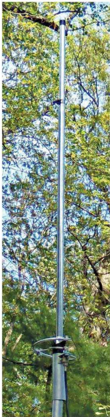
◀ Figure 11 — The completed antenna AR-2 temporarily positioned for adjustment on top of a 1.25-inch aluminum TV mast section.
