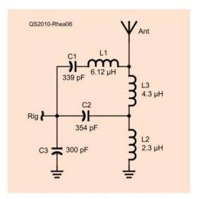
**Figure 6** — Antenna-matching network for the 80-, 40-, and 30-meter bands.
