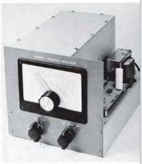
Front view of WA3EQK's VFO. The unit operates on 3.5 to 4 and 7 to 7.3 MHz. Included are a 2-watt amplifier and broadband rf transformers so that the VFO can drive tube-type transmitters directly.
