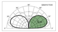
Figure 3 — The 43-foot vertical antenna is % wavelength on 40 meters for a 3 dB gain reduction.
