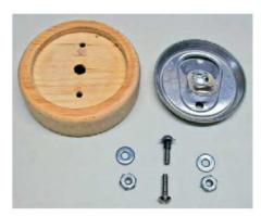
Figure 3 — The can top is secured to the base with two  $6-32 \times \frac{1}{2}$  inch long machine bolts. [Karl Schwab, KO8S, photo]
