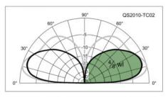
Figure 2 — The 43-foot vertical antenna is  $\frac{1}{2}$  wavelength on 30 meters. This results in about a 2 dB reduction in maximum gain.
