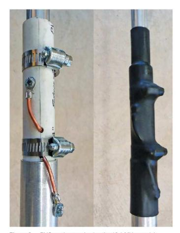
**Figure 2** — PVC section terminating the 10.1 MHz coaxialstub trap at 60 feet, before (left) and after (right) applying heat-shrink tubing.
