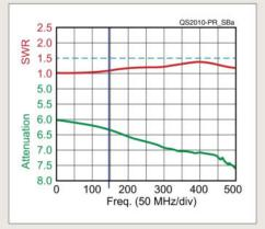
**Figure A** — SWR and insertion loss sweep of the HecKits attenuator with 6 dB attenuation selected.
