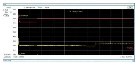
**Figure 4** — Kenwood PS-60 conducted emissions from 150 kHz to 30 MHz with a 1 A load. The red lines at the top of each plot represent the FCC limit of conducted emissions based on frequency.
