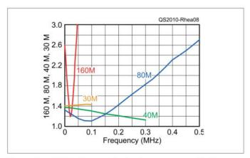
**Figure 8** — SWR of the matched antenna measured in the shack through 120 feet of LM400 coax cable. Frequency shown is from the bottom of each band.
