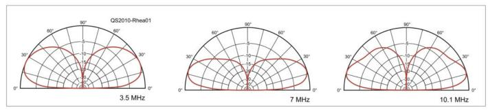
Figure 1 — EZNEC-simulated elevation patterns for the vertical over a medium ground.
