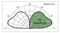
**Figure 1** — On 20 meters, the elevation plot of the 43-foot vertical antenna is labeled with its fraction of a wavelength:  $\frac{1}{2}$ . In my estimation, this is the gold standard for takeoff angles (TOA).
