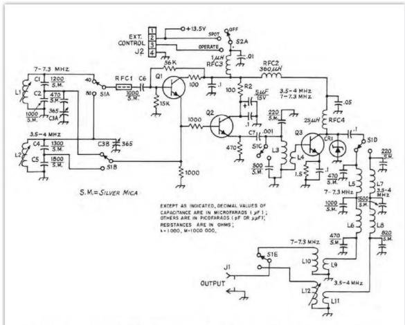
Fig. 1 - Schematic diagram of the VFO. Resistors are 1/2-watt composition; capacitors, except those marked as silver mica, are disk ceramic. Parts not listed below are marked for text reference.
