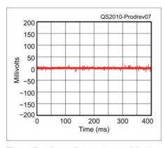
**Figure 7** — An oscilloscope trace of the dc output of the Yaesu FP-1030A with a 20 A load. The vertical scale is 50 mV/div, and the horizontal scale is 5 ms/div.
