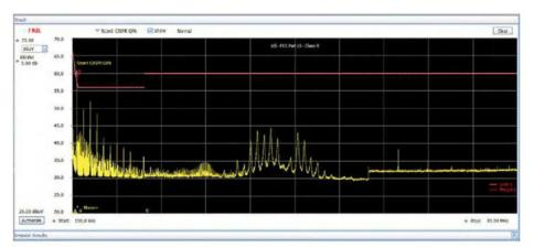
**Figure 2** — Alinco DM-430T conducted emissions from 150 kHz to 30 MHz with a 1 A load. The red lines at the top of each plot represent the FCC limit of conducted emissions based on frequency.
