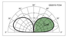
Figure 4 — The 43-foot vertical antenna is  $\frac{1}{2}$  wavelength on 60 meters, with gain comparable to 40 meters.
