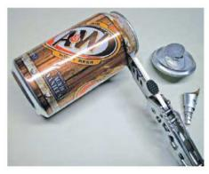
**Figure 1** — Cut away the top of the can with scissors or any other suitable tool. [Karl Schwab, KO8S, photo]
