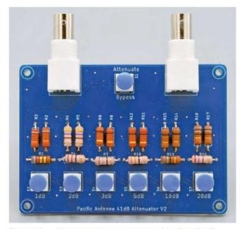
**Figure 11** — All components mount on one side of the Pacific Antenna attenuator PC board. The top switch bypasses the attenuator. Either BNC connector can be used as input or output.
