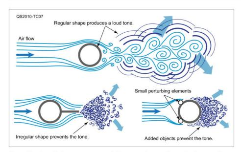
**Figure 7** — Acoustic tones can occur as air flows around a smooth, regular shape, such as a mobile antenna. By adding irregularly shaped elements to the antenna, it is possible to disrupt the downstream air flow and prevent the production of tones.
