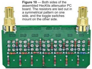
two solder pads on the two top corners; the reverse side, where the resistor leads are soldered, has three pads near each corner. Figure 10 shows the assembled board.
