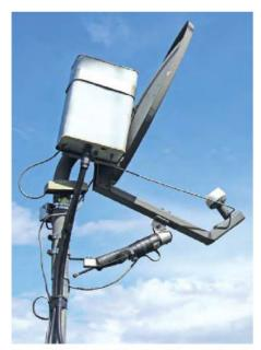
**Figure 3** — A 10 GHz dish with a cordless screwdriver and threaded rod for elevation adjustment. [Bill Davis, KØAWU, photo]
