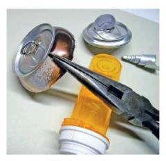
Figure 2 — With pliers, grip the remaining metal at the top of the can and roll the pliers around the circumference of the lid, removing all the metal. [Karl Schwab, KO8S, photo]
