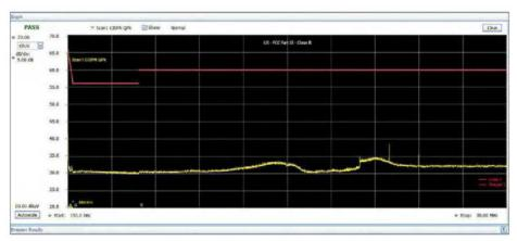
**Figure 8** — Yaesu FP-1030A conducted emissions from 150 kHz to 30 MHz with a 1 A load. The red lines at the top of each plot represent the FCC limit of conducted emissions based on frequency.
