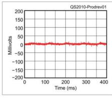
Figure 1 — An oscilloscope trace of the dc output of the Alinco DM-430T with a 20 A load. The vertical scale is 50 mV/div, and the horizontal scale is 5 ms/div.
