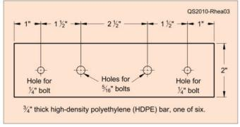
Figure 3 — Drill-hole pattern for a  $\% \times 2 \times 7\%$  inch high-density polyethylene (HDPE) hinge. Six hinges are needed.
