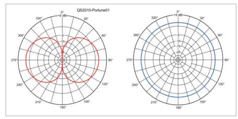
Figure 1 — Elevation (red), azimuth (blue) free-space radiation patterns.
