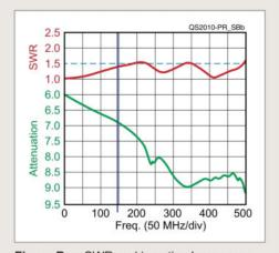
**Figure B** — SWR and insertion loss sweep of the Pacific Antenna attenuator with 6 dB attenuation selected.
