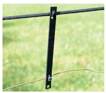
**Figure 13** — Sturdy  $\frac{3}{16}$ -inch UV-resistant dacron/polyester rope supports the #18 AWG solid antenna wire. The wire is quite stiff, and it takes some experimentation to get it to look like the photo at **www.hybriddx.com**.
