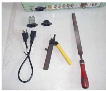
**Figure 5** — You can enhance the electrical safety of older gear by replacing the two-wire ac cord with a socket to accommodate a three-wire cord. Both filtered and unfiltered sockets are shown here. [Patrick Hamel, W5THT, photo]
