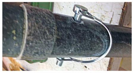
Figure 4 — The mast after holes are drilled and the hitch pins inserted.
