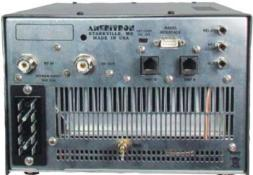
New! Ameritron ALS-606S/ALS-606 Solid State 600 Watt amplifier covers 160-6 Meters and automatically bandswitches by your transceiver.
