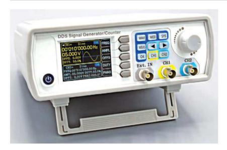
When set to generate a waveform, the 2.4-inch TFT color LCD confirms the settings and displays the selected waveform. It also serves as the readout for the measuring capabilities. The enclosure measures approximately  $2.7 \times 7.6 \times 7$  inches.
