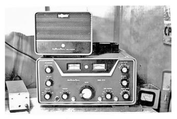
**Figure 1** — The Hallicrafters HT-44 transmitter. [Mike Dodd, N4CF, photo]
