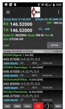
**Figure 2** — The RFinder B1 application's main window.
