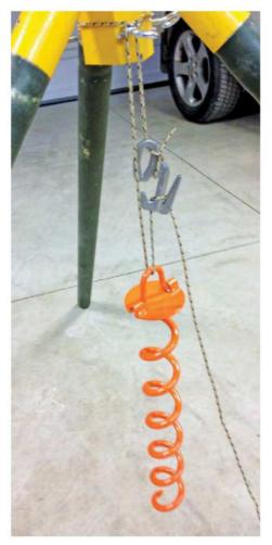
**Figure 6** — A view of how the tripod rope tightener and ground anchor are connected together using paracord.
