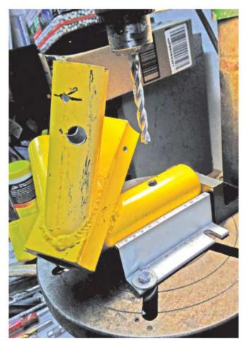
Figure 2 — Positioning a tripod leg for drilling.
