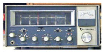
Figure 2 — The Hallicrafters SX-146 receiver. [Photo courtesy of www.universal-radio.com]
