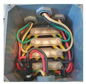
Figure 6 — The interior of the RPT box. The ac mains come in at the bottom, pass through the fuses on the left, and are then connected to the bus bars for distribution to the three output connectors exiting at the top. [Paul Christensen, W9AC, photo]
