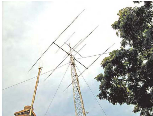
Karl Schwab, KO8S, has an antenna farm in Michigan, which consists of a 64-foot aluminum tower, stacked with multiple Yagi antennas to cover a wide spectrum of bands, including 440 MHz, and 2, 6, 10, 15, 20, and 160 meters.
