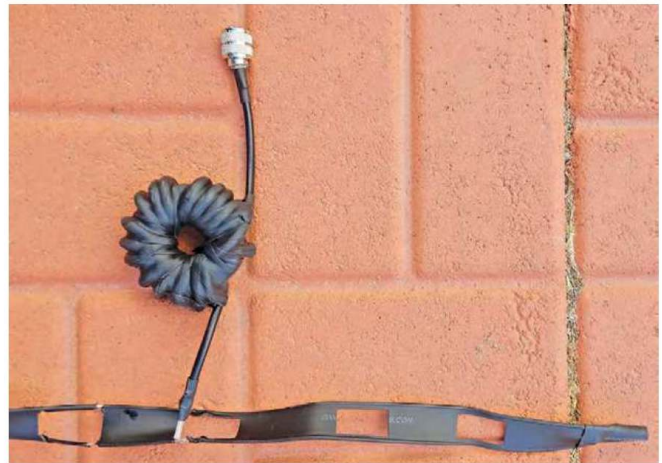
Figure 4 — The connection of the balun to the matching section.
