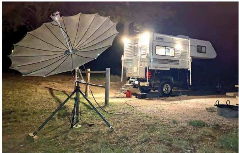
Figure 3 — Gene, KB7Q, set up a portable 23-centimeter EME operation in Wyoming on September 30, 2021. [Gene Shea, KB7Q, photo]
