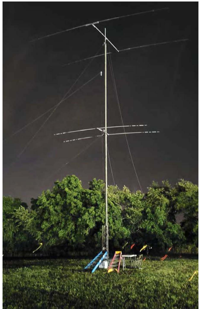
The Gloucester County Amateur Radio Club, W2MMD, in New Jersey, operated at night during the 2021 ARRL Field Day, with antennas for the 15-, 20-, and 80-meter CW stations. The antennas were supported by a portable aluminum military mast, which takes about an hour to deploy. [Vincenzo Sallustio, N4NYY, photo]
