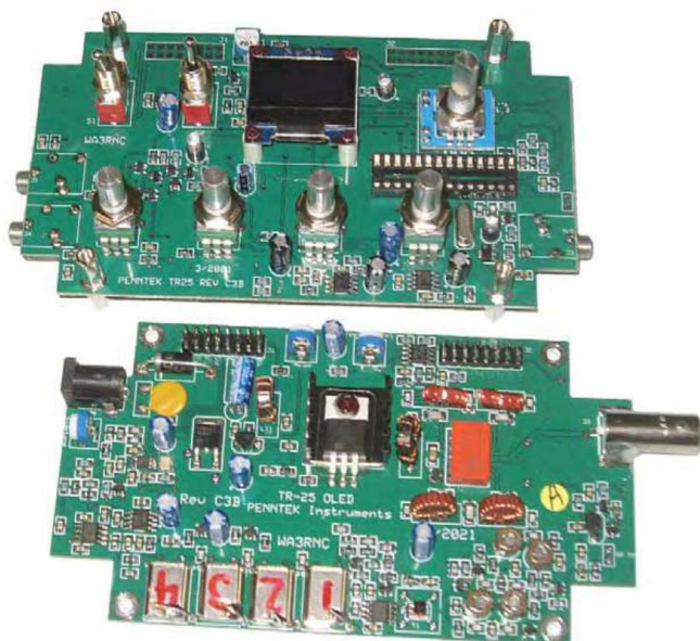
Figure 1 — The kit is assembled as two PC boards. The upper board contains the display and controls. On the center right is the microcontroller. This IC is plugged in after the two boards are assembled as a sandwich. The lower board has the final amplifier FET and heatsink in the center. The numbered and matched filter crystals are along the bottom edge.
