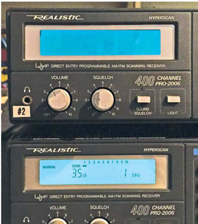
Figure 4 — It's obvious which scanner has the replacement backlight panel!
