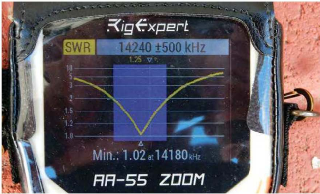
Figure 6 — An antenna analyzer shows the achievable SWR.
