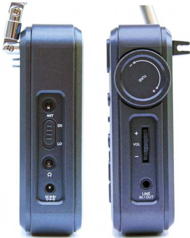
Figure 3 — The left side of the receiver has an external antenna jack, a DX/local switch to reduce gain if the receiver overloads, a stereo headphone jack, and an external power jack. The right side includes tuning and volume controls and a line in/out jack.
