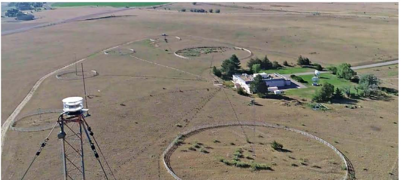
An aerial view of WWV. The station broadcasts six frequencies with their own antennas, which are all surrounded by a white fence. The lowest frequency has the tallest antenna, and it requires a flashing strobe to be visible to passing aircraft.
