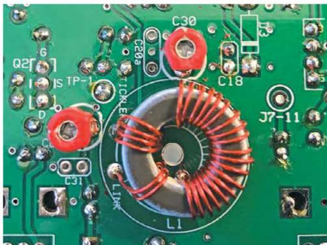
Figure 2 — This triple-winding toroid assembly forms the heart of the Bayou Jumper's regenerative receiver.
