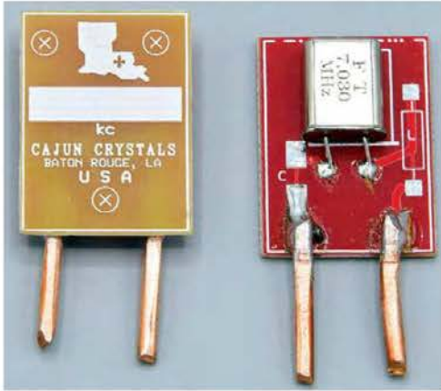
Figure 4 — HC-49/U crystals mounted on the two small circuit boards supplied with the kit.
