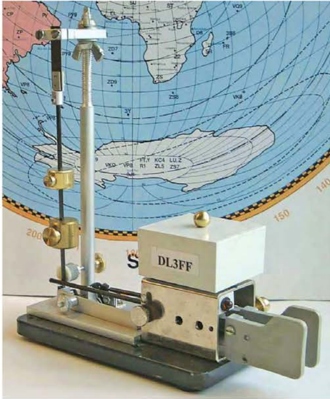
Figure 3 —The pendulum bug with oscillation release.
