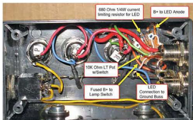
Figure 3 — I built the LED control components into a mobile power-control box of my own design, but any small enclosure will do. All you need is a box that you can mount near the radio so that you can easily adjust the potentiometer.
