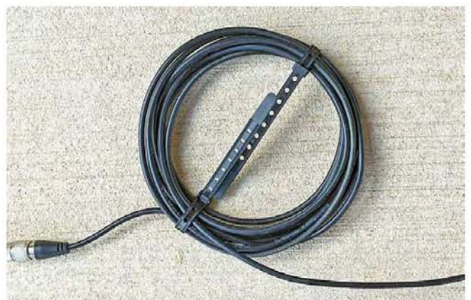
Figure 4 — The finished balun.
