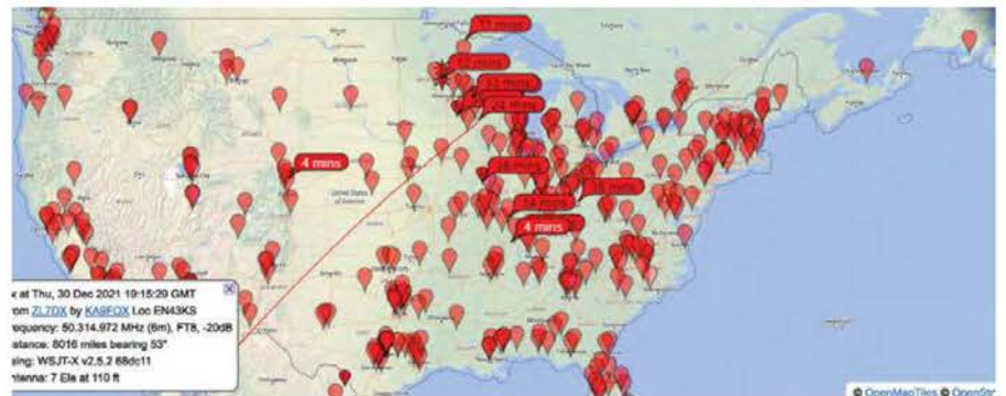
Figure 1 — A PSK Reporter map of the 6-meter FT8 flags from ZL7DX Chatham Island to the upper Midwest US at 1915 UTC on December 30, 2021. [ https://pskreporter.info ]
