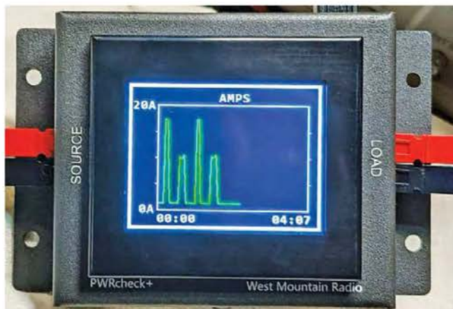
Figure 5 — Key down (tall spikes), and 20 WPM string-of-dits current plot are shown on the PWRcheck+ screen.
