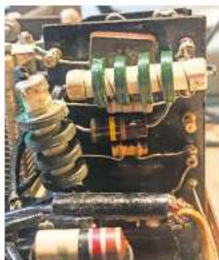
Figures 3 and 4 — These two figures show the modifications performed. Figure 3 (on the left) shows the two new RFCs and two replacement resistors in the voltage divider circuit. Figure 4 (on the right) shows the 2 W, 100 \Omega , wire-wound parasitic choke mounted behind the tube socket.
