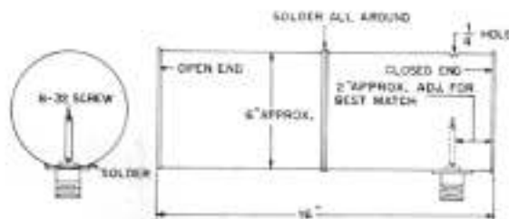
Fig. 1 - Dimensions for the wave-guide-transition feed for 1296-MHz use. The wave guide is made from two antifreeze cans soldered end to end.
