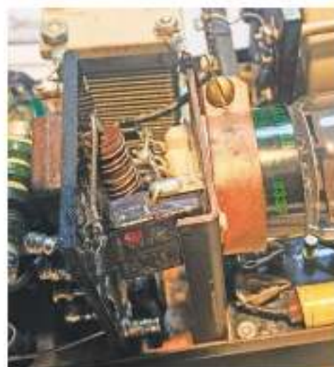
Figures 3 and 4 — These two figures show the modifications performed. Figure 3 (on the left) shows the two new RFCs and two replacement resistors in the voltage divider circuit. Figure 4 (on the right) shows the 2 W, 100 \Omega , wire-wound parasitic choke mounted behind the tube socket.
