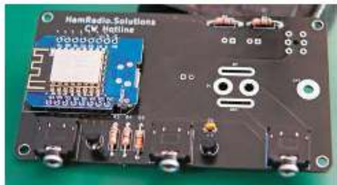
Figure 6 — A nearly assembled board ready to be soldered into place. But wait! The ESP8266 shown here is placed incorrectly. Always double-check that you have the electronics part in the correct orientation prior to soldering the components in place.
