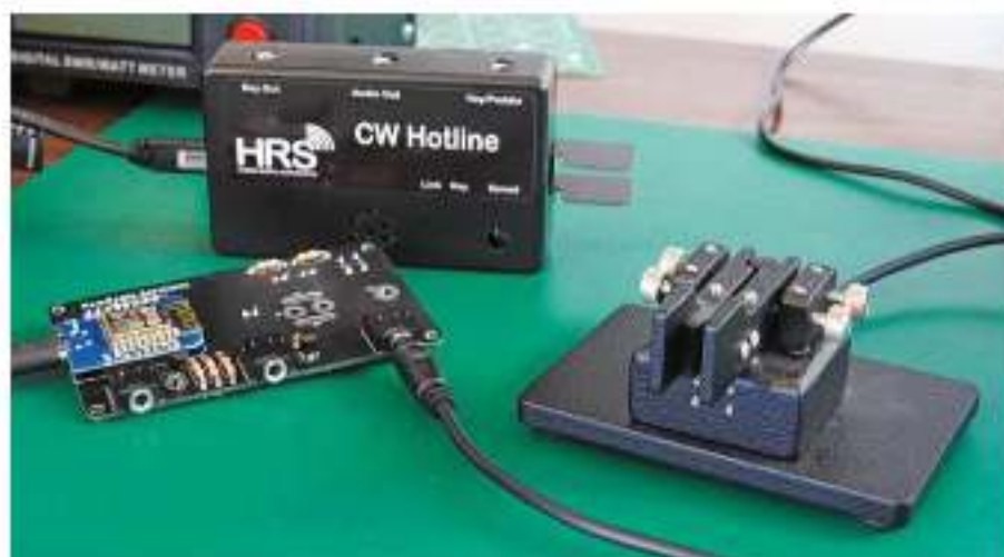
Figure 7 — Two CW Hotline kits working together. For my second kit, I chose not to install a straight key or paddle, as it will be used with an external key.
