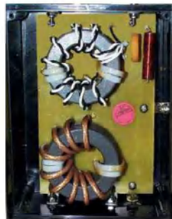
Inside of Matching Unit
