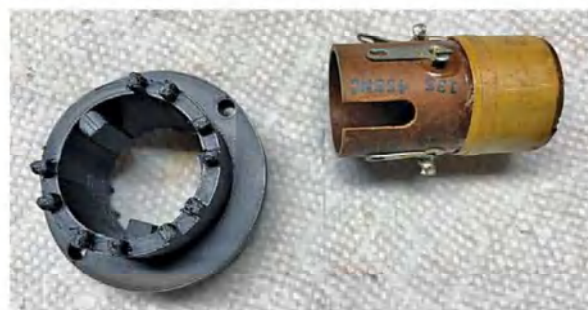
The Meissner 18-3502 coil (on the right) and #9693 socket copy that I made with polylactic acid plastic using my 3D printer.
