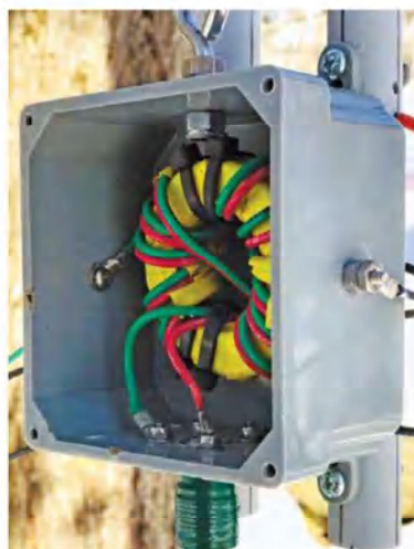
Figure 3 — The feed-point box with the balun installed and PVC spacers attached to the box-mounting tabs.
