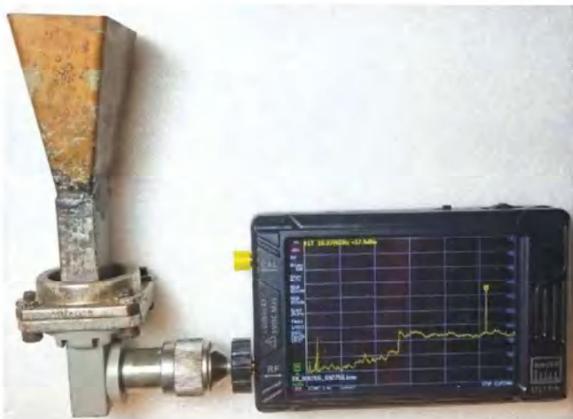
Figure 4 — An inexpensive tinySA Ultra spectrum analyzer displays a clean output from my 10 GHz dish. The horn antenna was held off to the side — never stand in front of the antenna while transmitting.
