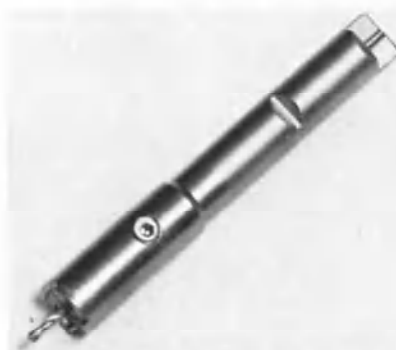
Fig. 4 — Tool used in isolated-pad construction. Set screw allows removal of the No. 60 center drill. The shank will fit either an ordinary hand drill or certain push-type screwdrivers.
