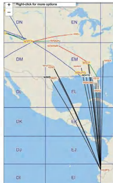
Figure 1 — An F2 opening on 6 meters occurred on January 6, 2023, between the southeast US and Ecuador. [www.dxmaps.com]
