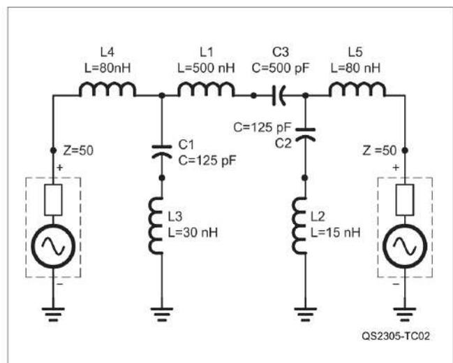
Figure 2 — For use on the HF bands, I simulated and built this 30 MHz low-pass filter.
