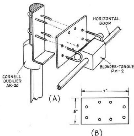
Fig. 3 - The method of mounting two rotators together. A pair of PM-2 rotators may also be used. The adapter plate (B) may be fabricated from 1/4-inch-thick aluminum stock, or a ready-made plate is available from Blonder-Tongue.
