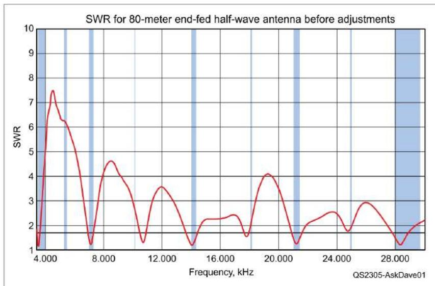
**Figure 1** — Joe Barcelo, KB2JSB, measured the SWR across the entire range of the ARRL EFHW antenna kit after he had extended it by 66 feet. He used his RigExpert AA-600 and the included *AntScope2* software. The measurements show excellent results of the extended antenna, including on the bottom of 80 meters.
