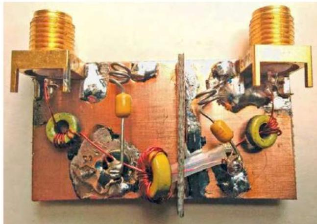
shielded it. Then I saw the AM band come to life. With the added 26 dB low-noise amplifier and a way to attenuate the FM signals, the screen began to display the weak signals.
