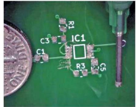
**Figure 4** — Syringe-applied solder paste.
