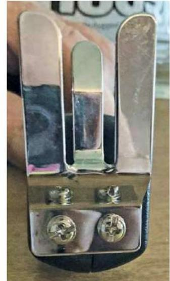
**Figure 7** — Using small screws, attach the microphone connector to the top of the adapter.
