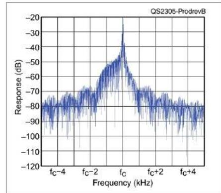
**Figure B** — Spectral display of the Xiegu G106 transmitter during keying sideband testing. Equivalent keying speed is 60 WPM using external keying and the default rise time setting. Spectrum analyzer resolution bandwidth is 10 Hz, and the sweep time is 200 ms. The transmitter was being operated at 5 W PEP output on the 14 MHz band, and this plot shows the transmitter output  $\pm$  5 kHz from the carrier. The reference level is 0 dBc, and the vertical scale is in decibels.
