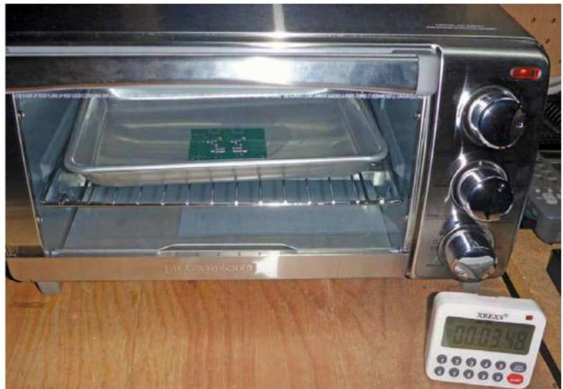
**Figure 5** — The toaster oven soldering station.
