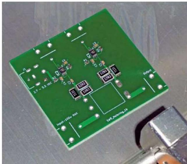
**Figure 7** — The final soldered SMD assembly.
