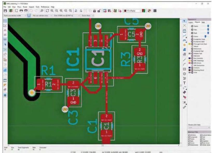
**Figure 1** — A screenshot of the *KiCad* PCB design editor. Red traces are on the top layer, and green traces and ground plane fill are on the bottom layer.
