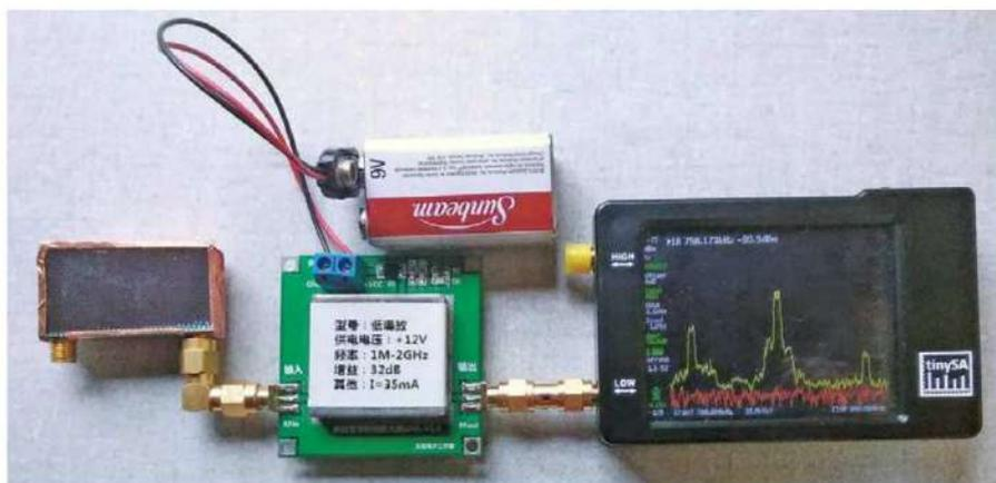
**Figure 4** — The completed setup with the shielded filter, amplifier, and tinySA.
