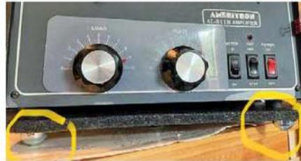
**Figure 5** — Adding a set of small wheels (circled in yellow) to my amplifier cabinet made it easy to maneuver in tight spaces.
