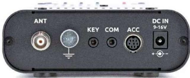
Figure 2 — Rear panel connectors.
