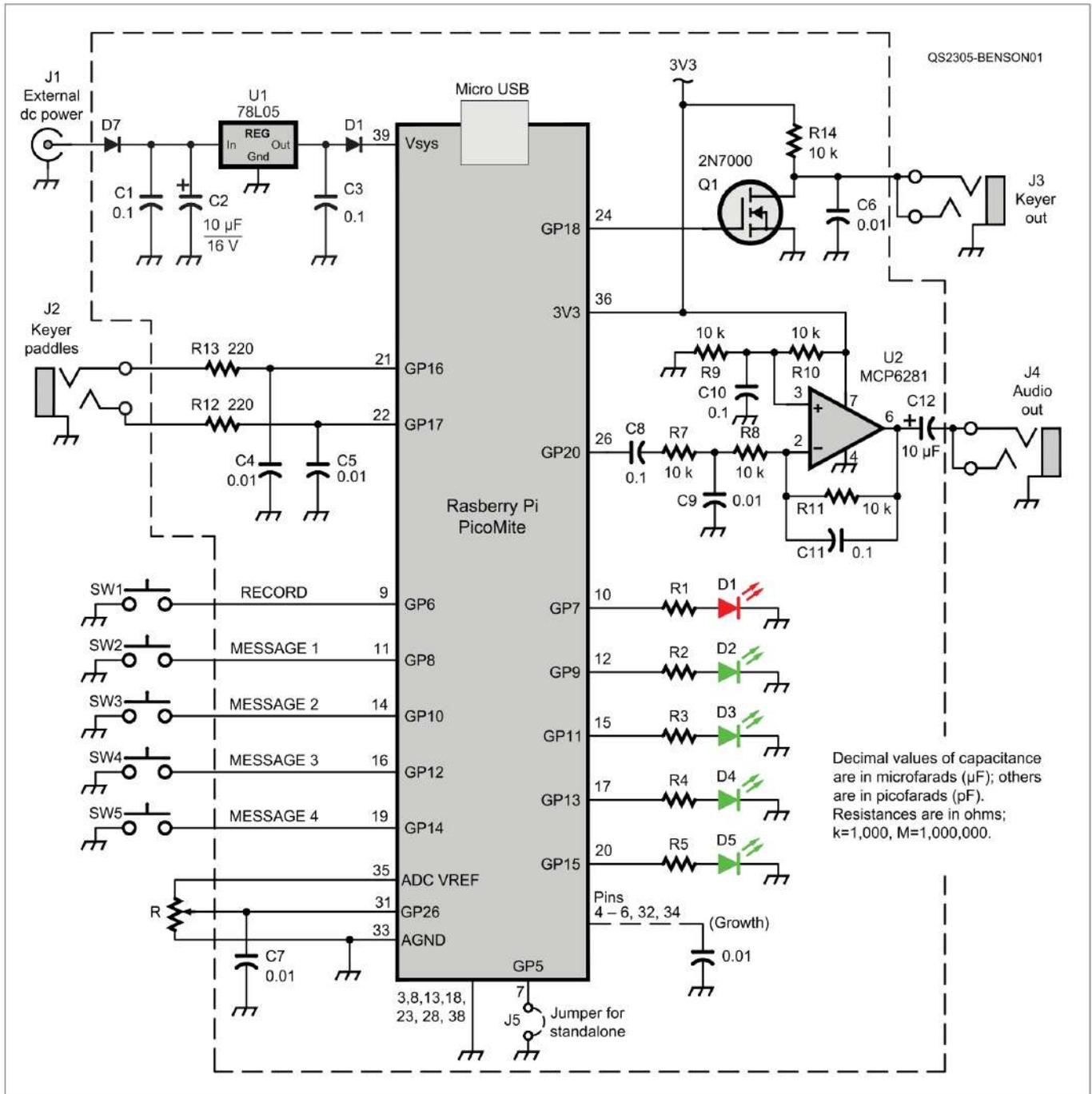
Figure 1 — Schematic diagram of the Pico Memory Keyer.
