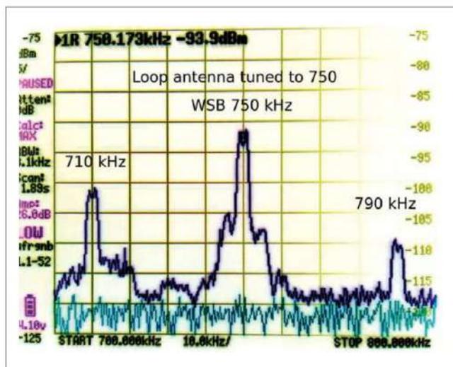
Figure 1 — The addition of a front-end filter made it possible to accurately measure AM broadcast signals.
