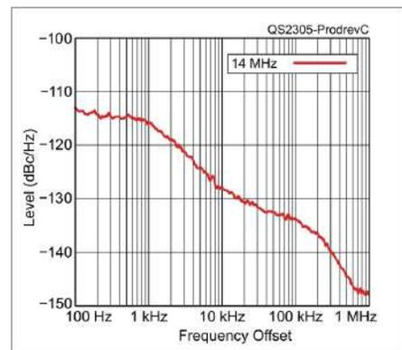
**Figure C** — The spectral display of the Xiegu G106 transmitter output during phase-noise testing. Power output is 5 W on the 14 MHz band. The carrier, off the left edge of the plot, is not shown. This plot shows phase noise 100 Hz to 1 MHz from the carrier. The reference level is -100 dBc/Hz, and the vertical scale is 10 dB per division.
