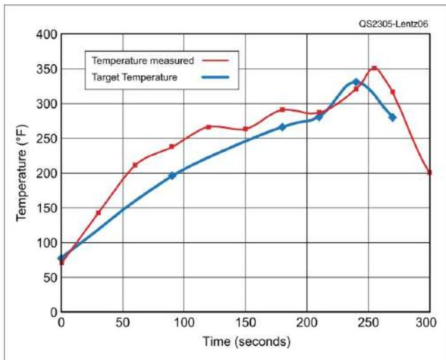
**Figure 6** — A graph of the Chip Quik TS391LT recommended soldering temperature profile (blue) versus the measured temperature profile (red). This depicts the PCB surface temperature, not the oven air temperature.
