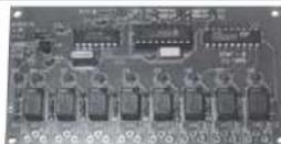
Remote control eight devices via radio audio. Password protection against unauthorized entry. Unique board ID. Comes assembled with relays. 4.5" x 2.5".
