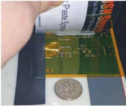
**Figure 2** — Applying solder paste through a stencil.
