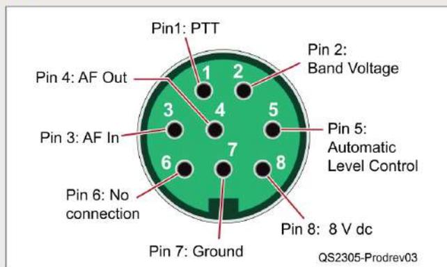
Figure 3 — Xiegu accessory port pinouts and descriptions.
