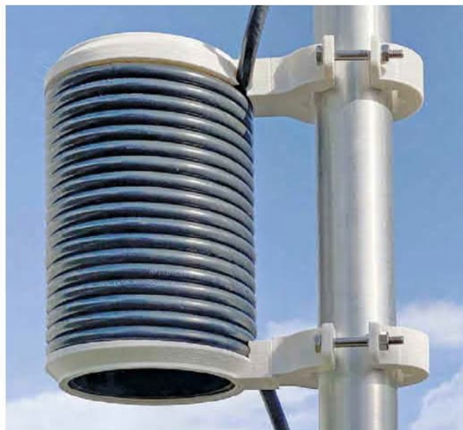
Pole-mounted 160-meter un-ugly balun.
