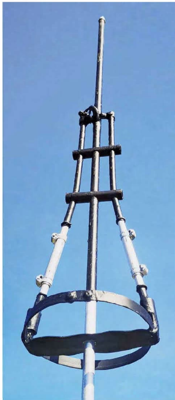
The Astroplane antenna modified for 2 meters.
