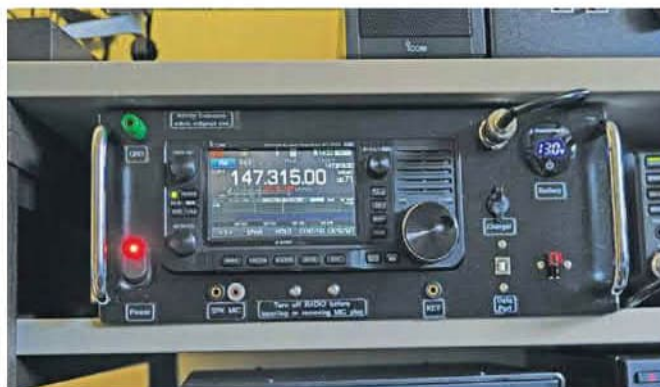
Figure 10 — The aluminum chassis out of the IC-705 Go-Bag, fitting perfectly on my shack shelf.
