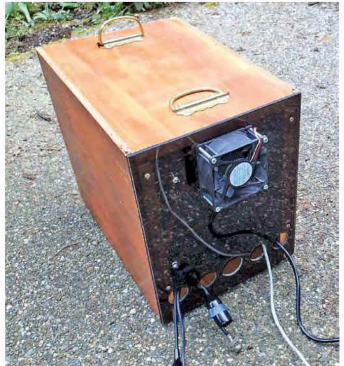
The completed station in a box with Plexiglas. Note the coax antenna plugs, ground wire, network, and power cables.
