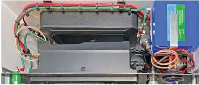
Figure 5 — The inside of the IC-705 Go-Bag with the AH-705 automatic antenna tuner.
