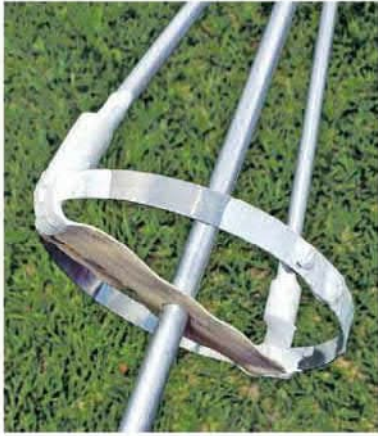
Figure 4 — A close-up of the loop attachment. The supporting strap across the bottom is PVC insulating material.
