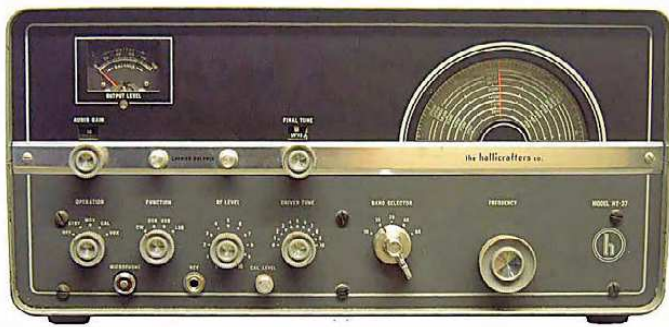
The HT-37 used the phasing method of sideband generation, while the HT-32 family used a crystal-lattice filter to generate SSB. [Photo courtesy of www.rigpix.com ]
