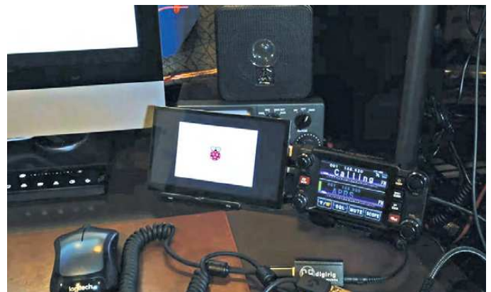
Darren, N4VFR, shows viewers the process of setting up an APRS digipeater and IGate.
