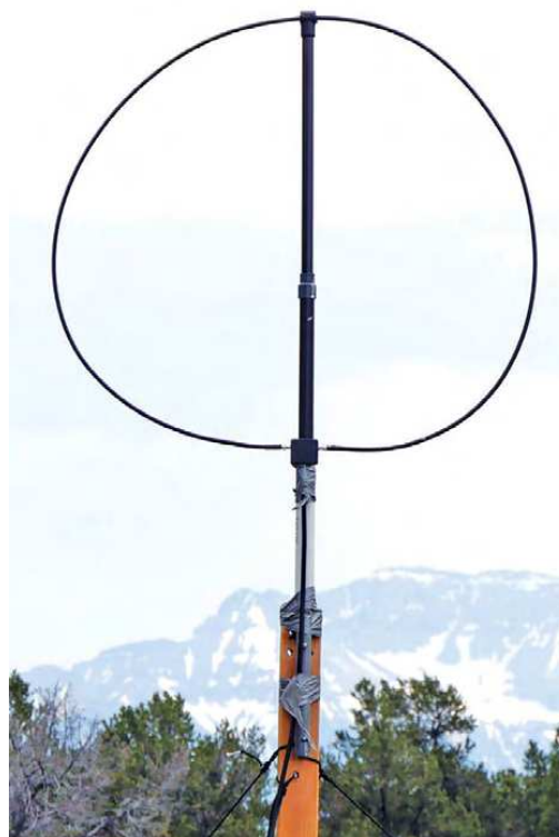
Figure 2 — Dave Casler’s, KE0OG, W6LVP receive-only antenna. The shield of the loop of coax is the actual antenna. The preamp box is located where the ends of the coax loop come together at the bottom. Twelve V dc is supplied via the antenna-to-receiver coax to the preamp via a bias T that comes with the antenna. Do not try to transmit through this antenna, as doing so will ruin the preamp.
