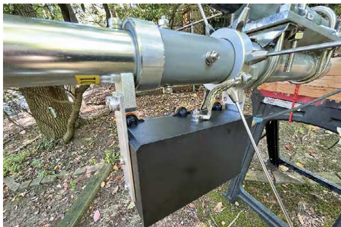
Figure 4 — The Xiegu VG4 base section with balun box.
