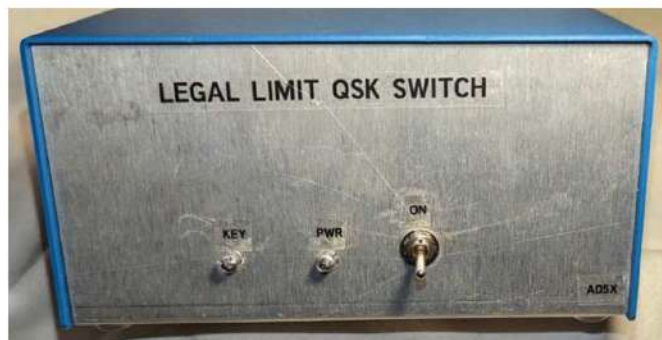
The author's new inexpensive relay-based QSK switch.
