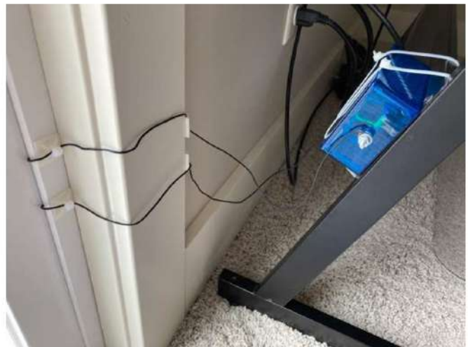
Figure 3 — The 49:1 balun is mounted in the blue box with the antenna lead also shown, and the ground connection and feed line are at the opposite end. The antenna and ground wires exit through the patio door and are secured via self-adhesive cable tie anchors. [Rich Barnett, N9NP, photo]
