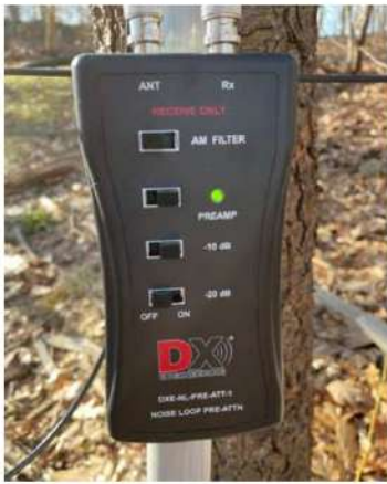
Figure 10 — DXE Portable Receive Preamp/Attenuator.
