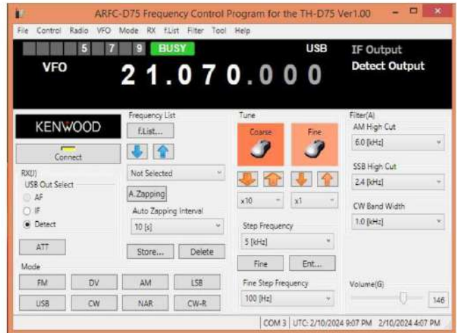
Figure 4 — The free Kenwood ARFC-D75 application allows remote control of the TH-D75A.
