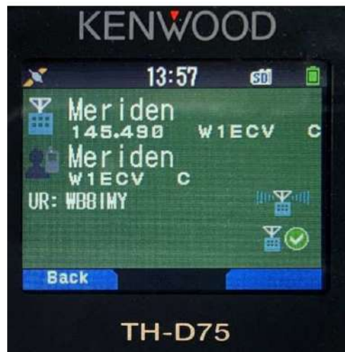
Figure 1 — Connecting to a nearby D-STAR repeater. Thanks to the TH-D75A's GPS and D-STAR repeater list, finding available repeaters takes only seconds.
