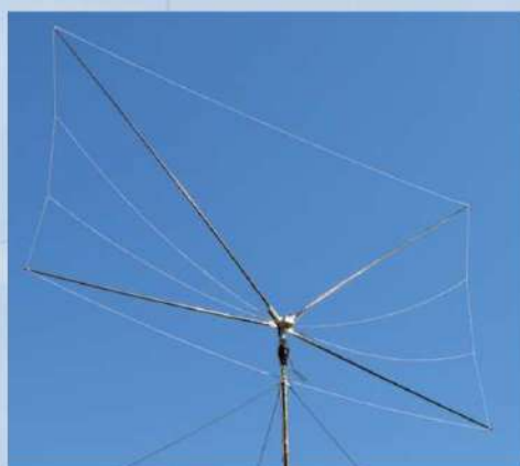
This page displays two past winners of the 2017 QST Antenna Design Competition, 80 through 10 meters category, both published in the March 2018 issue of QST. The photo to the left is "Cat Whiskers," The Broadband Multi-Loop Antenna," by Jacek Pawlowski, SP3L. The
