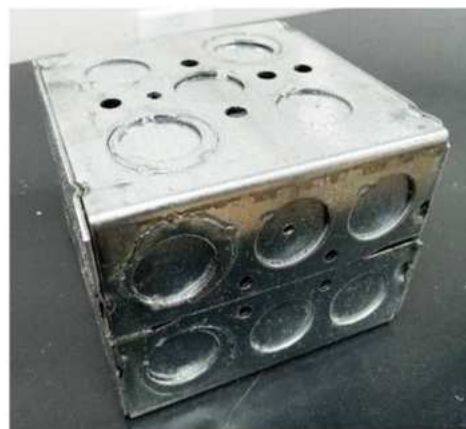
Figure 1 — The two steel electrical boxes mounted one on top of the other. [Robert J. Zavrel, W7SX, photo]
