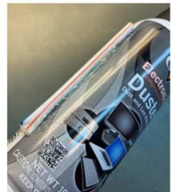
Figure 4 — Attach the drinking straw to the side of the can, with the closed end pointing down. [Dino Papas, KLØS, photo]
