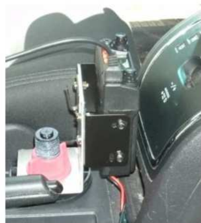
Figure 6 — The custom mount fits perfectly into the cup holder without causing damage. A piece of scrap aluminum was used to create a small platform for the radio. [John Dewey, KA9CAR, photo]
