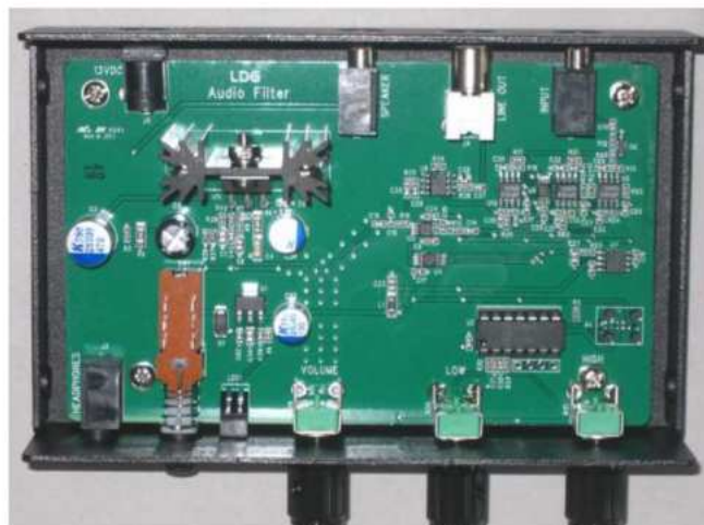
Figure 8 — The LDG AAF5 internal printed circuit board.
