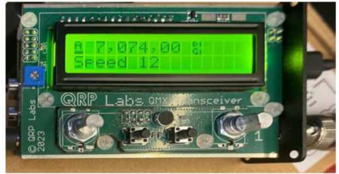
Figure 2 — The QMX with the display board installed.
