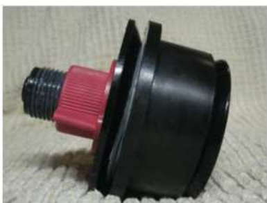
Figure 5 — A test plug is used to temporarily seal a pipe for testing under pressure. [John Dewey, KA9CAR, photo]
