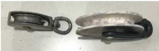
Figure 1 — On the left is a steel rope pulley; on the right is a plastic clothesline pulley. [Bruce Blackley, WD4LBR, photo]
