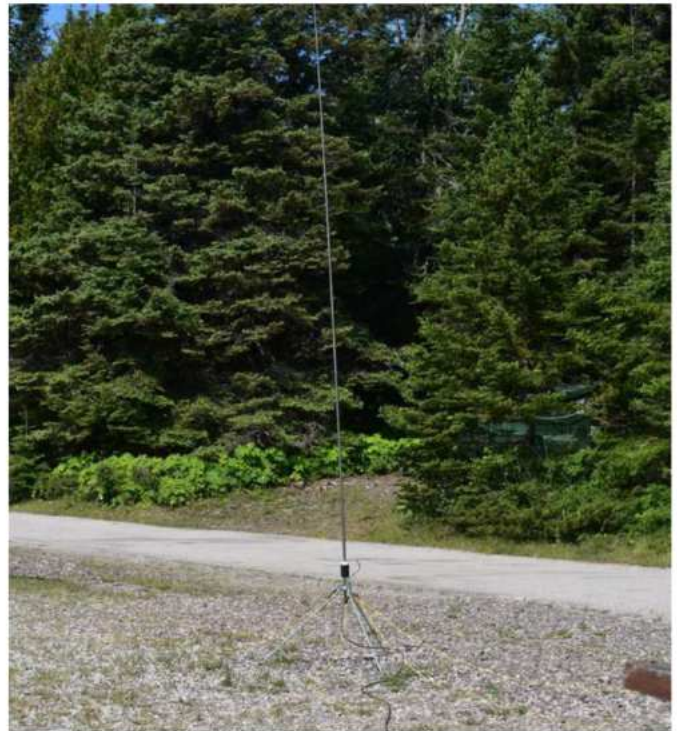
A Wolf River Coils Take It Along (TIA) antenna was used for operating. [Jon Oldenburg, AB9AH, photo]
