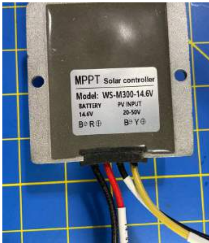
Figure 2 — My solar controller can manage a 24 V panel, providing a constant 14.6 V to the battery while the sun shines. It comes with solar panel connectors, but I changed mine to Anderson Powerpoles for maximum flexibility.
