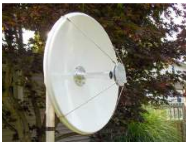
Figure 10 — The AH-109PB parabolic dish antenna available from Icom. This antenna would be a good choice for 10 GHz DX work.
