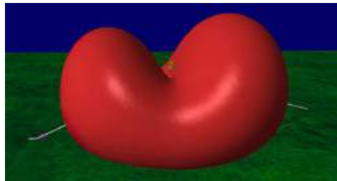
Figure 5 — The 3D pattern of an 80-meter EFHW operating on 40 meters, as generated in 4nec2.
