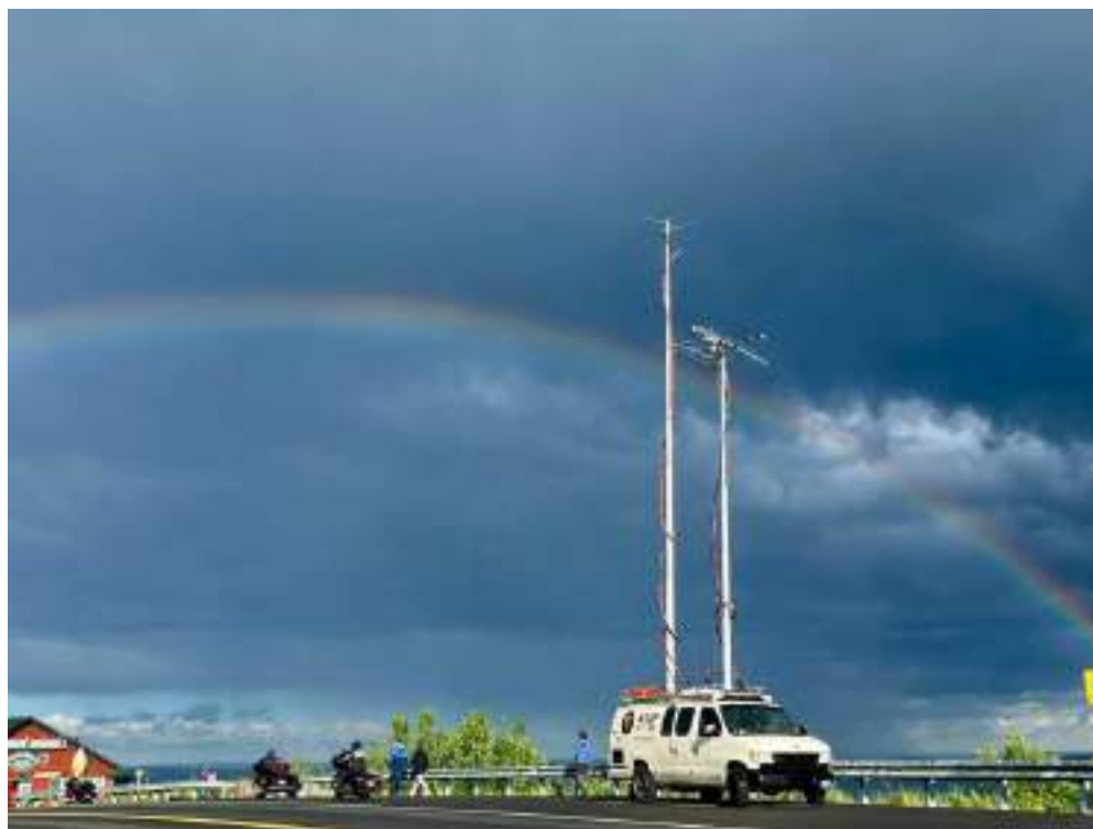
Chris Knox, K11P, operated from Hogback Mountain in southern Vermont during the 2024 ARRL June VHF Contest. His rover vehicle is a repurposed television news production van, which he outfitted as his mobile shack. [Christopher Knox, K11P, photo]
