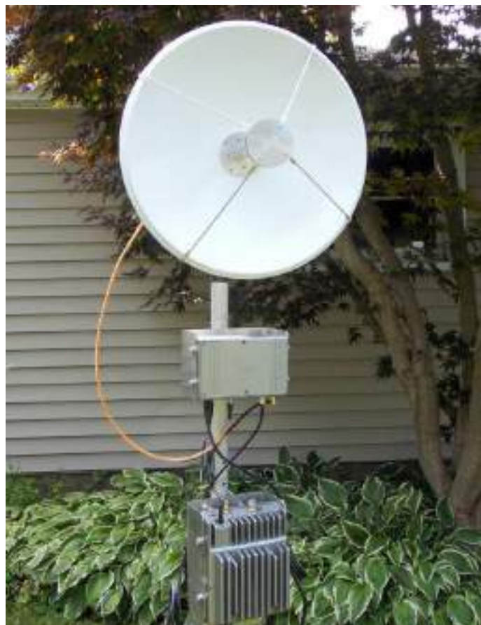
Figure 1 — The bottom unit is the RF for 2 meters and 70, 23, 13, and 6 centimeters. The upper unit is the 3-centimeter transverter. The antenna shown is the optional AH-109PB parabolic antenna for 10 GHz (Note: the tripod and mast are not included).
