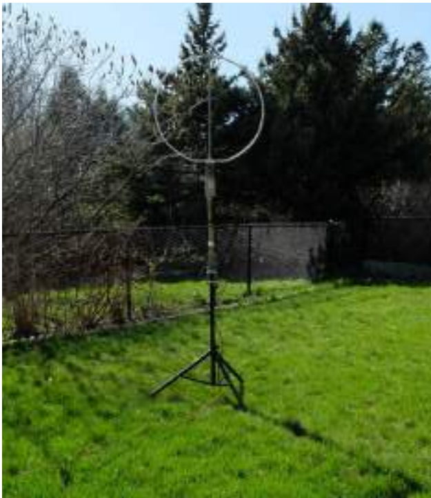
Figure 16 — The PWRC setup with a low-noise loop.
