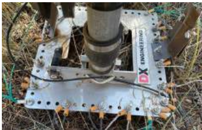
Figure 1 — A stainless steel radial plate at the base of my vertical antenna. Each connector is crimped and soldered. Each radial terminates at the radial plate. The coax outer conductor is attached to the radial plate. A ground rod is connected, too. Note that you should use an anti-seize compound when installing the stainless steel nuts and bolts so the bolts will not shear off when they are removed.
