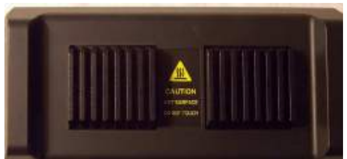
Figure 5 — The IC-905 main-unit rear-panel heatsink.
