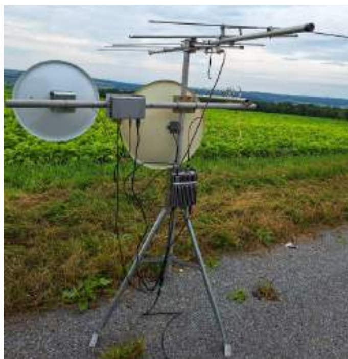
Figure 11 — The system set up for six-band operations in FN02, showing the short RF cables needed between the antennas and radio. The dual-band Yagi, short loop Yagi, and dish in the center of the tripod are not supplied by Icom. The setup of the equipment was simple and took no more than a few minutes to be fully operational.
