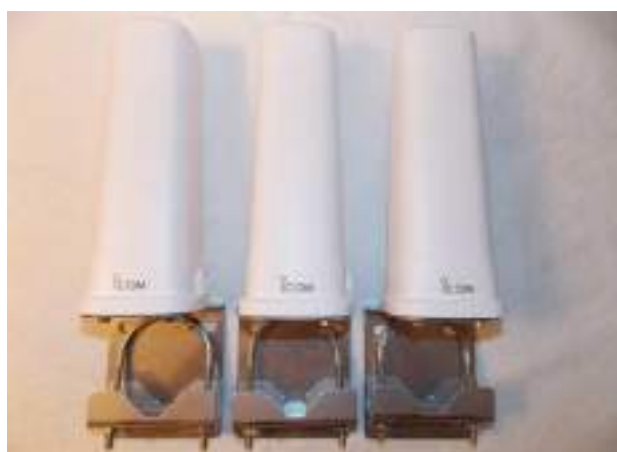
Figure 9 — The three omnidirectional antennas offered by Icom for 2.4, 5.6, and 10 GHz (Note: these are low-gain antennas and are vertically polarized).
