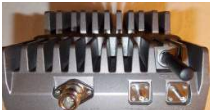
Figure 6 — Connections to the included RF module. Left to right: N-female for 2 meters, 70 centimeters, and 23 centimeters; SMA female for 13 centimeters, and SMA female for 6 centimeters. Also shown is the GPS antenna.
