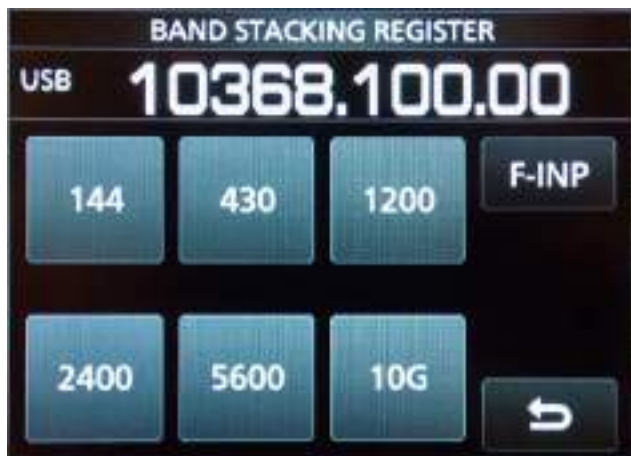
Figure 8 — Band stacking register (“bandswitch”). You can also manually enter a frequency in the radio’s operating range using the F-INP button.
