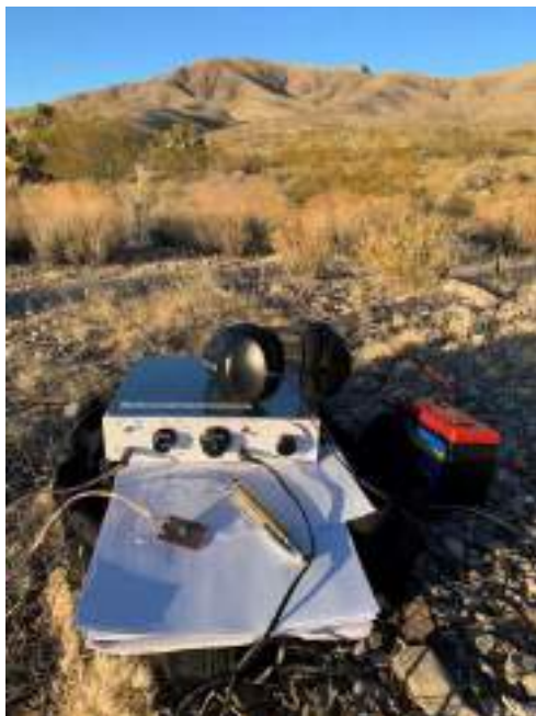
James Kretzschmar, AE7AX, participated in the 2024 ARRL Straight Key Night using his homebrew 40-meter CW transceiver while portable at the Beaver Dam Wash National Conservation Area in Utah. He completed three contacts running 2 W into a temporary inverted-v antenna. [James Kretzschmar, AE7AX, photo]
