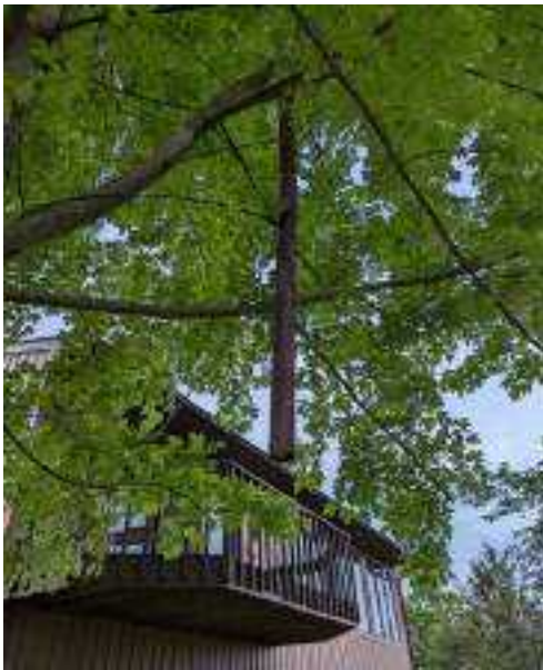
Figure 4 — The antenna in place, with a coat of camouflage paint. To a casual observer, it looks like it is part of the tree. [Tom Inman, KC8T, photo]
