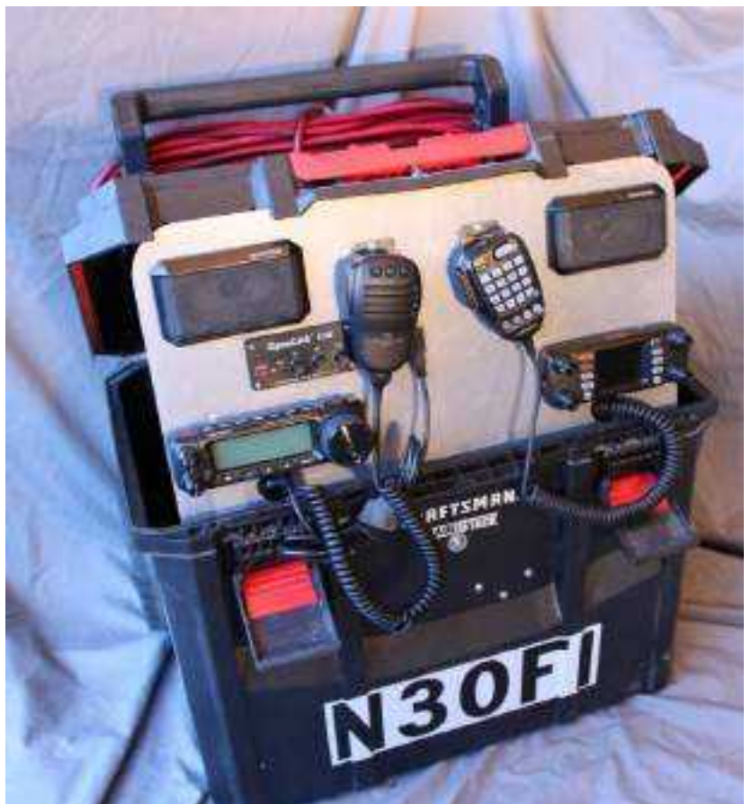
The radio go-box with the aluminum plate in the inverted position.
