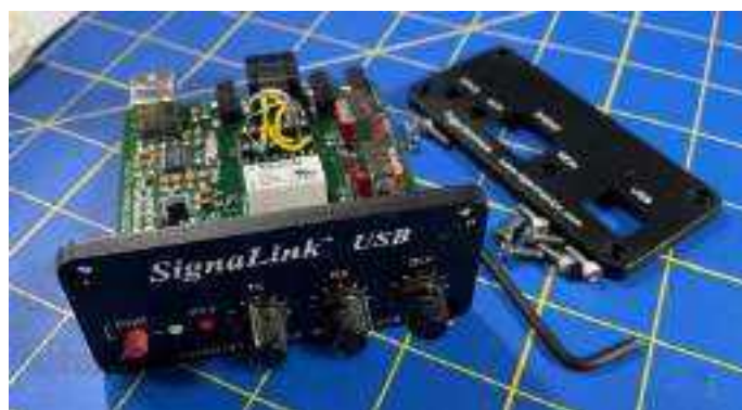
Figure 2 — The Signalink USB showing the jumpers inside. The jumpers get ground, transmit, and receive audio to the right pins on the cable connected to the radio. Nowadays, most HF radios contain a built-in sound card, so a separate sound card interface is not required.
