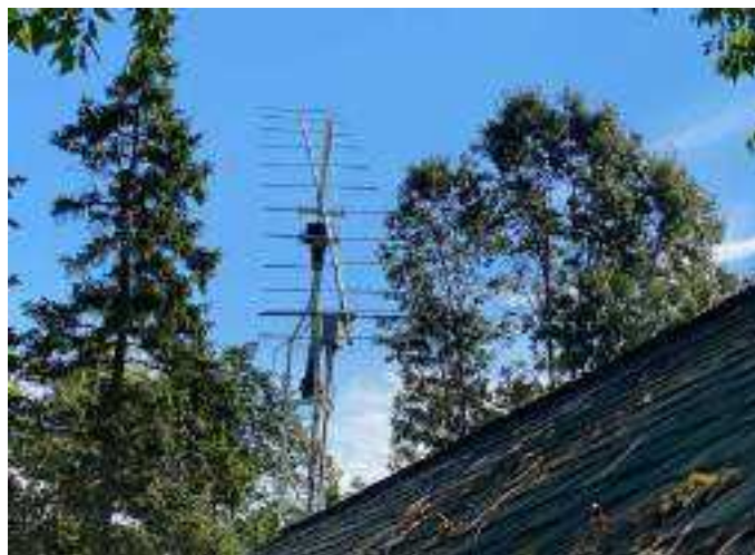
Jim Kennard's, W2EKE, homebrew 13-element Yagi. He used this antenna to make his first 2-meter Earth-moon-Earth contact on September 20, 2024. [Jim Kennard, W2EKE, photo]
