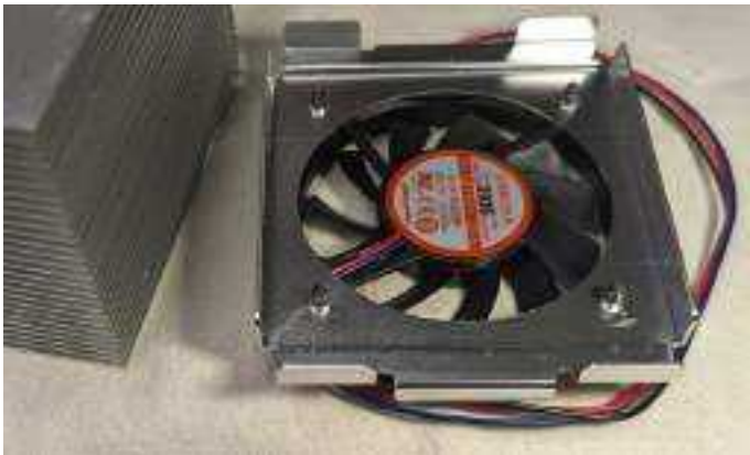
Figure 1 — The fan mounted with sheet metal screws.
