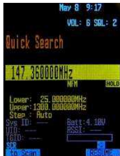
Figure 4 — The Quick Search function allows you to directly enter a frequency of interest.
