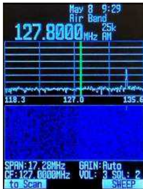
Figure 5 — The optional SDS100 waterfall display shown sweeping through the aviation band.
