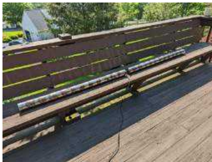
Figure 3 — I made my initial tests with the antenna too close to the house and other objects. As a result, I thought the dipole was too long, and I shortened it accordingly. That was a big mistake, but a valuable learning experience. [Tom Inman, KC8T, photo]
