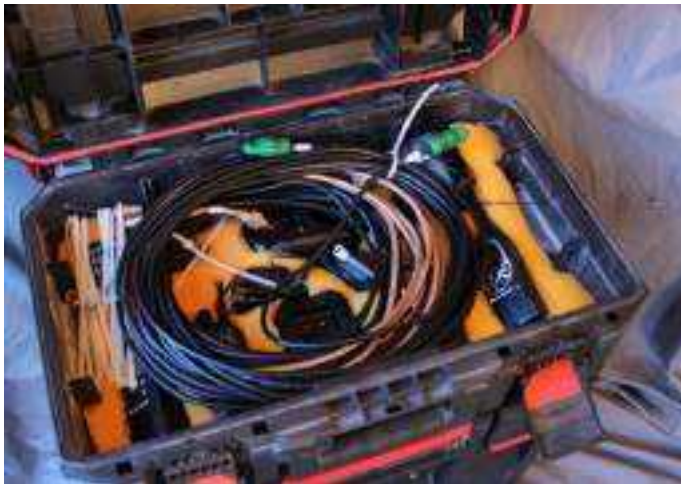
The radio go-box with cutouts in the foam padding to easily store handheld radios and their accessories while maintaining organization.
