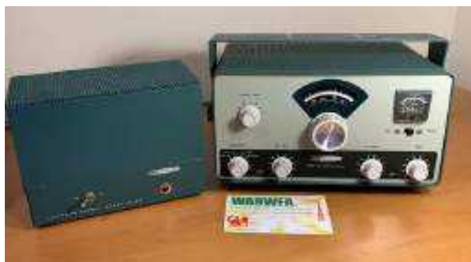
The HW-12 75-meter SSB station and HP-23 power supply built by re-kitting.
