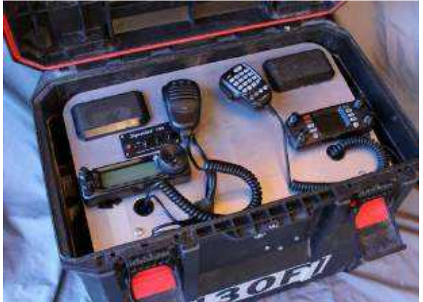
The radio go-box with the aluminum plate in the flat position.
