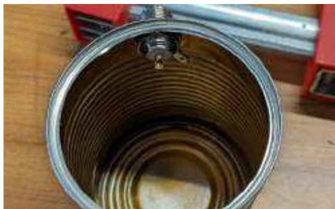
Figure 2 — Installing the SO-239. [Tom Inman, KC8T, photo]
