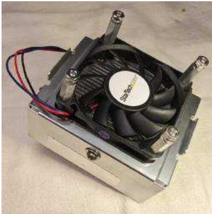
Figure 2 — The standoffs and fan attached to the heatsink.
