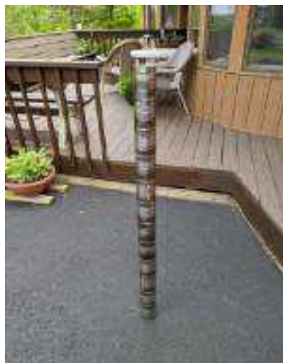
Figure 1 — One leg of the soup can vertical dipole, soldered and ready for use. [Tom Inman, KC8T, photo]
