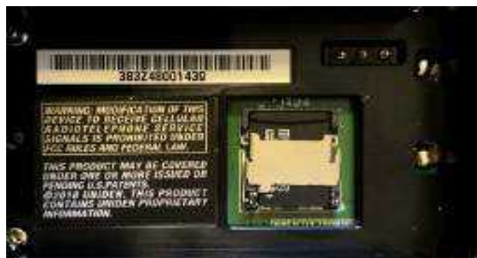
Figure 1 — The SDS100 memory card can be found inside the radio, directly beneath the battery. An 8 GB card is supplied, but you can install a larger card, up to 32 GB.
