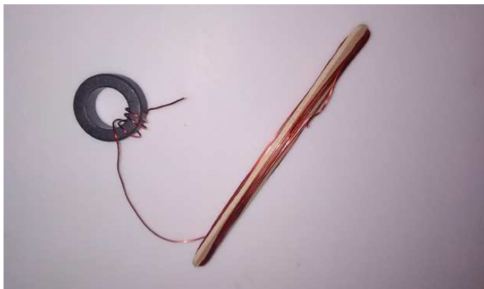
Figure 5 — When making lots of turns with a very fine wire, a shuttle can make it easier to pass the wire through the toroid without tangling the wire.
