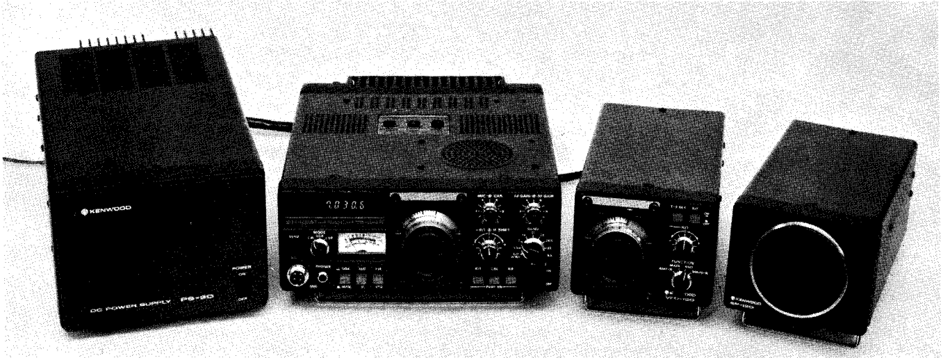
The Kenwood TS-120S ssb/cw five-band transceiver is shown here with the matching PS-30 power supply, VFO-120 remote VFO and SP-120 external speaker. The combination makes a compact, flexible station whether mobile, portable or fixed.
