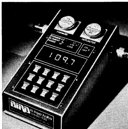
Fig. 6 — The Bird Model 4381 RF Power Analyst. A collapsible bail permits positioning the unit for easy readability.
