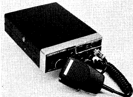
Fig. 4 — An easy way to 10-meter fm. The Comtronix FM80 presents a simple but functional control panel.
