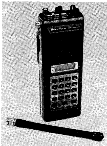
Fig. 7 — The Kenwood TR-2400 2-meter fm transceiver. The BNC antenna connector is a thoughtful feature.
